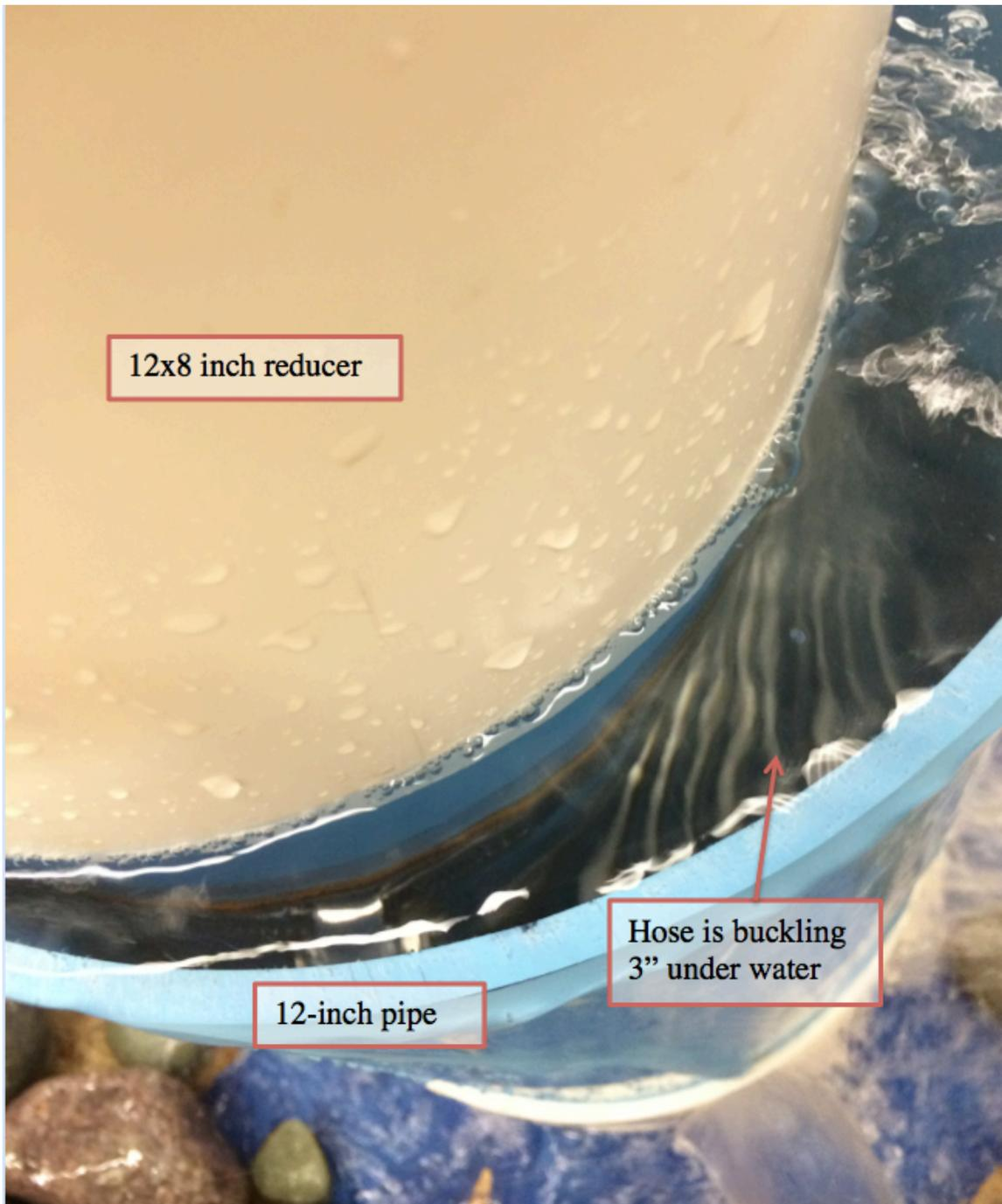
**Figure 4-12** Hose is buckling with the water counter pressure approach used.
