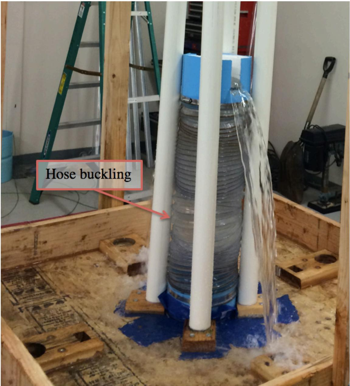
**Figure 4-14** Hose is buckling and leaning toward the supporting pipes.
