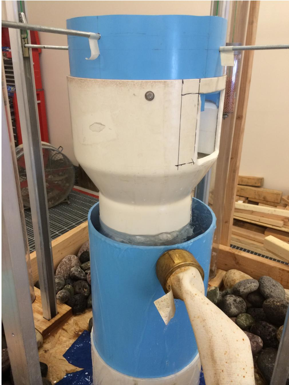
**Figure 4-11** water outside the hose is used to counter the water pressure inside the hose
