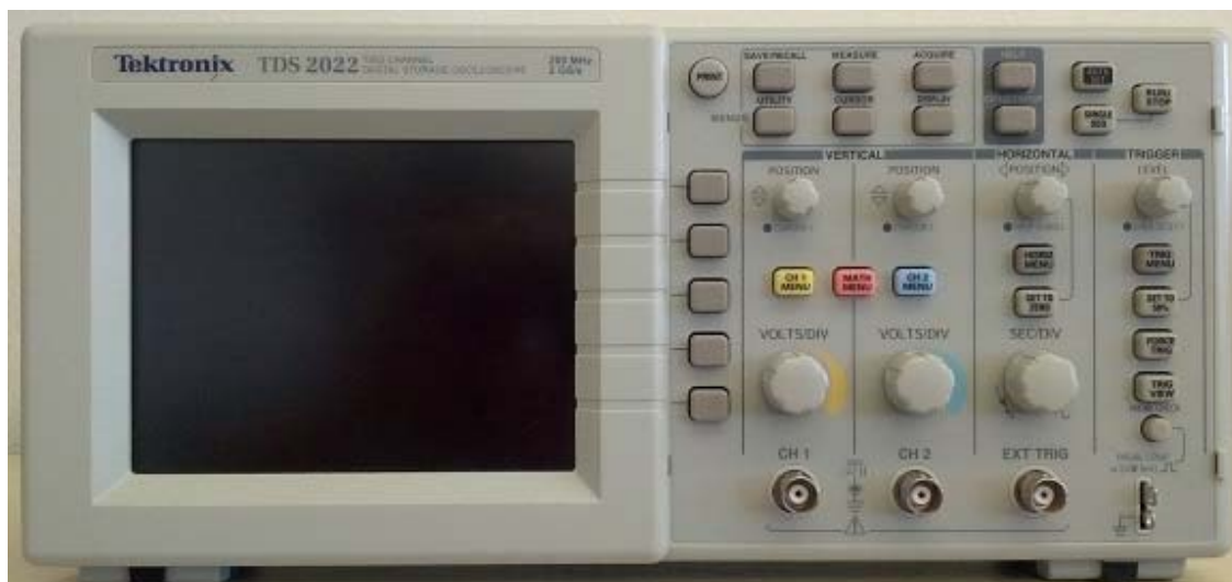
Figure 6. Oscilloscope used for graphically representing voltages.
