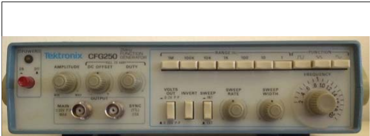
Figure 12(a). Traditional bench-top function generator.
