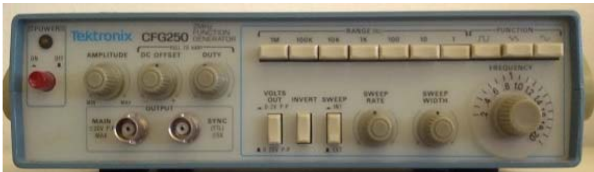
Figure 5. Function generator used for producing AC voltages.
