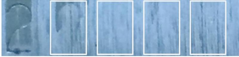
Figure 4.8: Stainless steel sample with numbers defaced (boxes show areas extracted and individually analyzed for each number).
