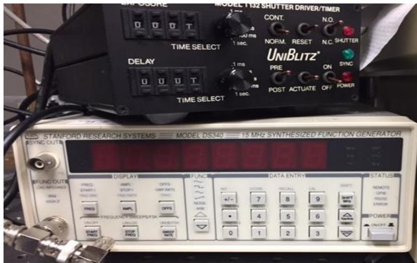
Figure A7: Mechanical shutter control box (top) and Stanford Research Systems function generator (bottom).
