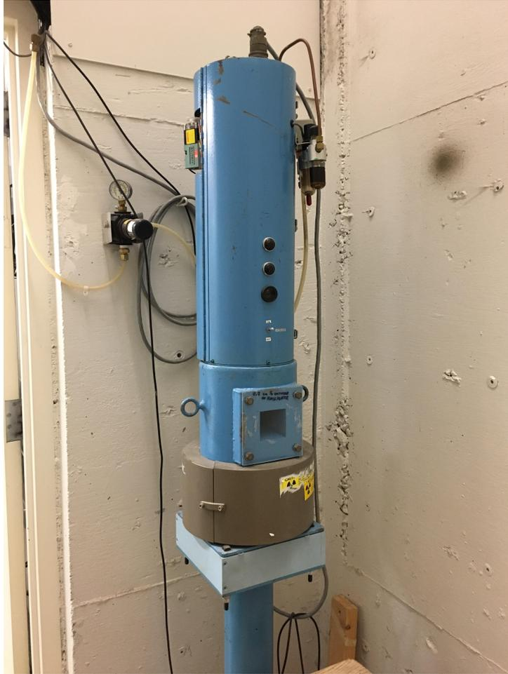
Figure 3.1: Containment unit for the Cs-137 source.
