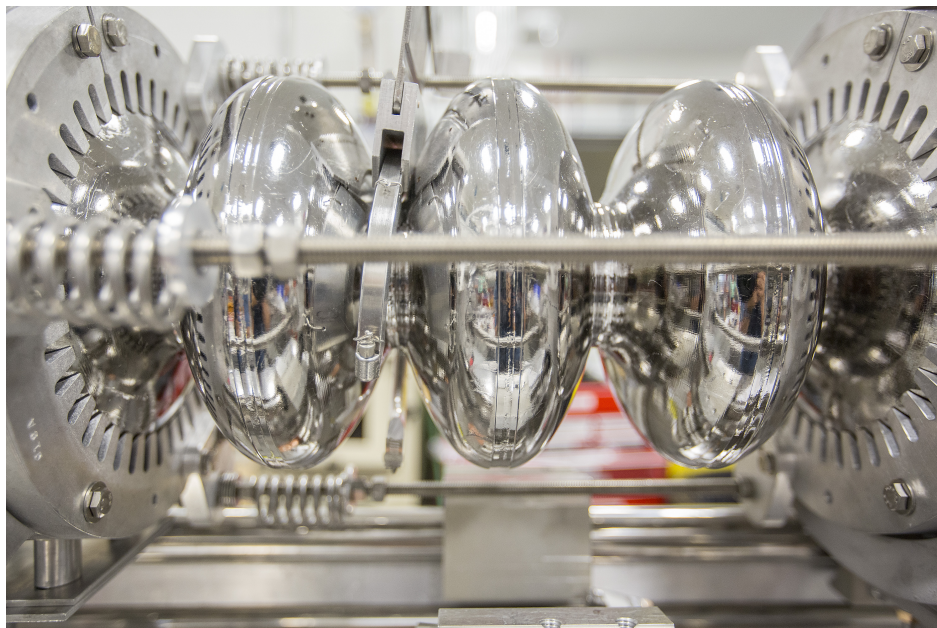
Figure 3.3. Photo of a Niobium Cavity.
