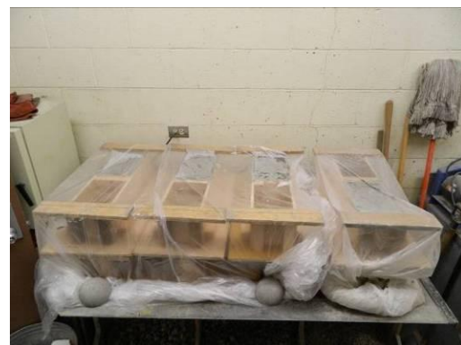
Concrete curing after pouring (allowed to cure for 24 hours).
