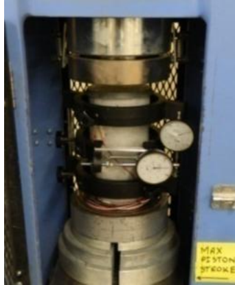
Figure 3.22 Compressometer/Extensometer Test Set-Up
