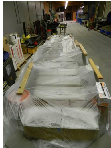
Covered with plastic for the first 24 hours.
