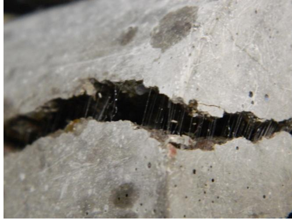
Figure 5.3 Split Tensile Crack
