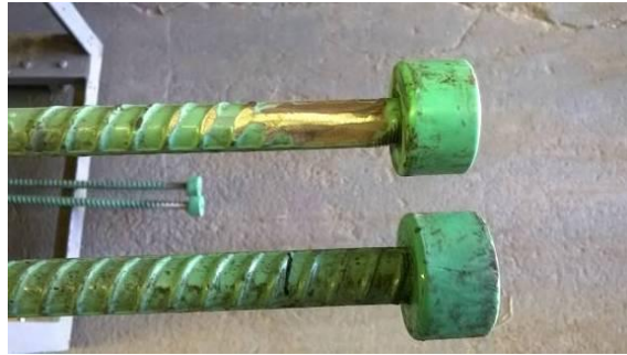
Headed rebar before (bottom) and after (top) grinding.
