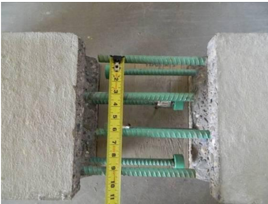
Rebars spaced 3 in. on center.
