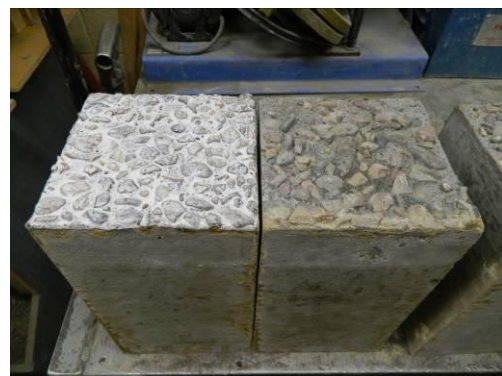
Sample applied with bonding agent (left) and without (right).
