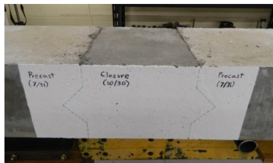
Figure 5.23 Beam Specimen Painted and Interface Lines Drawn
