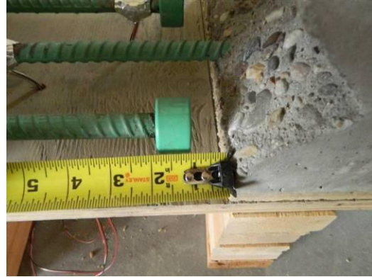
Headed rebars located 1 in. from the interface.
