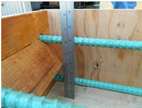
Showing rebars placed 2 in. and 6 in. from the bottom of the mold.
