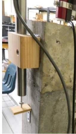
Figure 4.14 LVDT Set-Up for Headed Bar Pullout Tests
