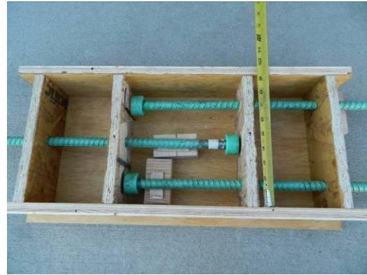
HB pullout mold showing width of 9 inches.
