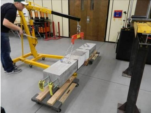
Lifting beam with shop crane.
