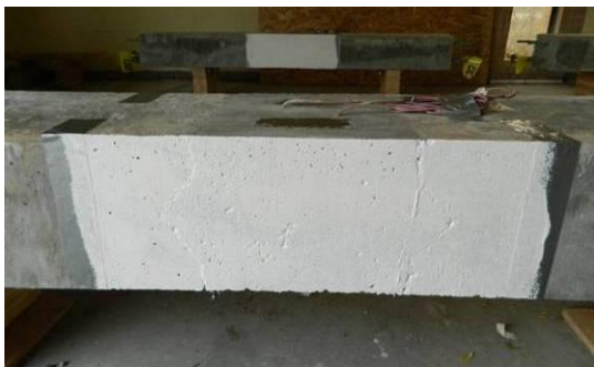
Side of beam painted white (Only center portion).
