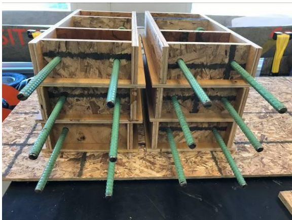
All six HB pullout molds.
