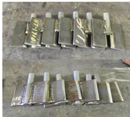
End fixtures made from 1 in. threaded rod and steel plate.
