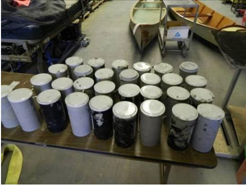
Over 30 cylinders poured (4 in. by 8 in.).
