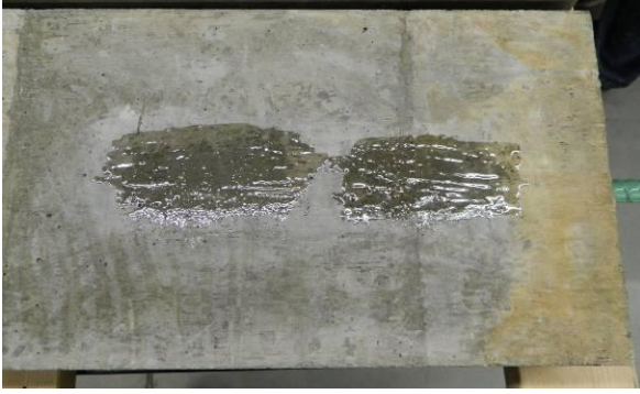
Base coat after curing 24 hours.
