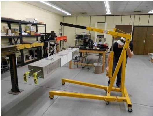
Lifting beam with shop crane.
