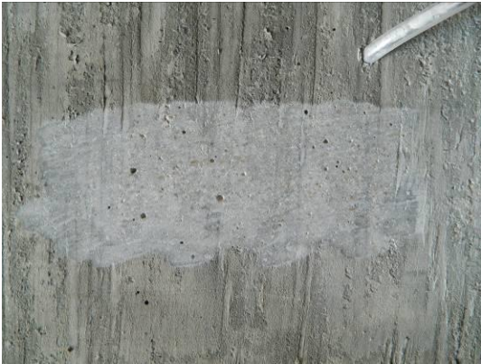
Gage area after grinding with a few small voids.
