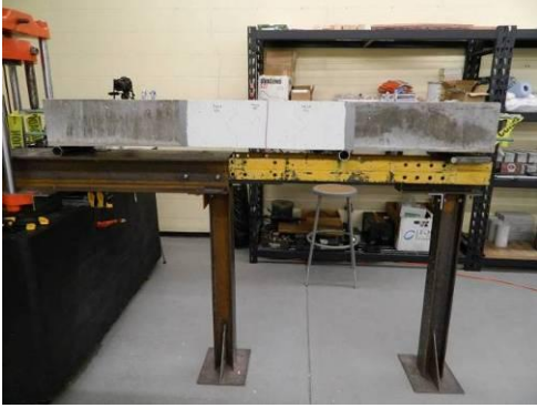
Concrete beam before setting in Tinius Olsen.
