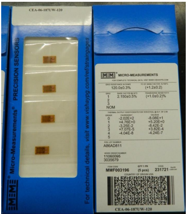
Figure L.1 Quarter Inch Strain Gage Specifications
