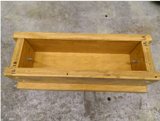
Wood mold. A wood sealer was applied to protect the mold over multiple uses.
