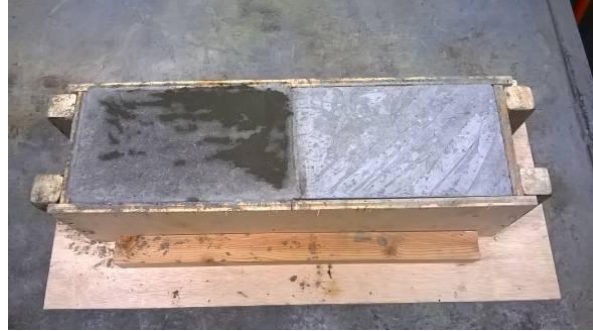
Closure concrete poured.
