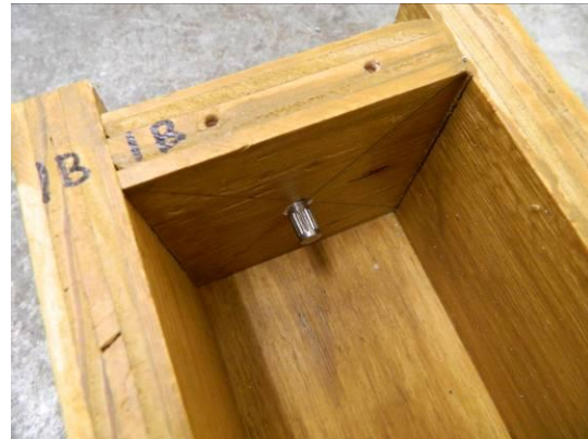
Gage stud screwed into end of mold.
