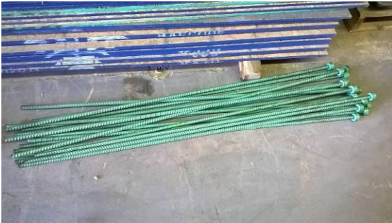
Rebars with Lenton Terminators (Headed rebars).
