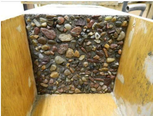
SSD substrate moisture condition applied to specimen without bonding agent.
