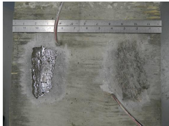
Before grinding/sanding epoxy base coat (left) and after (right).
