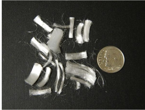
Figure 3.1 Polypropylene Fibers (Fibermesh 150)
