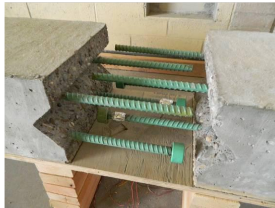
View of closure pour connection.
