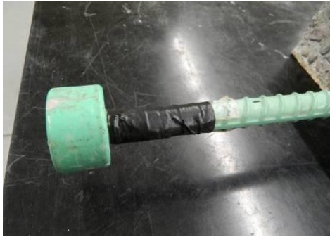
Strain gages wrapped with tape for protection during curing.
