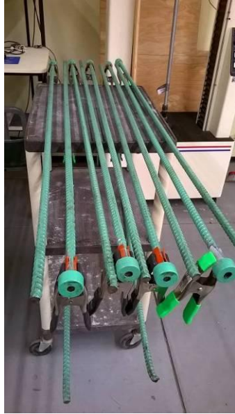
After strain gages were applied they were set out to cure.
