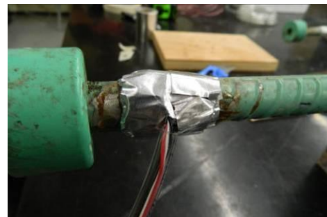
M-Coat F gage protection.
