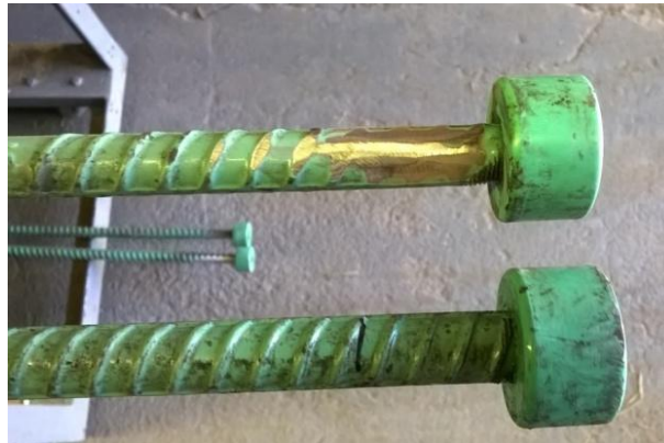
Figure L.4 Rebar Before (Bottom) and After (Top) Grinding
