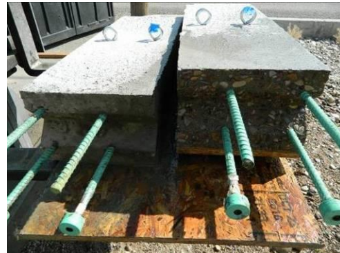
LB precast before and after washing.
