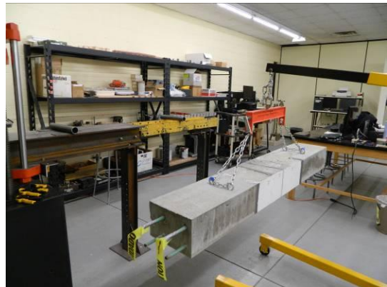
Lifting beam with shop crane.
