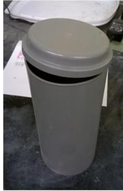
(a) Cylinder mold
