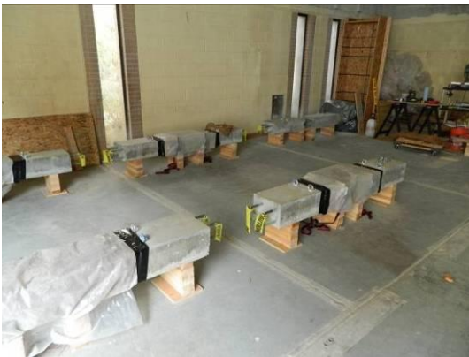
LB specimens curing.
