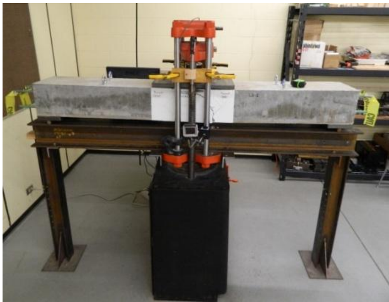
Figure 5.21 Typical Three-Point Flexural Beam Test
