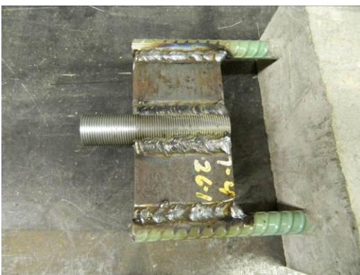
Threaded bar and steel plates welded to bottom rebars.
