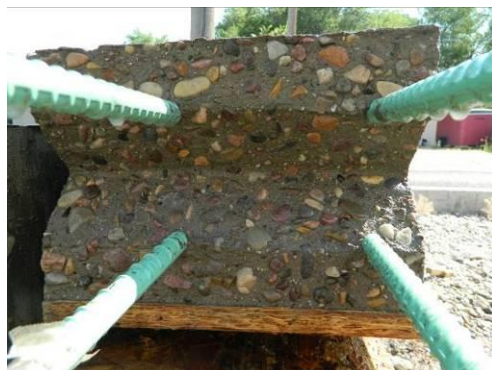
LB precast after washing, showing EA finish.
