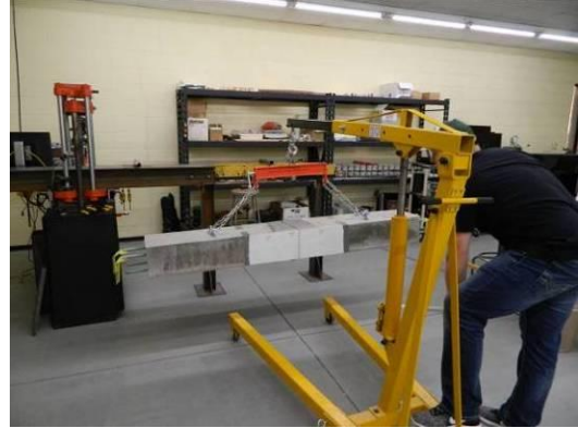
Lifting beam with shop crane.
