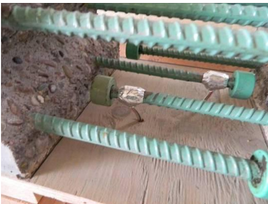
Strain gage wires and protective tubing set through the formwork.
