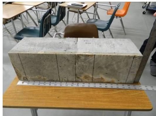
Interface beam marked and ready to be testing.
