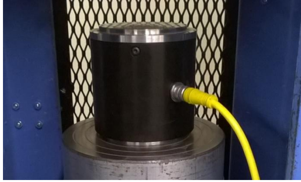
Figure 4.10 CLC-300K Load Cell
