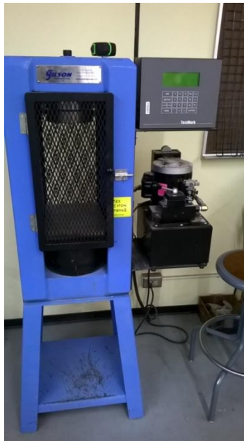
Figure 3.16 Gilson Compression Machine
