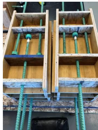
Inside dividers painted with Formula F concrete surface retarder.
