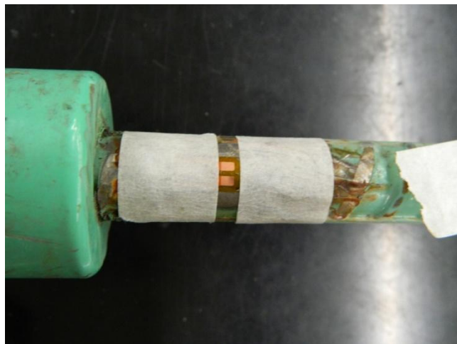
Figure L.7 Masking Tape Wrapped Around SG
