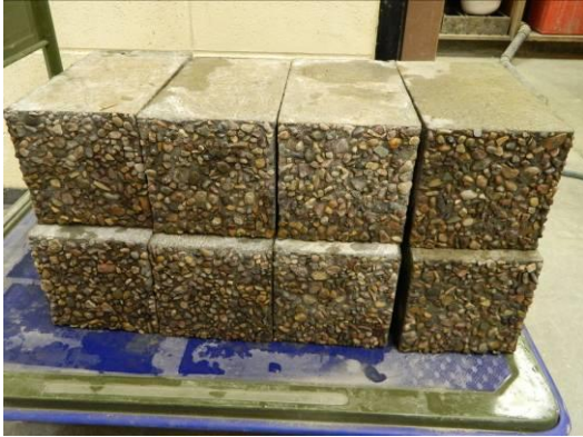
After washing away unhardened concrete produced from concrete retarder.
