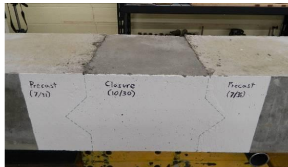
Interface between precast and closure concrete traced with a green marker.
