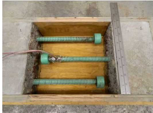
HB specimen before pouring closure concrete.
