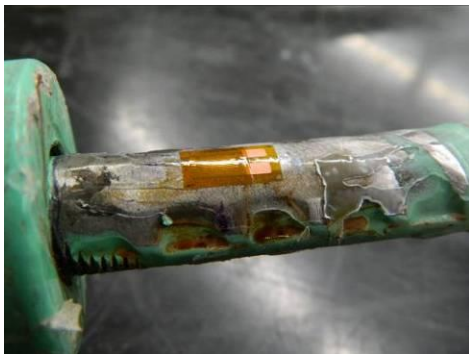
Bonded strain gage.
