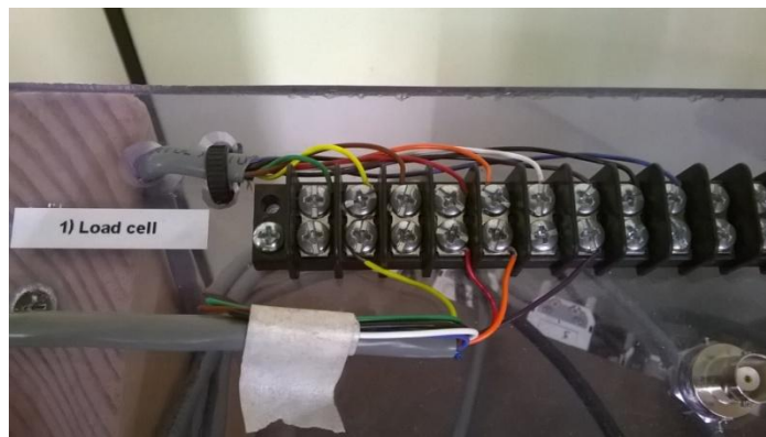
Figure L.22 CLC Wiring to Scanner
