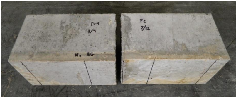
Figure 5.8 Interface Bond Test Sample –D-4 without Bonding Agent
