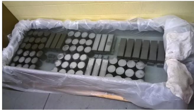
Figure 3.5 Water Tank for Moist Curing of Samples
