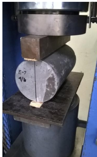
Figure 3.18 Splitting Tensile Testing Set-Up
