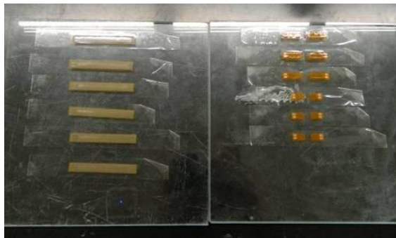
Strain gages ready for placement.
