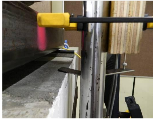
(b) LVDT extension bracket
