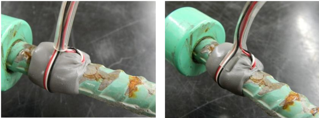
Figure L.15 Pressing Vinyl Tube into Rubber
