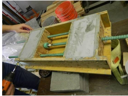
Removing HB precast portions from molds.
