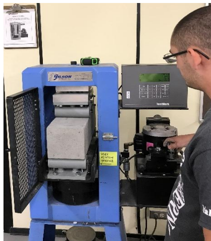
Figure 3.23 Interface Bond Test Set-Up
