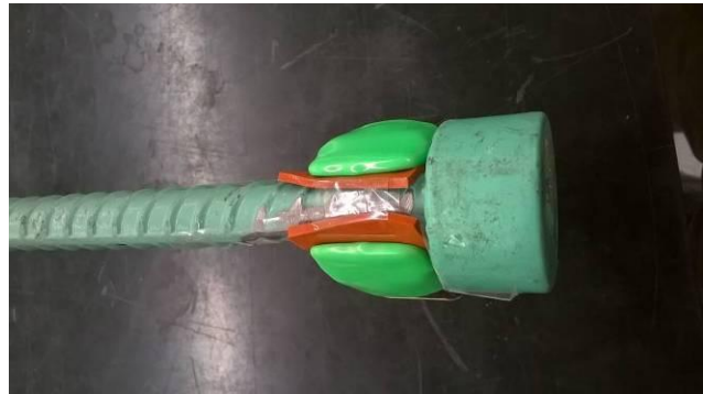
Silicon pads and a spring clamp applying pressure over gage area.
