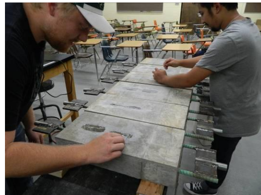
Applying base coat of M-Bond AE-10 to gage areas.
