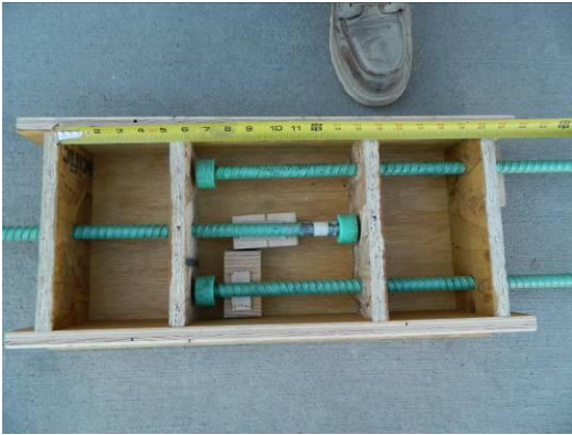
Headed bar pullout mold showing an overall length of 20 inches.
