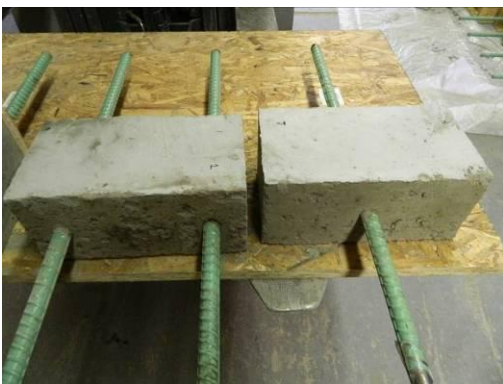
Precast interface before washing.
