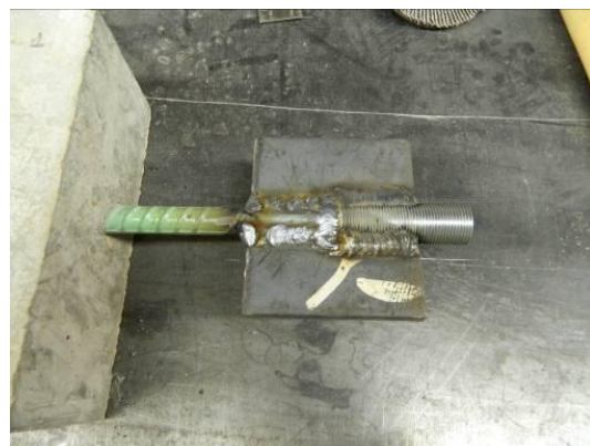
Threaded bar and steel plates welded to top rebar.
