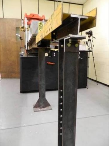
Extension beam (yellow) used for inserting and removing concrete beams.
