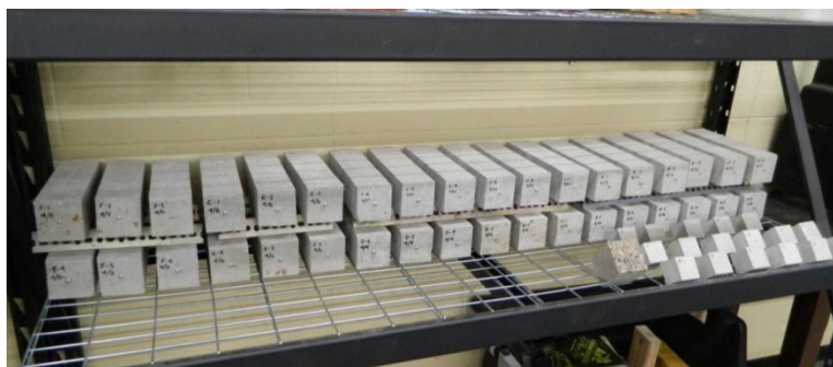
Figure 3.19 Shrinkage Specimens Air Drying
