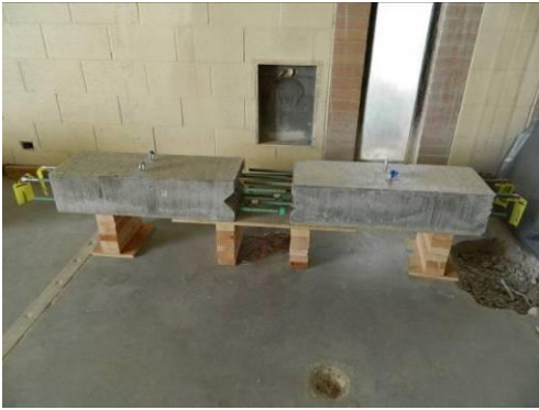
Setup for pouring closure concrete between the two precast beams.
