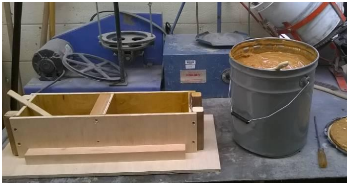
Concrete surface retarder (Formula F) being applied to inside of mold.
