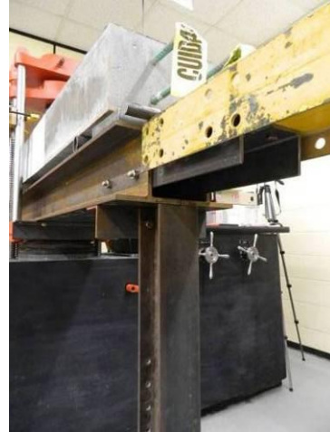
Extension beam connected to steel beams.
