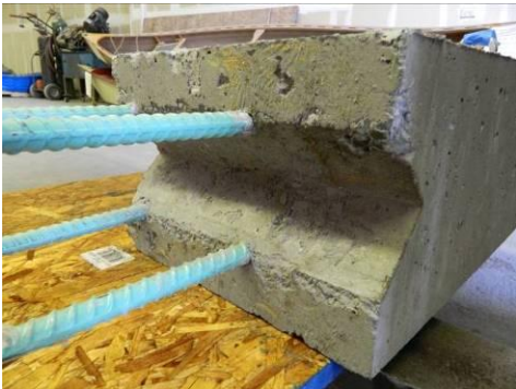
Unwashed precast interface.
