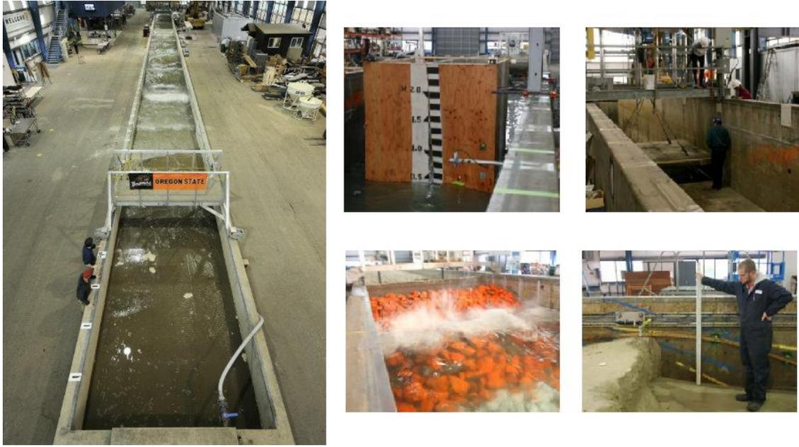
Figure 5: Large wave flume at Oregon State University
