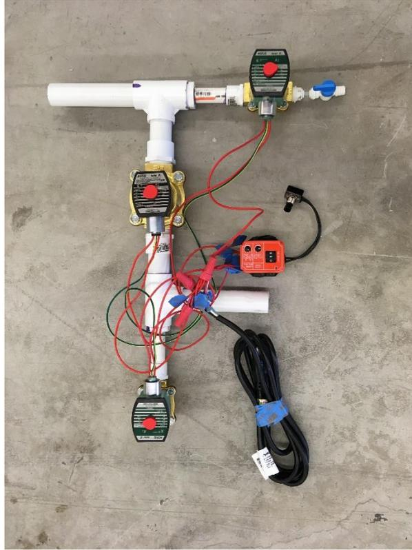
Figure 21: Solenoid valves arrangement
