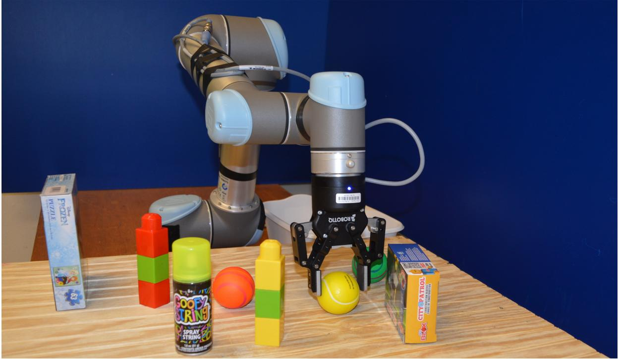
Figure 6.4.2: UR5 robot and Robotiq 2-finger gripper in the table clearing scenerio
