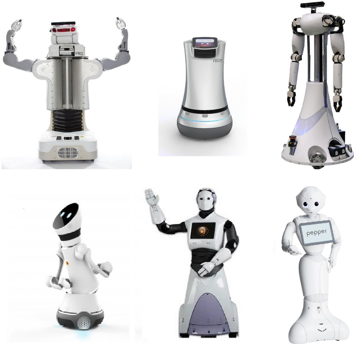
Figure 1.0.1: Several service robots present today: From left to right, top to bottom, a) PR2 by Willow Garage, b) Relay from Saviaoke, c) Amigo robot of Eindhoven University of Technology, d) Care-O-Bot 4 by Fraunhofer, e) Reem robot from PAL robotics, f) Pepper from SoftBank Robotics.
