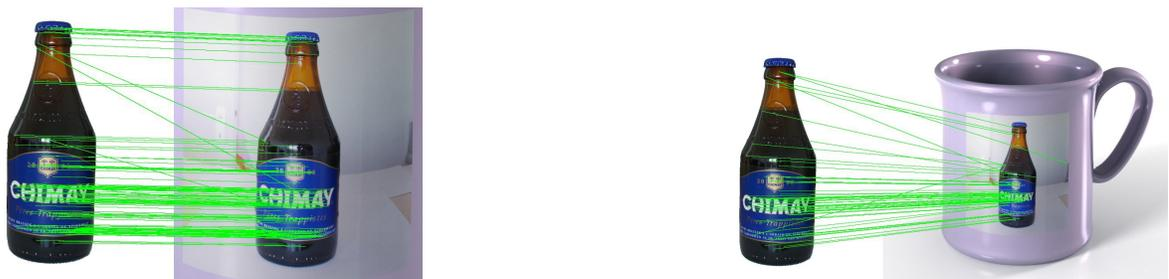
Figure 2.3.2: An example of a good model match using features extracted from 2D images (left), where a beer bottle template is successfully identified in an image. However, zooming out from the image, we observe that the bottle of beer is in fact another picture stitched to a completely different 3D object (in this case a mug). The semantics of the objects in this case are thus completely wrong (image from <https://pointclouds.org/>).
