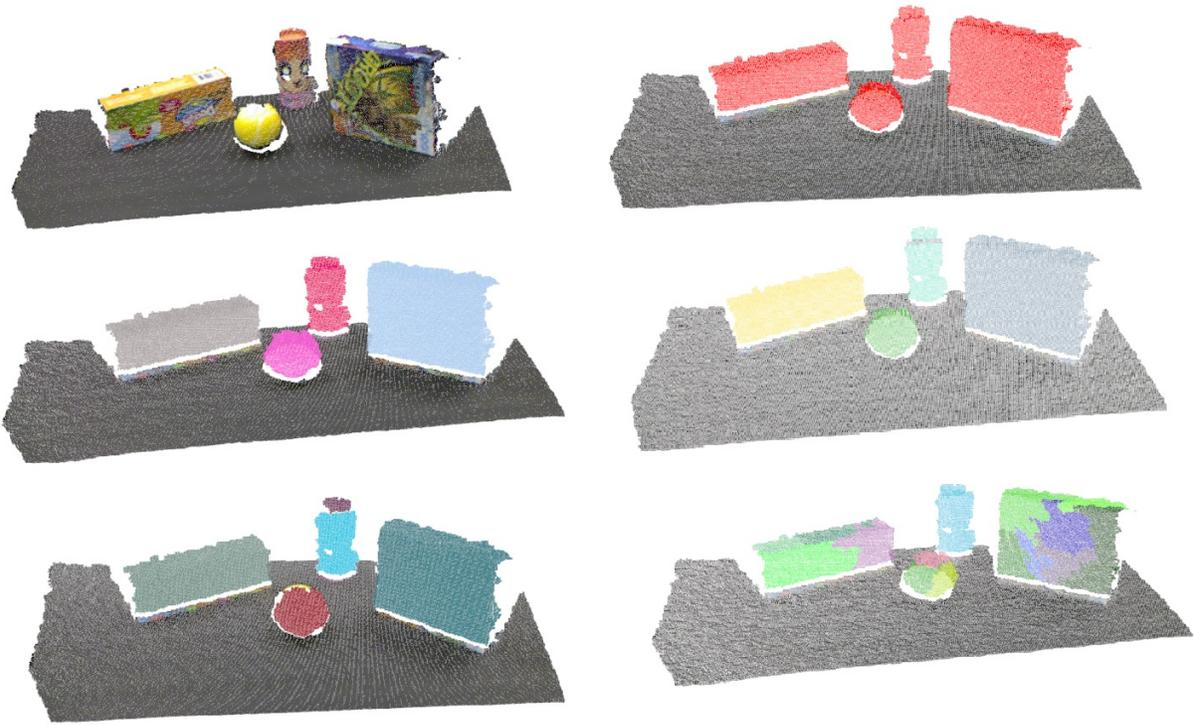
Figure 2.6.2: Different object clustering techniques. From left to right, up to down, a) Original captured image, b) Min-Cut segmentation, c) Euclidean clustering, d) Condition euclidean clustering, e) Region growing segmentation, f) Color based segmentation
