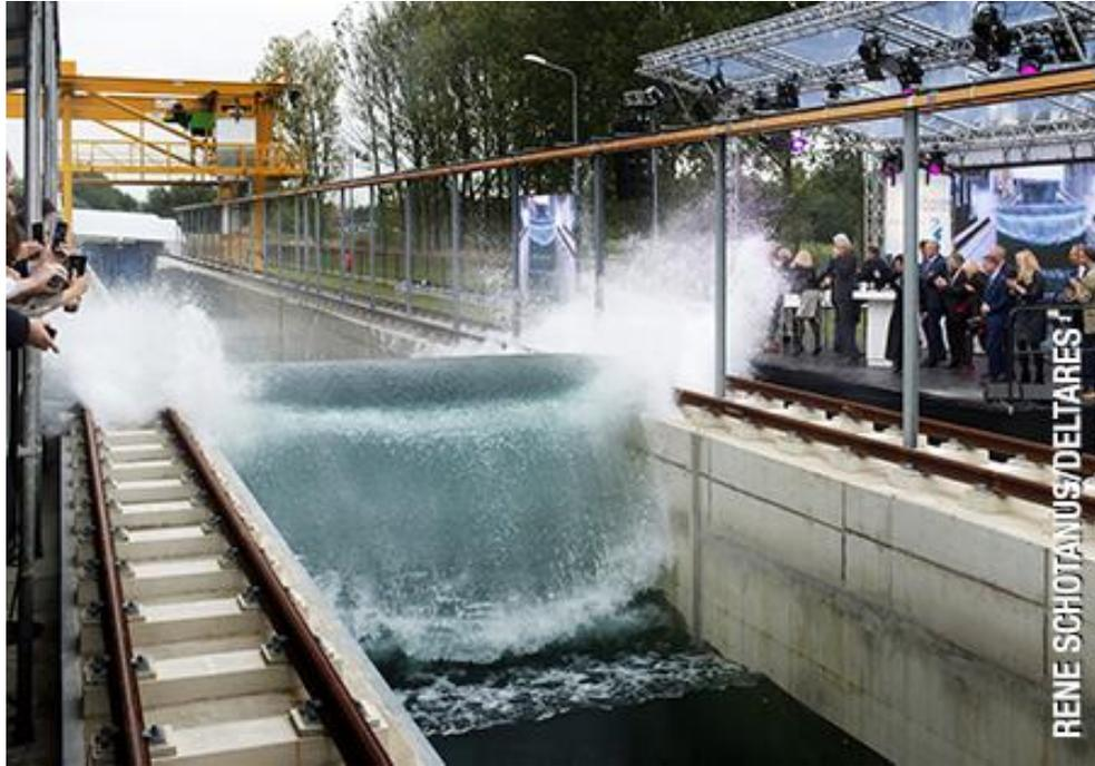
*Figure 7: Wave Generated at Deltares Delta Flume*
