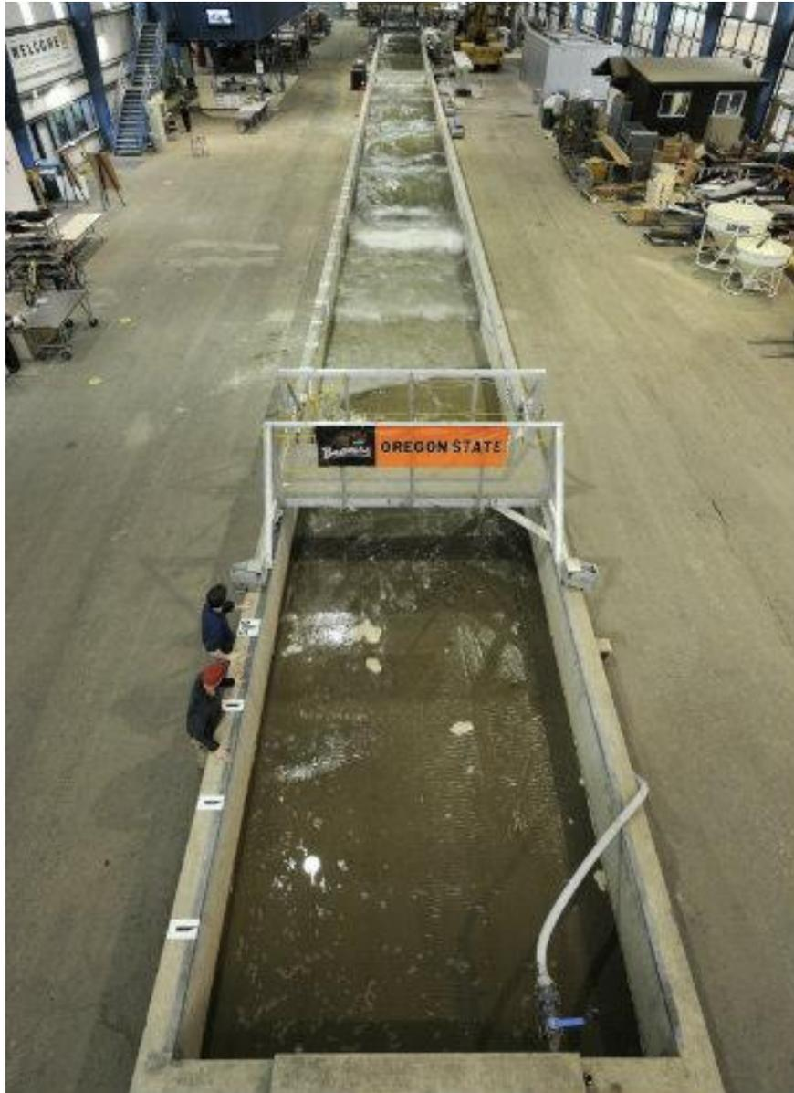
*Figure 8: Large Wave Flume at Oregon State University*
