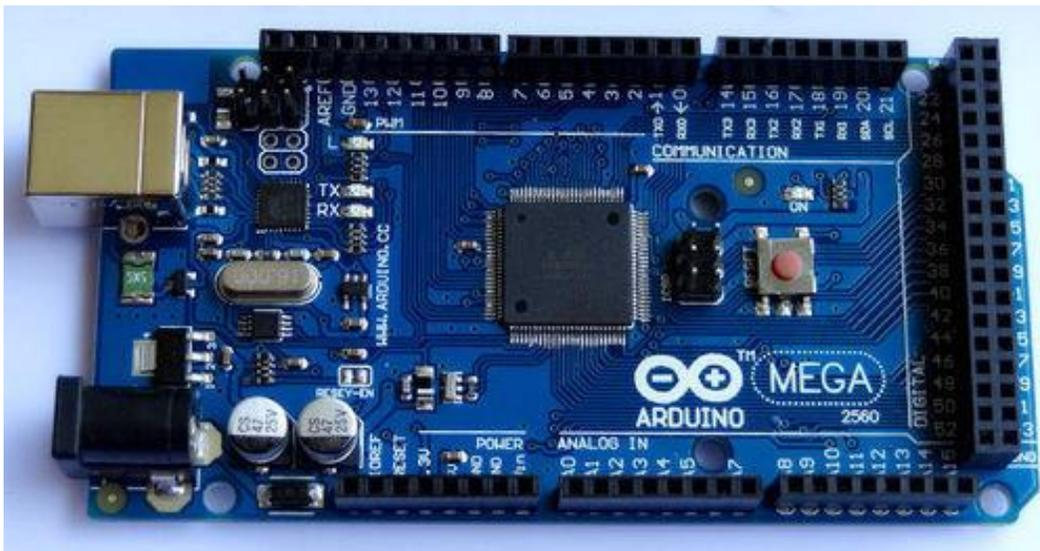
Figure 31: Arduino Mega 2560 Micro-controller
