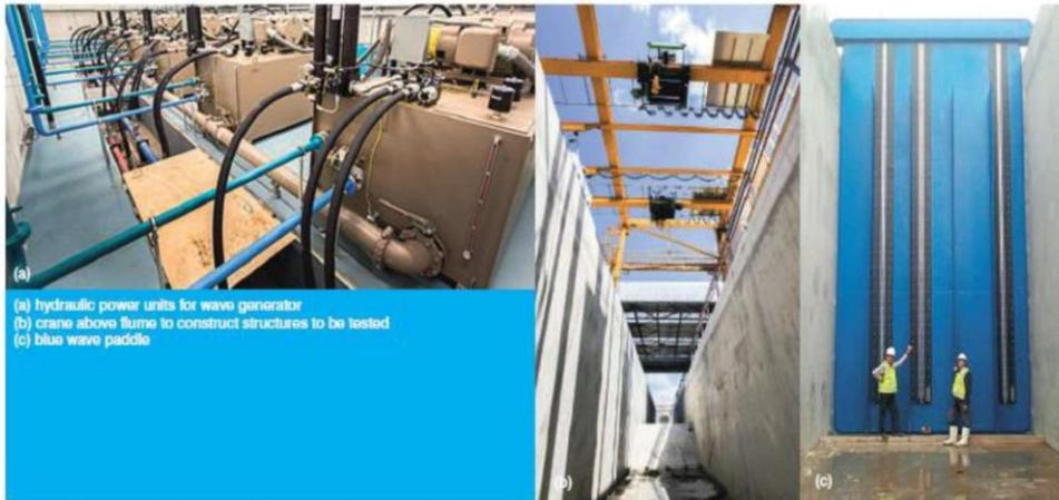
(a) hydraulic power units for wave generator
