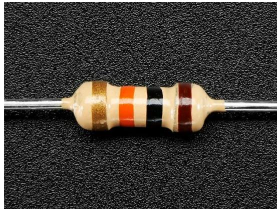
*Figure 35: 10k Resistor*
