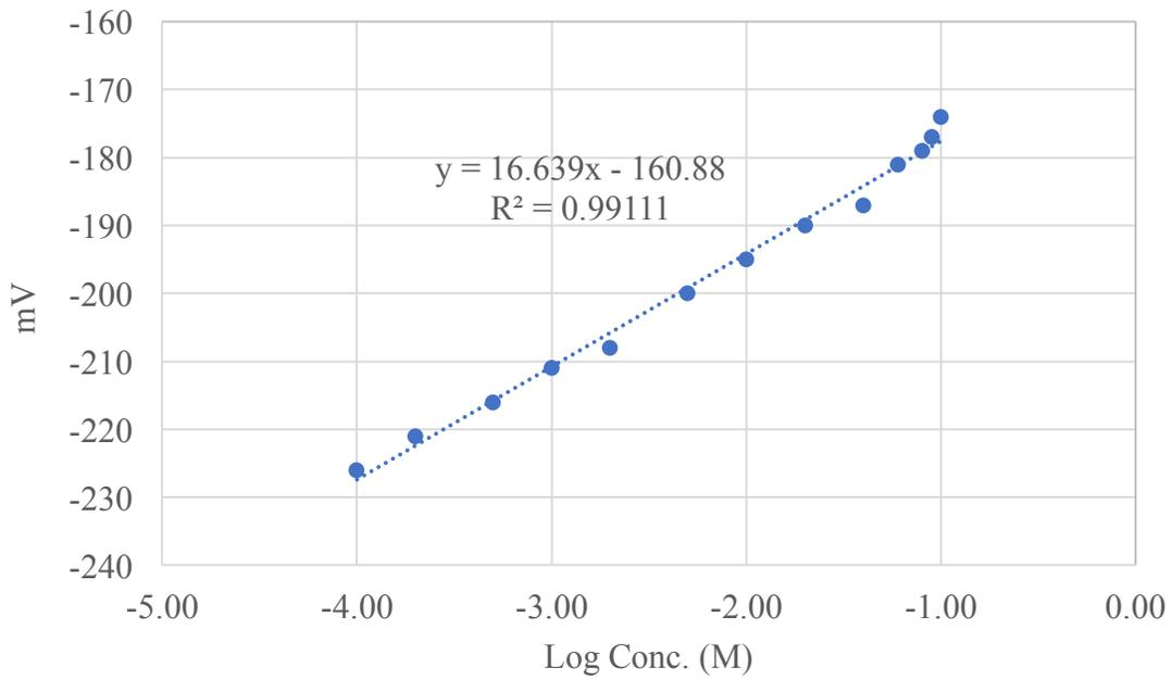
**Figure 131 Calibration curve for lead (taken before 120 minutes reading)**
