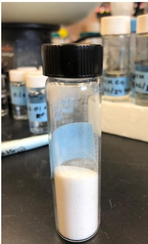
**Figure 15 – ZnCl<sub>2</sub>-MCM-41 after drying in an oven at 373K**
