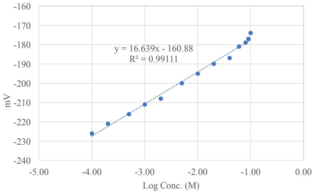
**Figure 127 Calibration curve for lead (before taking 300 minutes reading)**
