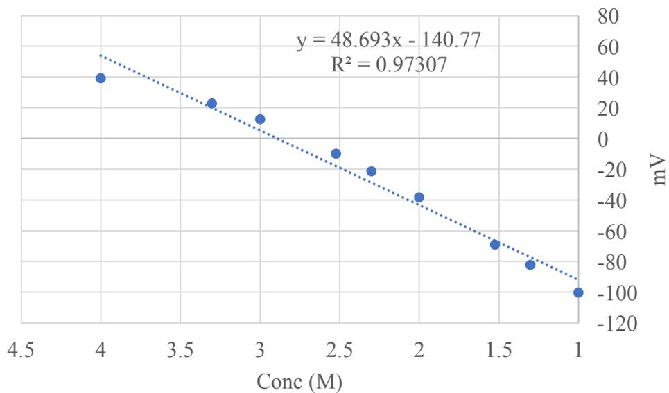
**Figure 140 Initial Calibration curve for nitrate (before taking 24 hours reading for samples with MCM-41 & ZnCl<sub>2</sub>-MCM-41)**
