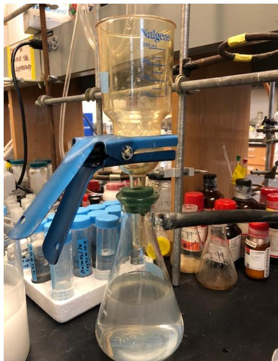
**Figure 12 – Filtration Process for separation of MCM-41 from the solution**
