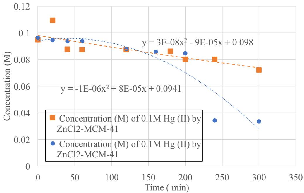
Figure 42 - Experimental: Adsorption of 0.1M Hg (II) by MCM-41 & ZnCl<sub>2</sub>-MCM-41
