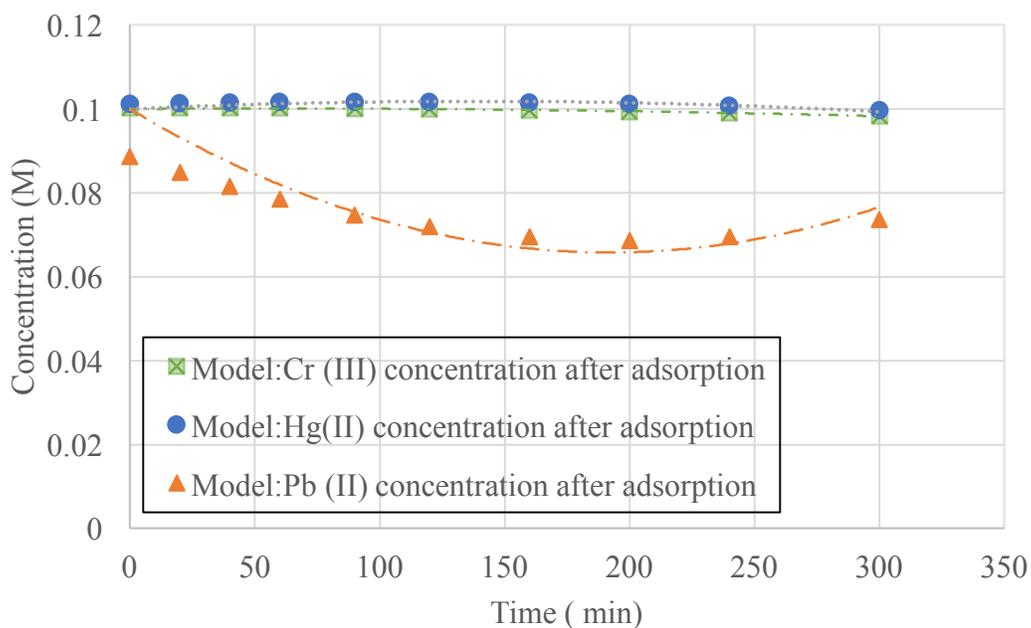
**Figure 71 Model: Adsorption of 0.1M heavy metals (Cr<sup>3+</sup>, Hg<sup>2+</sup>, & Pb<sup>2+</sup>) by ZnCl<sub>2</sub>-MCM-41**
