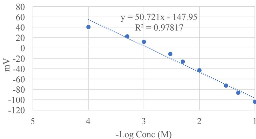
Figure 100 Initial Calibration Curve for NO<sub>3</sub><sup>-</sup> electrode
