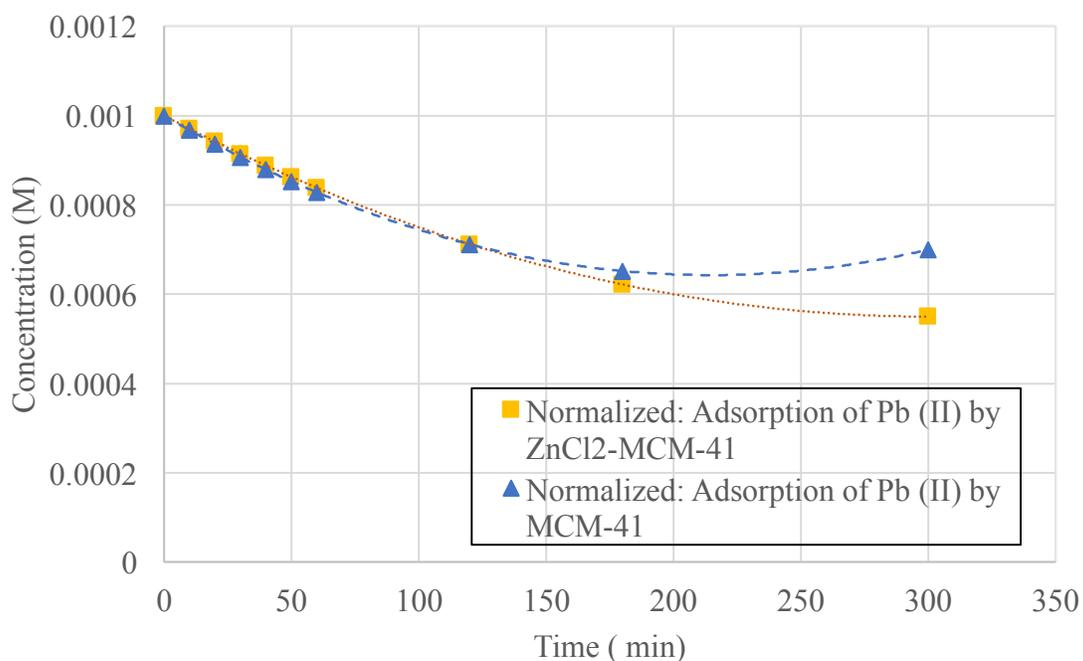
**Figure 40 - Normalized: Adsorption of 0.001M Pb (II) by MCM-41 & ZnCl<sub>2</sub>-MCM-41**
