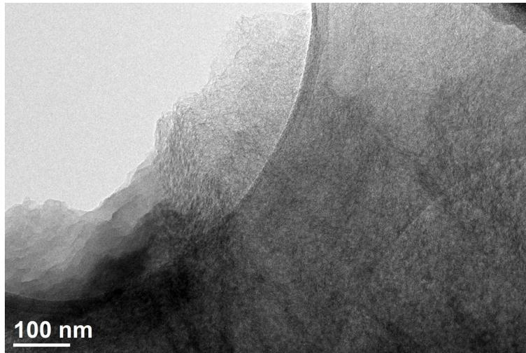
**Figure 17 - TEM image of MCM-41 taken at higher magnification (100nm), showing the morphologies in the sample**
