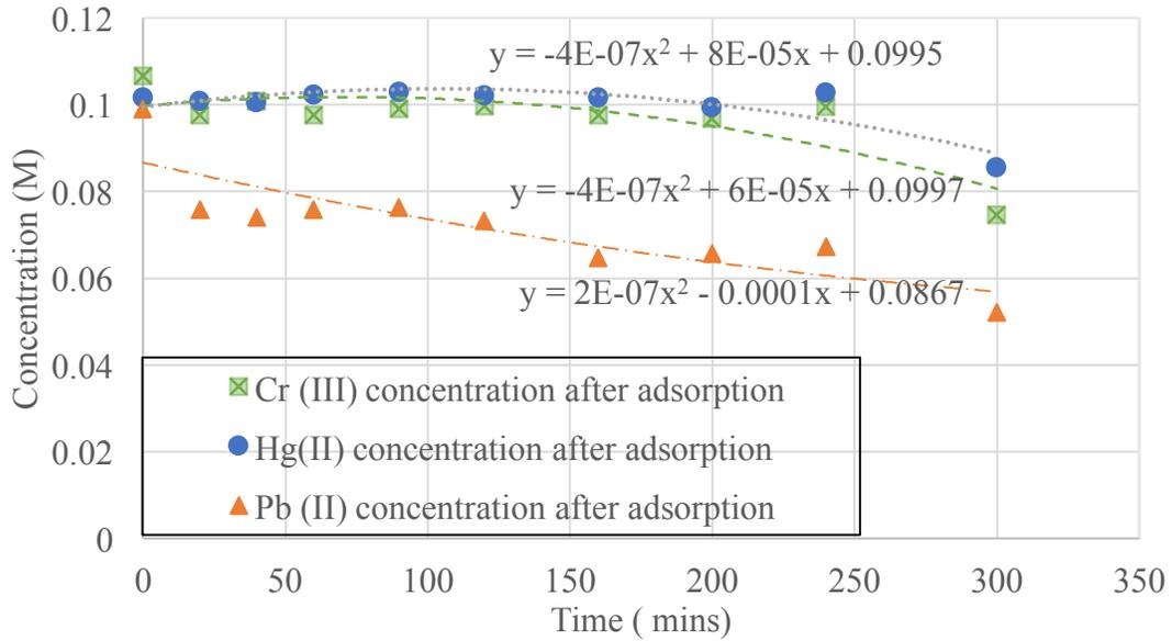
**Figure 66 Experimental: Adsorption of 0.1M heavy metals (Cr<sup>3+</sup>, Hg<sup>2+</sup>, & Pb<sup>2+</sup>) by MCM-41**
