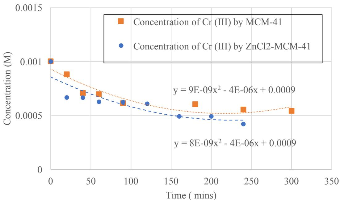
**Figure 62 - Experimental: Adsorption of 0.001M Cr (III) by MCM-41 & ZnCl<sub>2</sub>-MCM-41**
