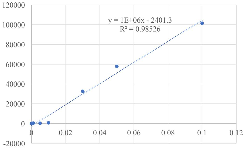
**Figure 142 Calibration curve for Pb (with wavelength 220.53)**
