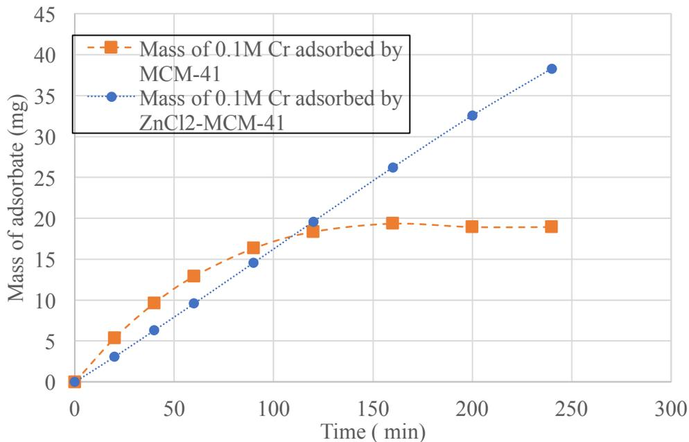
**Figure 57 - Model: Mass of 0.1M Cr (III) adsorbed by MCM-41 & ZnCl<sub>2</sub>-MCM-41**
