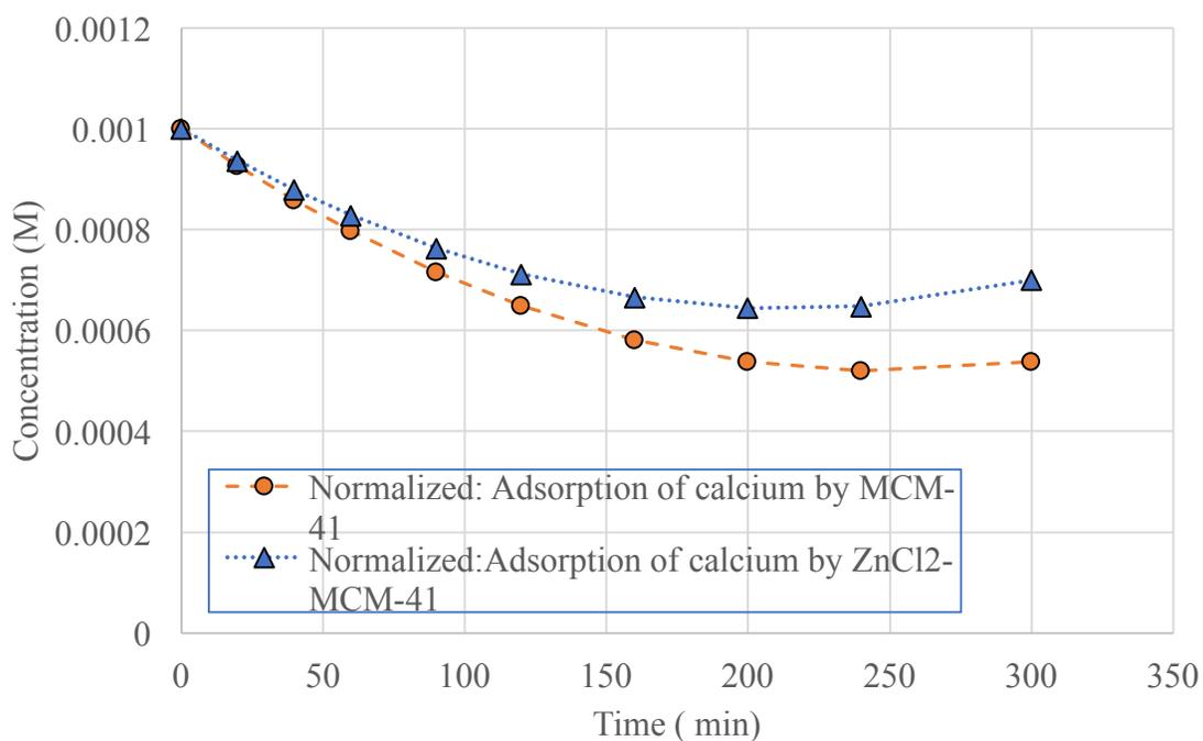
**Figure 77 Normalized: Adsorption of 0.001M  $Ca^{2+}$  ions by MCM-41 and ZnCl<sub>2</sub>-MCM-41**
