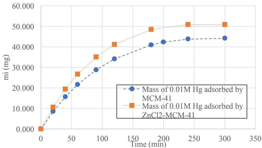
**Figure 49 - Model: Mass of 0.01M Hg (II) adsorbed by MCM-41 & ZnCl<sub>2</sub>-MCM-41**
