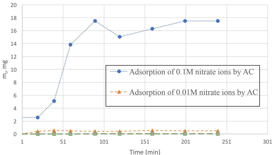
**Figure 112 Mass of  $\text{NO}_3^-$  ions adsorbed by AC**
