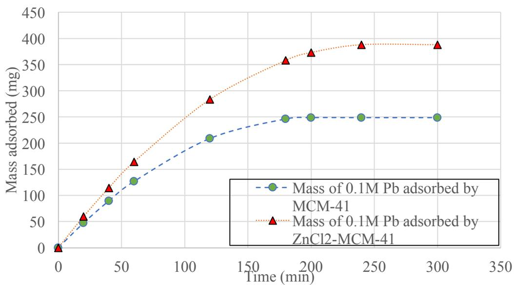
**Figure 33 - Model: Mass of 0.1M Pb (II) (mg) adsorbed by MCM-41 & ZnCl<sub>2</sub>-MCM-41**
