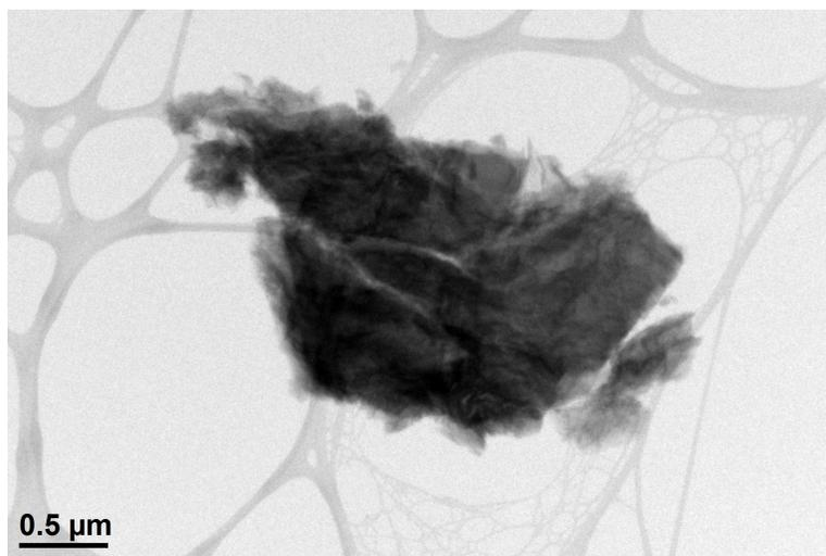
**Figure 19 - TEM image of ZnCl<sub>2</sub>-MCM-41, taken at low magnification (the sample overlays with Lacey Carbon film)**
