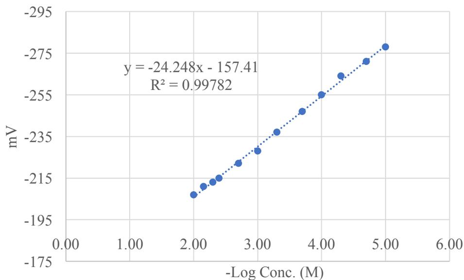
**Figure 115 Initial Calibration curve for lead**
