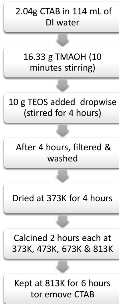
**Figure 10 – Room temperature synthesis of MCM-41**
