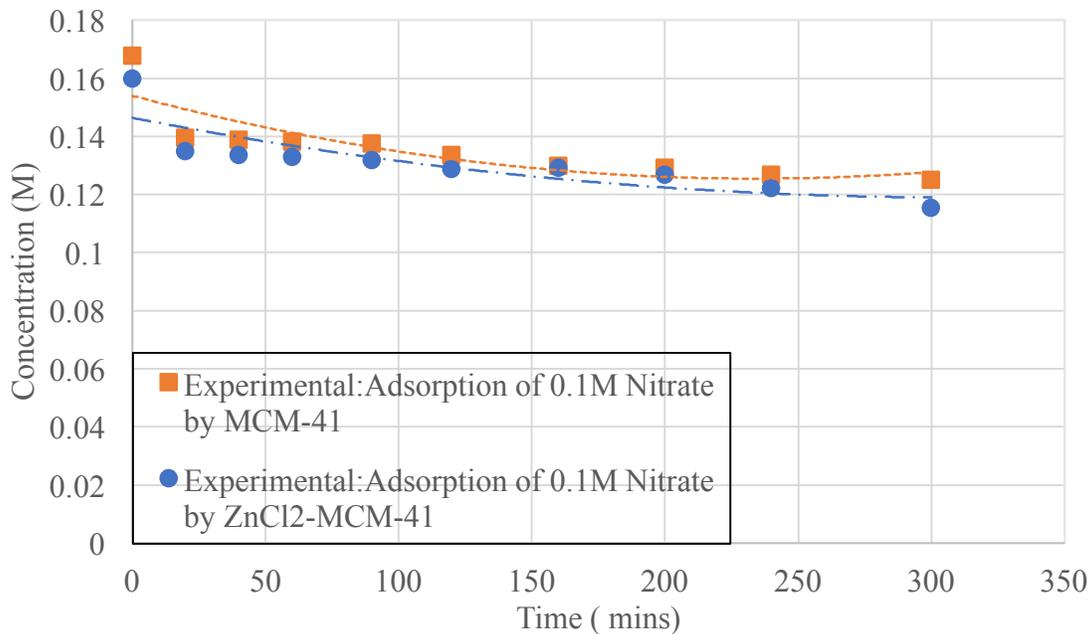
**Figure 105 Experimental: Adsorption of 0.1M NO<sub>3</sub><sup>-</sup> ions by MCM-41 and ZnCl<sub>2</sub>-MCM-41**
