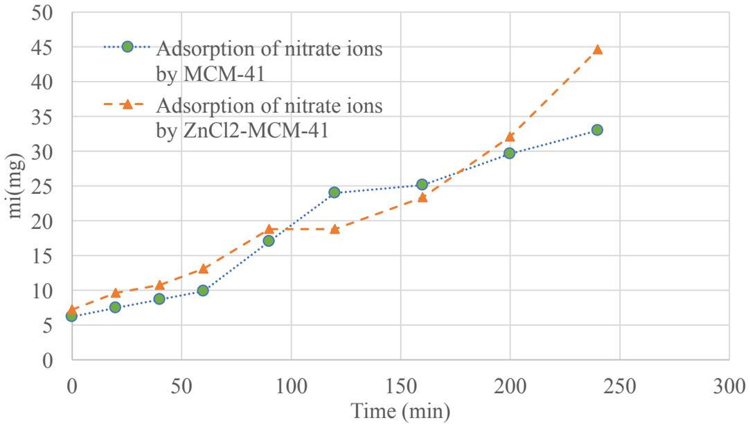
**Figure 106 Mass of 0.1 NO<sub>3</sub><sup>-</sup> ions adsorbed by MCM-41 and ZnCl<sub>2</sub>-MCM-41**
