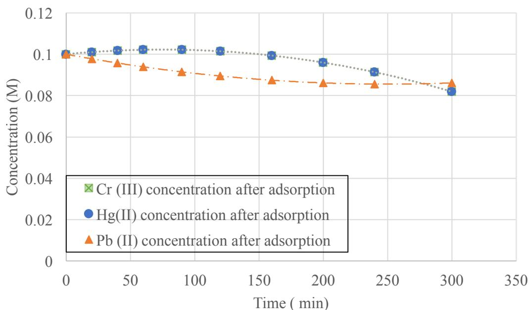
**Figure 68 Normalized: Adsorption of 0.1M heavy metals ( $\text{Cr}^{3+}$ ,  $\text{Hg}^{2+}$ , &  $\text{Pb}^{2+}$ ) by MCM-41**
