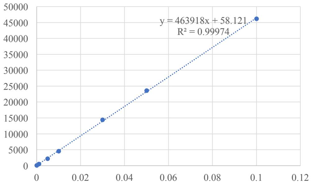
**Figure 143 Calibration curve for Hg (with wavelength 194.164)**
