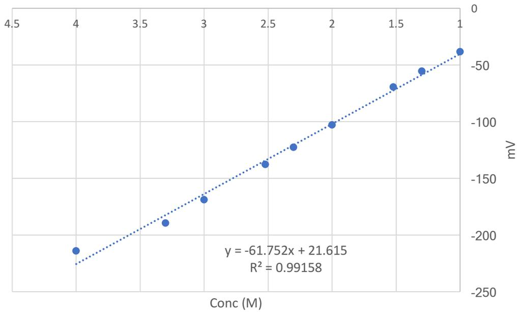
**Figure 136 Calibration curve for potassium (for taking 1 hour reading)**
