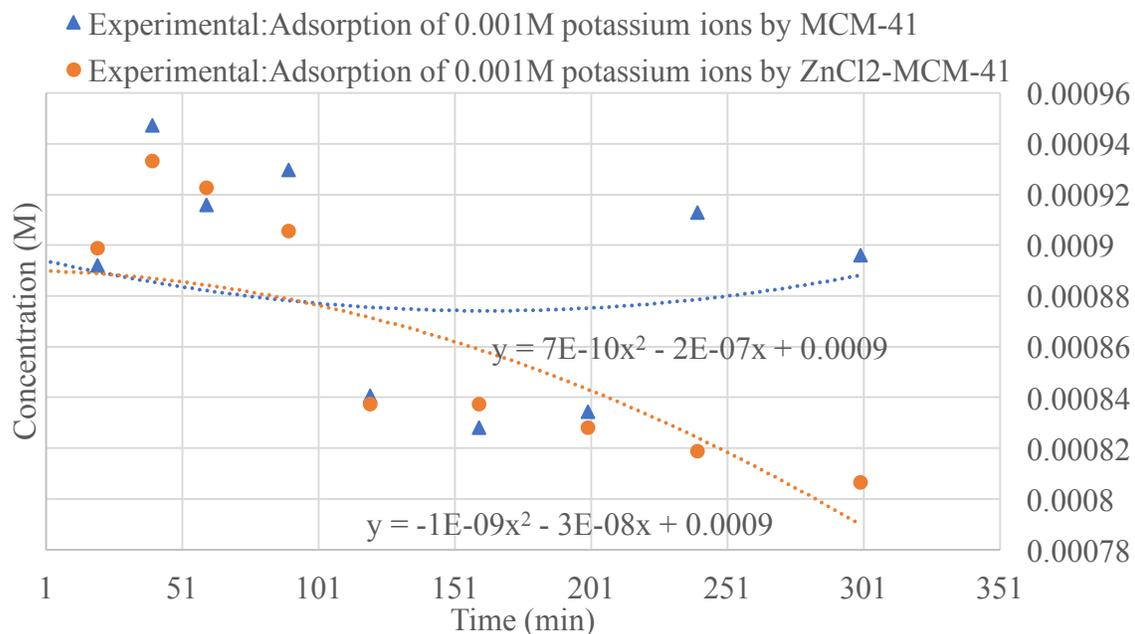
**Figure 88 Experimental: Adsorption of 0.001M K<sup>+</sup> ions by MCM-41 and ZnCl<sub>2</sub>-MCM-41**
