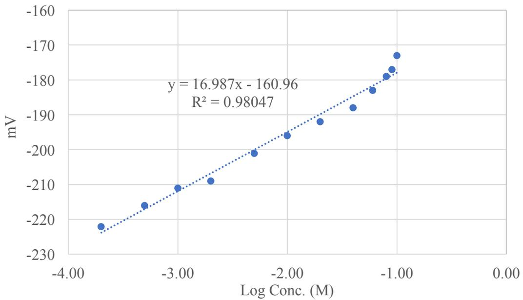
**Figure 126 Calibration curve for lead (before taking 120 minutes reading)**
