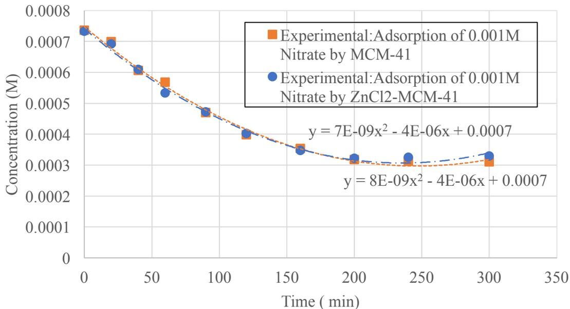
**Figure 101 Experimental: Adsorption of 0.001M NO<sub>3</sub><sup>-</sup> ions by MCM-41 and ZnCl<sub>2</sub>-MCM-41**
