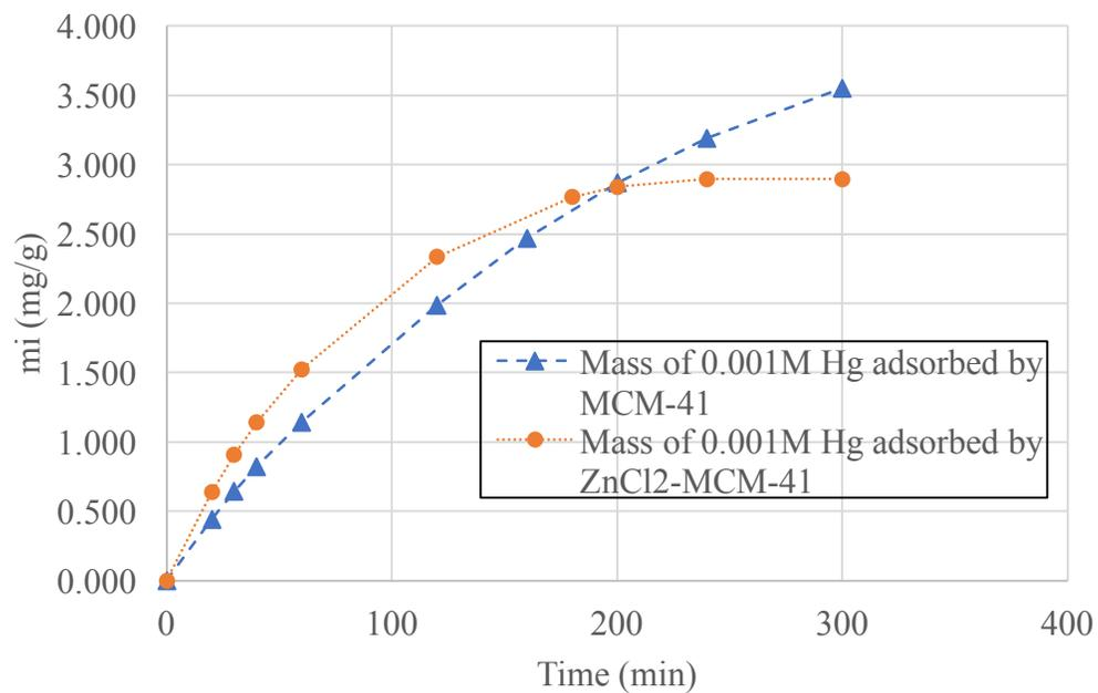
**Figure 53 – Model: Mass of 0.001M Hg (II) adsorbed by MCM-41 & ZnCl<sub>2</sub>-MCM-41**
