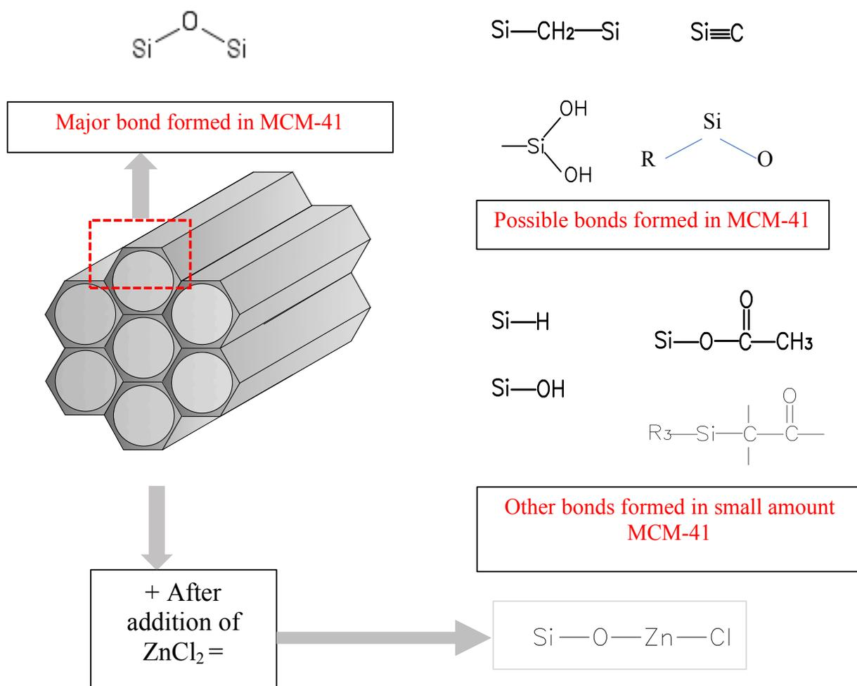
**Figure 25 MCM-41 and ZnCl<sub>2</sub>-MCM-41 structure**
