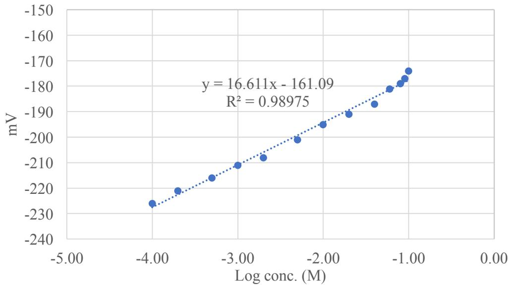
**Figure 128 Calibration curve for lead (before taking 24 hours reading)**
