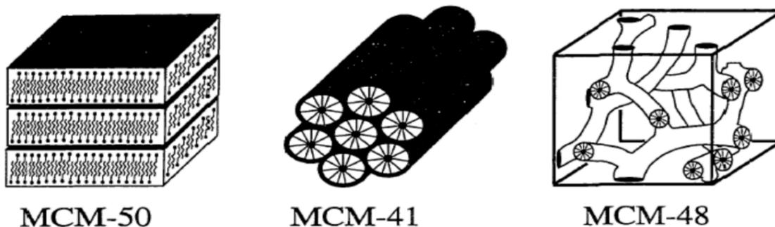
**Figure 1- Schematic Diagram of MCM-50 (layered), MCM-41 (hexagonal), and MCM-48 (cubic) (Alothman 2012)**
