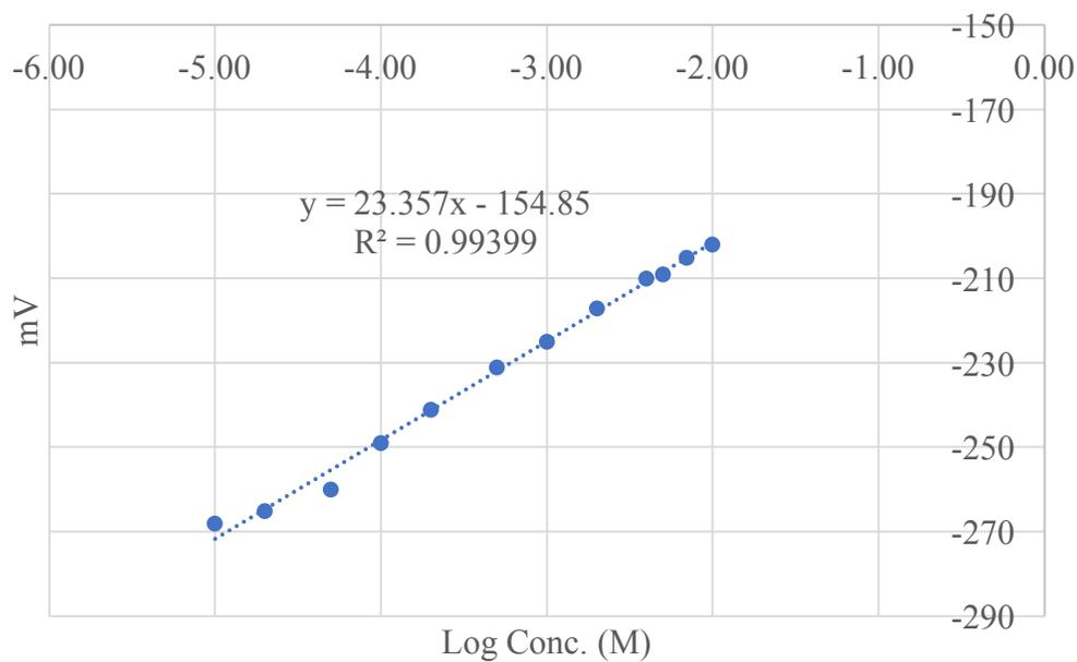
**Figure 119 Initial Calibration curve for lead (taken before 1 hour reading)**
