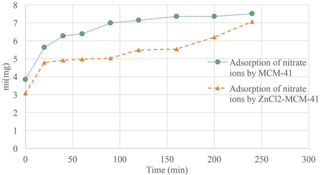
**Figure 104 Mass of 0.01 NO<sub>3</sub><sup>-</sup> ions adsorbed by MCM-41 and ZnCl<sub>2</sub>-MCM-41**
