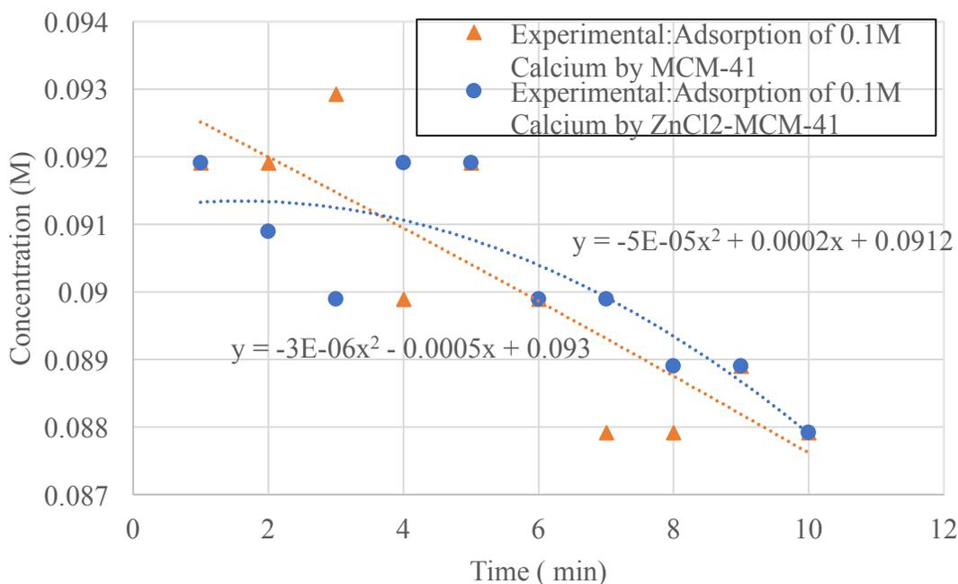
**Figure 83 Experimental: Adsorption of 0.1M Ca<sup>2+</sup> ions by MCM-41 and ZnCl<sub>2</sub>-MCM-41**
