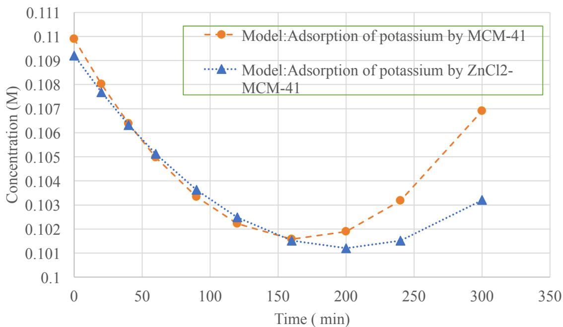
**Figure 97 Model: Adsorption of 0.1M K<sup>+</sup> ions by MCM-41 and ZnCl<sub>2</sub>-MCM-41**
