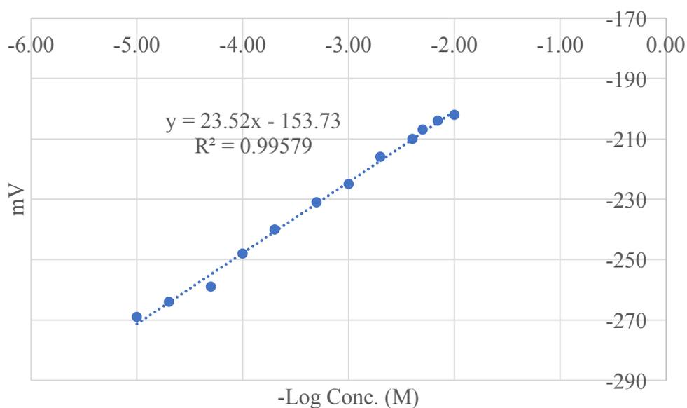
**Figure 118 Initial Calibration curve for lead (taken before taking 30 minutes reading)**
