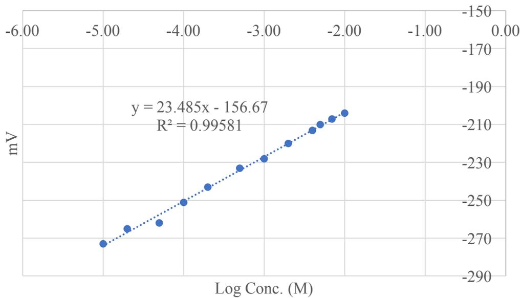
**Figure 121 Initial Calibration curve for lead (taken before 180 minutes reading)**
