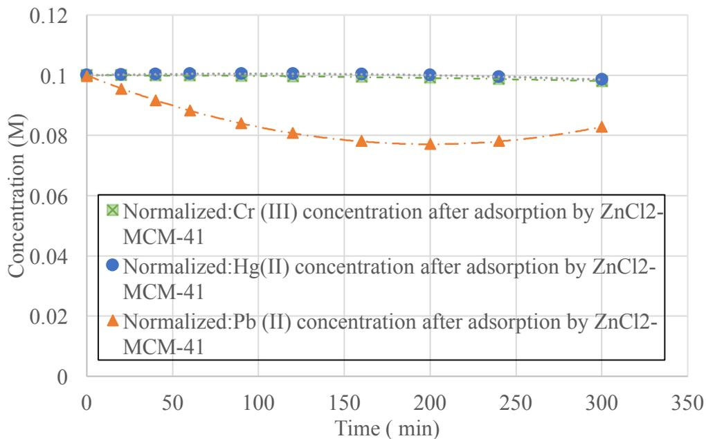
**Figure 72 Normalized: Adsorption of 0.1M heavy metals (Cr<sup>3+</sup>, Hg<sup>2+</sup>, & Pb<sup>2+</sup>) by MCM-41**
