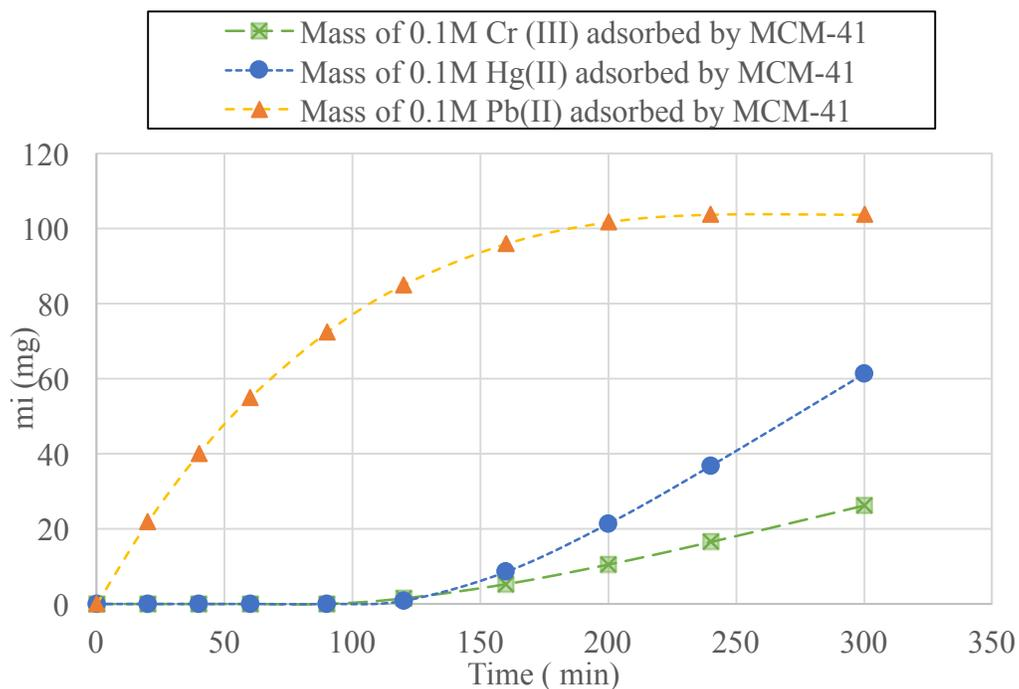
**Figure 69 Mass of the adsorbate (mg) 0.1M heavy metals ( $\text{Cr}^{3+}$ ,  $\text{Hg}^{2+}$ , &  $\text{Pb}^{2+}$ ) adsorbed by MCM-41**
