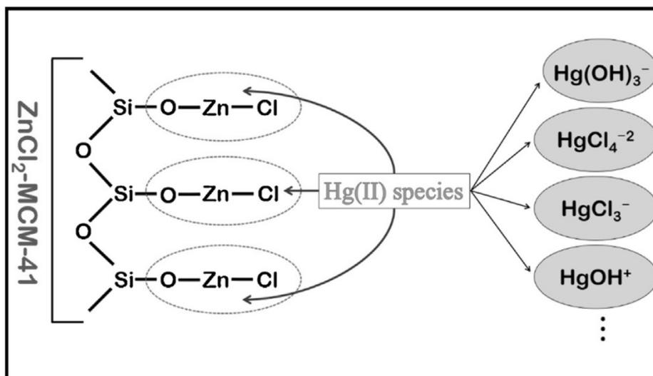
Figure 9 - Adsorption mechanism of Hg (II) species by  $ZnCl_2$ -MCM-41 (Raji & Pakizeh 2014)
