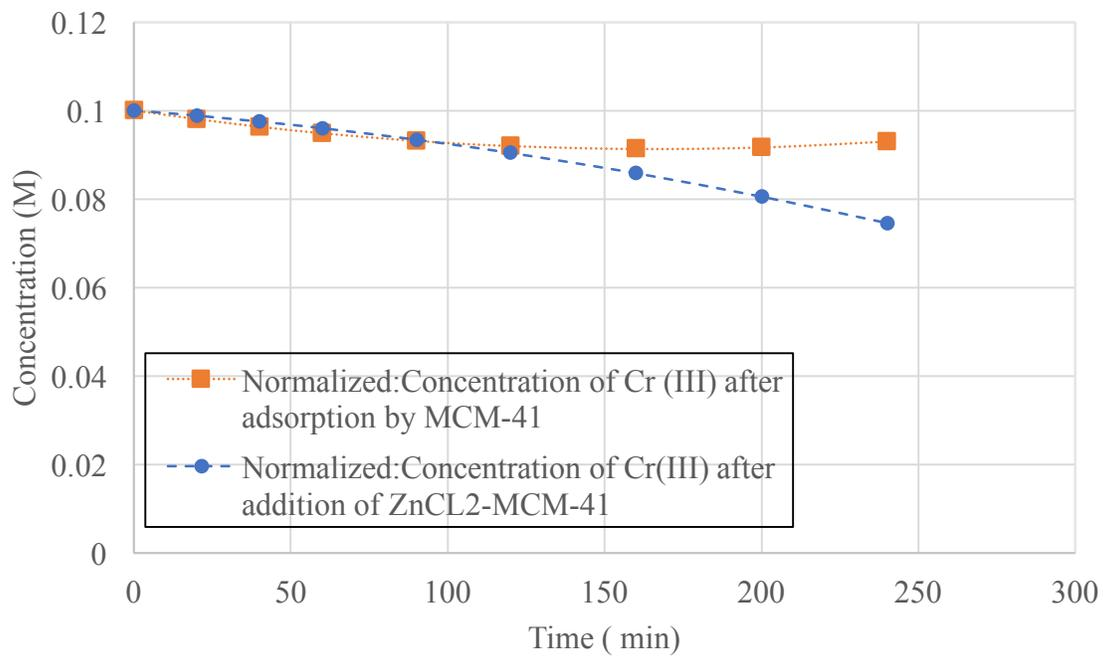
**Figure 56 - Normalized: Adsorption of 0.1M Cr (III) by MCM-41 & ZnCl<sub>2</sub>-MCM-41**
