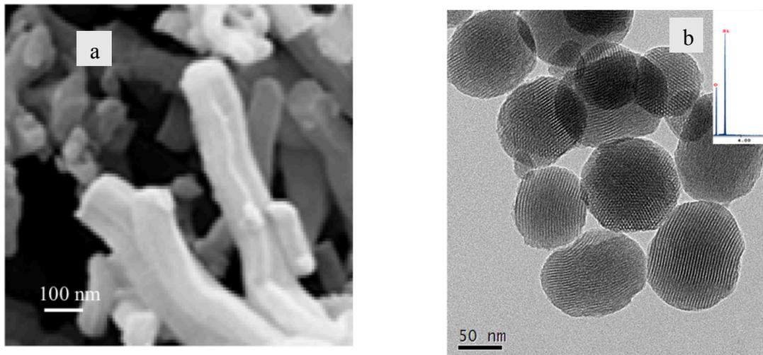
**Figure 3 -a) SEM image of MCM-41 (Bao et al. 2015) and b) TEM image of MCM-41 (Dai et al. 2014)**
