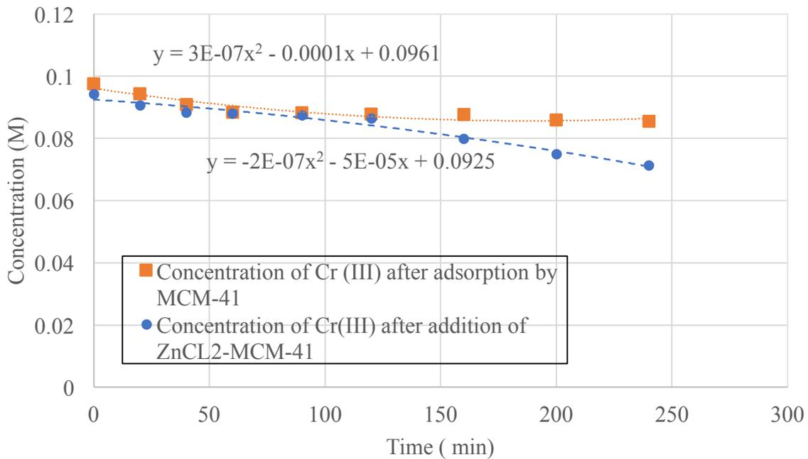
**Figure 54 - Experimental: Adsorption of 0.1M Cr (III) by MCM-41 & ZnCl<sub>2</sub>-MCM-41**
