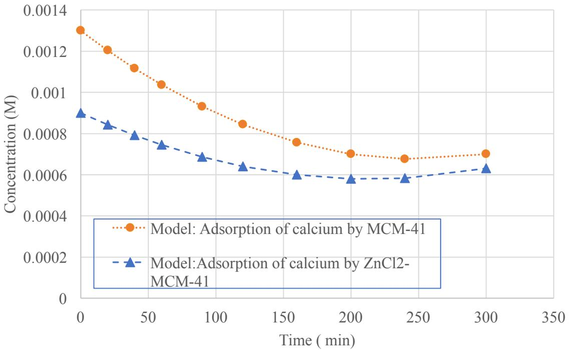
**Figure 76 Model: Adsorption of 0.001M Ca<sup>2+</sup> ions by MCM-41 and ZnCl<sub>2</sub>-MCM-41**
