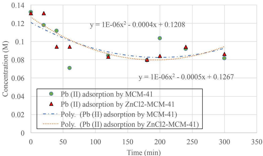
**Figure 30 - Experimental: Adsorption of 0.1M Pb (II) by MCM-41 & ZnCl<sub>2</sub>-MCM-41**
