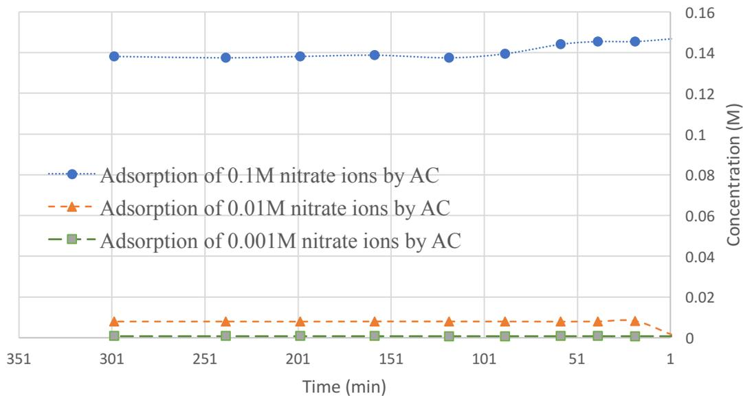
**Figure 111 Adsorption of NO<sub>3</sub><sup>-</sup> ions by AC**
