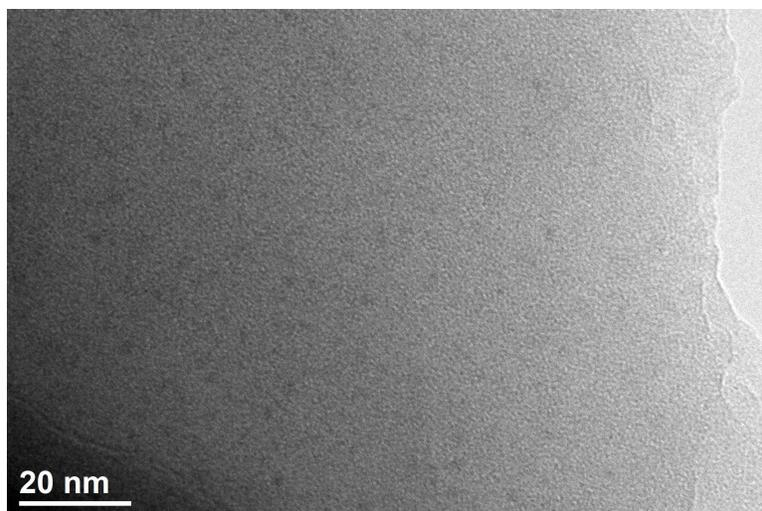
**Figure 23 - TEM image of ZnCl<sub>2</sub>-MCM-41 with the randomly distributed features (approx. 2nm) in darker contrast**
