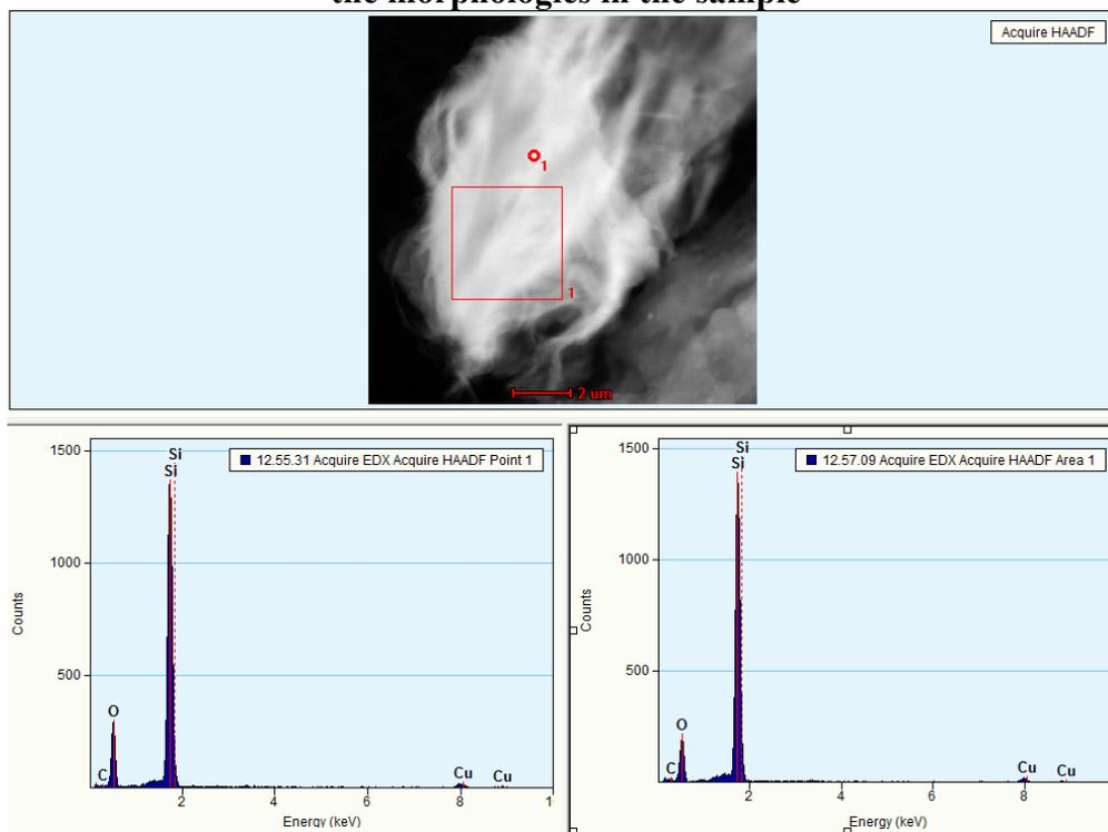
Figure 22 - STEM Z-contrast image of ZnCl<sub>2</sub>-MCM-41 showing presence of oxygen and silica in the material
