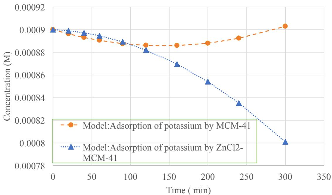
**Figure 89 Model: Adsorption of 0.001M K<sup>+</sup> ions by MCM-41 and ZnCl<sub>2</sub>-MCM-41**
