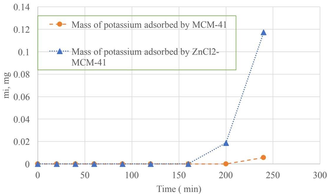
**Figure 95 Mass of 0.01 K<sup>+</sup> ions adsorbed by MCM-41 and ZnCl<sub>2</sub>-MCM-41**
