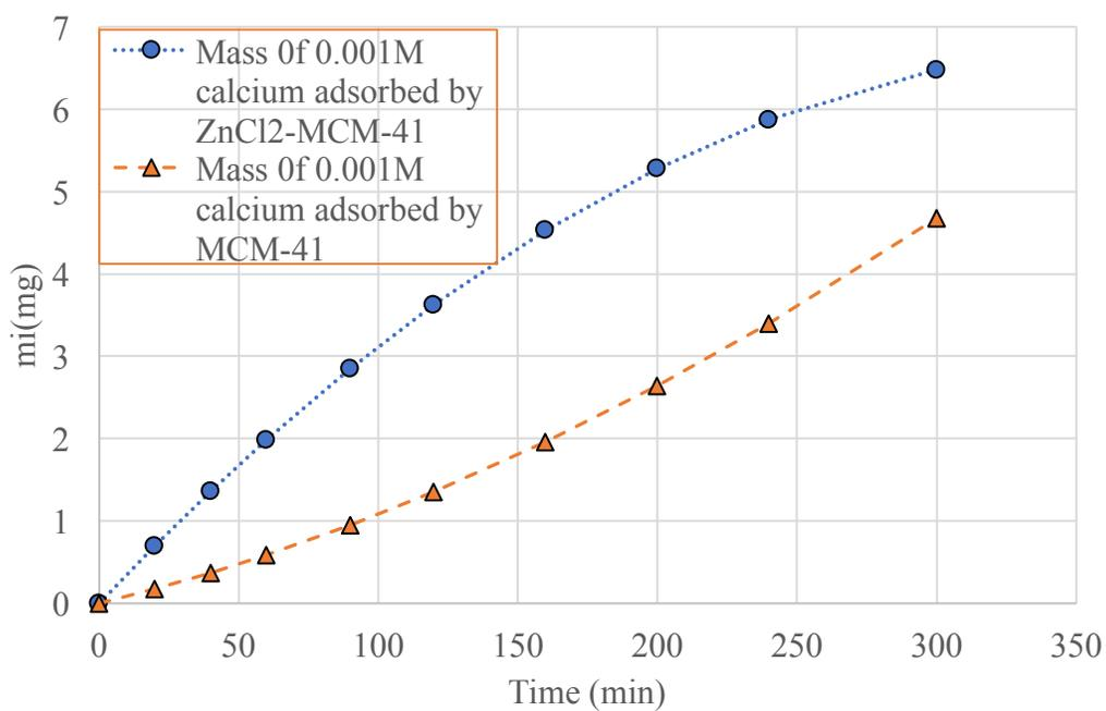
**Figure 86 Mass of  $0.1\text{M Ca}^{2+}$  ions adsorbed by MCM-41 and ZnCl<sub>2</sub>-MCM-41**
