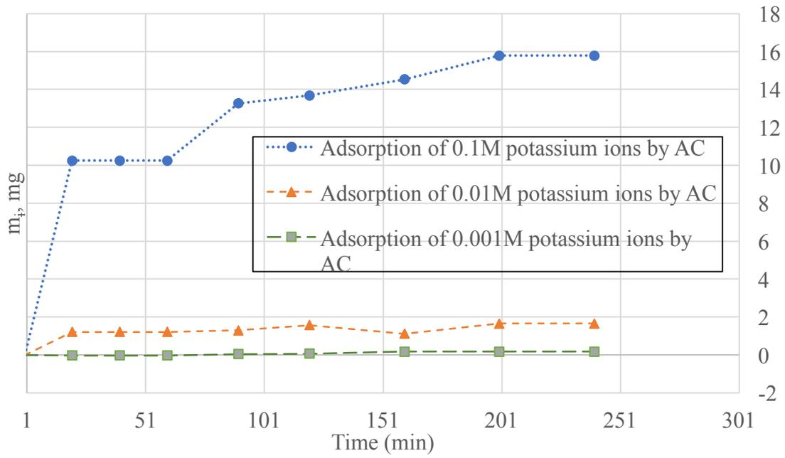
**Figure 114 Mass of  $K^+$  ions adsorbed by AC**
