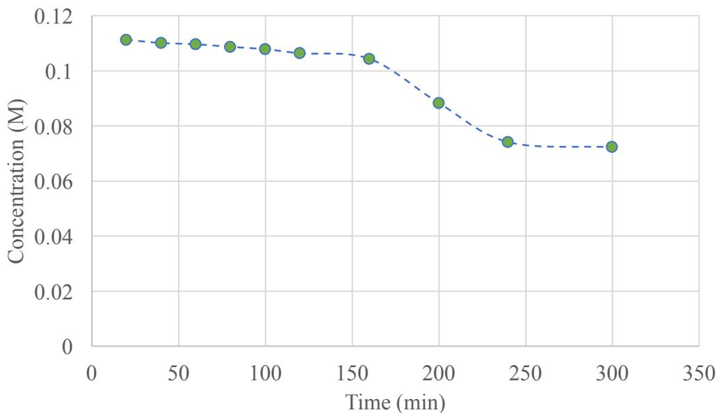
**Figure 108 Adsorption of 0.1M lead by AC**
