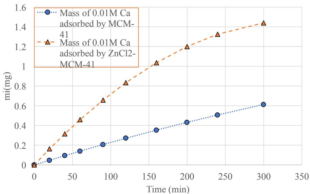
**Figure 82 Mass of 0.01 Ca<sup>2+</sup> ions adsorbed by MCM-41 and ZnCl<sub>2</sub>-MCM-41**
