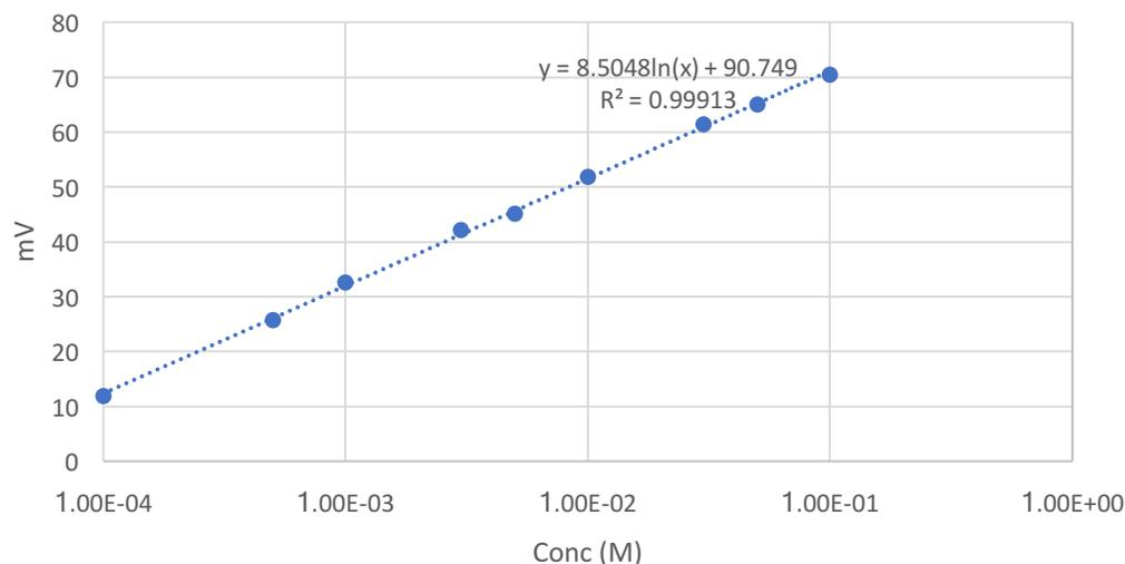
**Figure 107 Calibration Curve for Calcium electrode**
