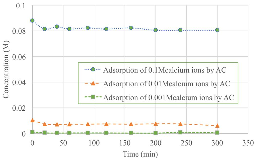
**Figure 109 Experimental: Adsorption of Ca<sup>2+</sup> ions by AC**
