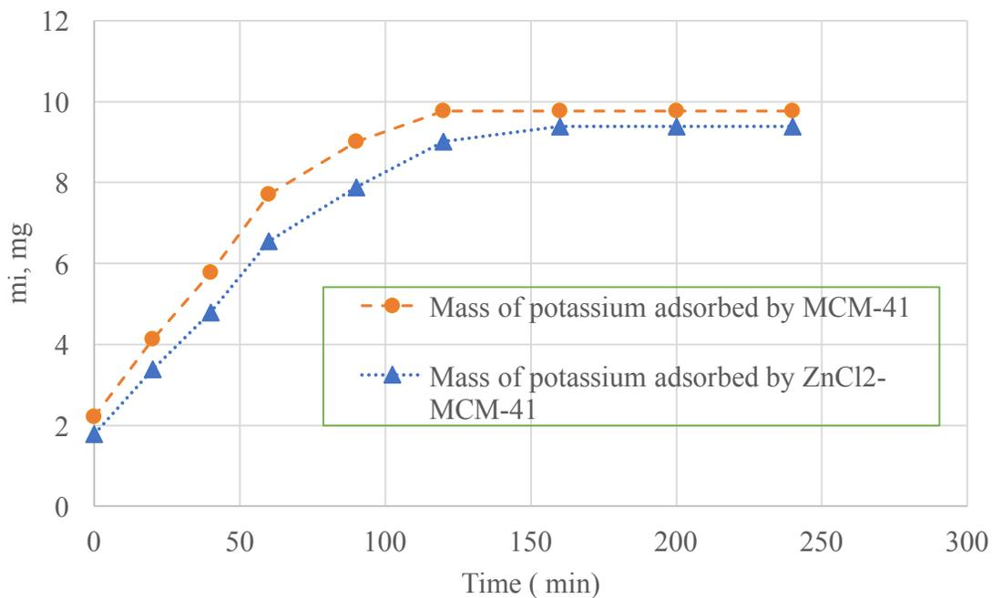
**Figure 99 Mass of 0.1 K<sup>+</sup> ions adsorbed by MCM-41 and ZnCl<sub>2</sub>-MCM-41**
