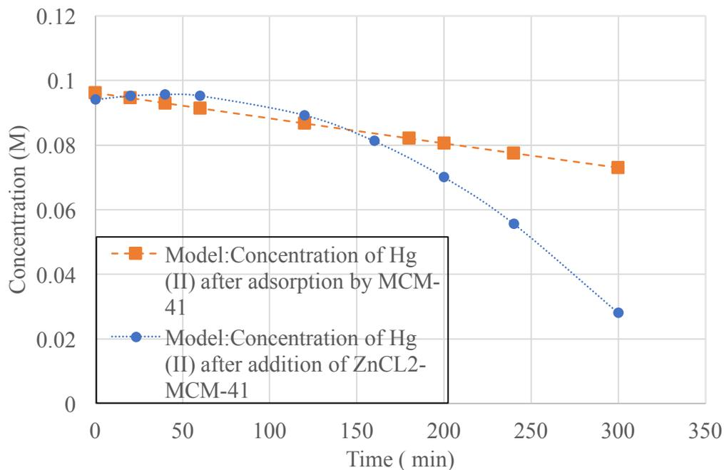
**Figure 43 - Model: Adsorption of 0.1M Hg (II) by MCM-41 & ZnCl<sub>2</sub>-MCM-41**
