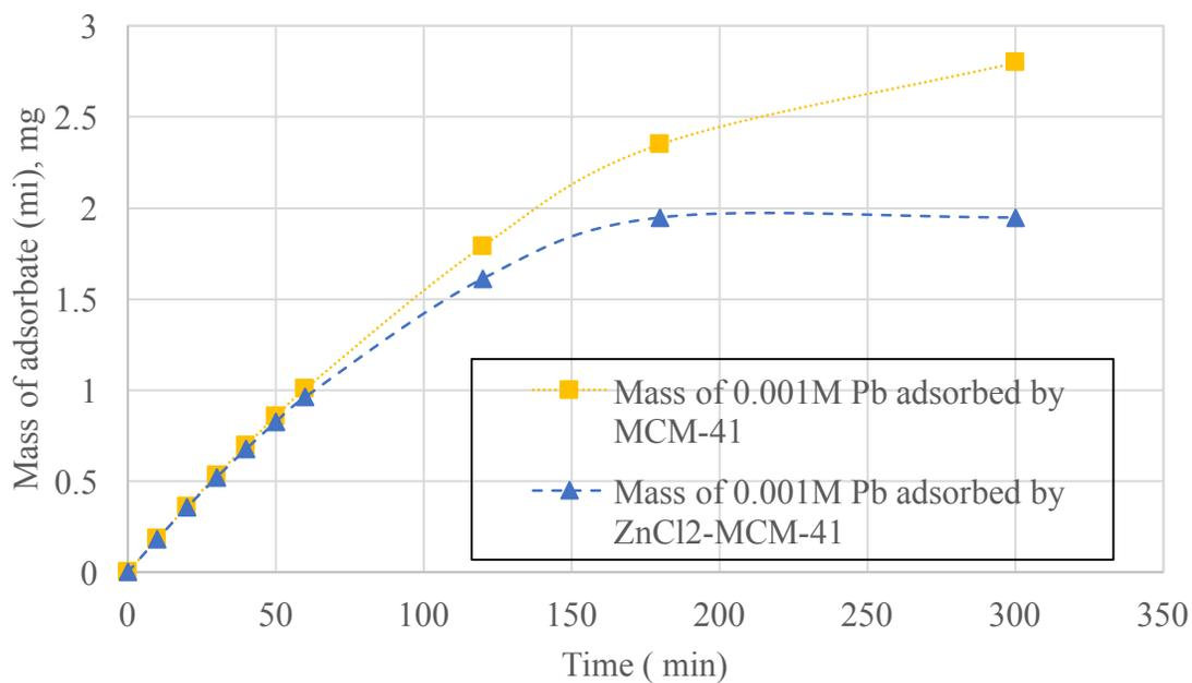
**Figure 41 - Model: Mass of 0.001M Pb (II) adsorbed by MCM-41 & ZnCl<sub>2</sub>-MCM-41**
