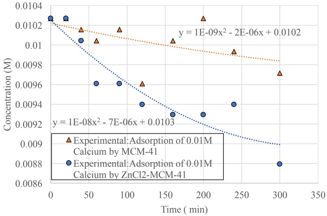
**Figure 79 Experimental: Adsorption of 0.01M Ca<sup>2+</sup> ions by MCM-41 and ZnCl<sub>2</sub>-MCM-41**
