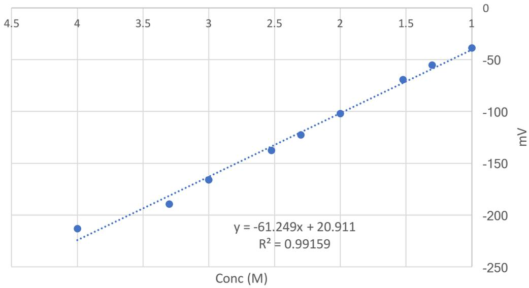
**Figure 135 Initial Calibration curve for potassium**
