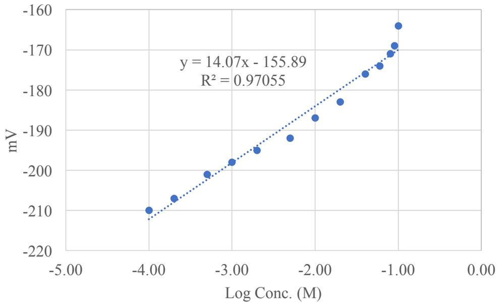
**Figure 130 Calibration curve for lead (taken before 1 hour reading)**
