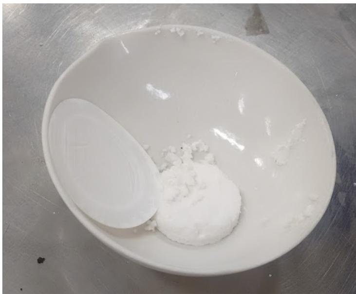
**Figure 13 – Filtered and washed MCM-41 (after 4 hours stirring)**
