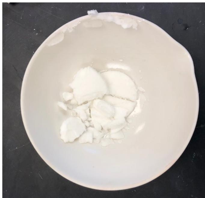
**Figure 14 – MCM-41 after completion of calcination at 813K**
