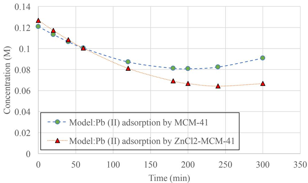
**Figure 31 - Model: Adsorption of 0.1M Pb (II) by MCM-41 & ZnCl<sub>2</sub>-MCM-41**
