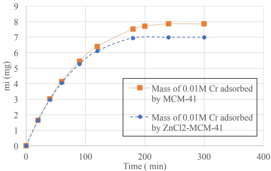
**Figure 61 - Model: Mass of 0.01M Cr (III) adsorbed by MCM-41 & ZnCl<sub>2</sub>-MCM-41**
