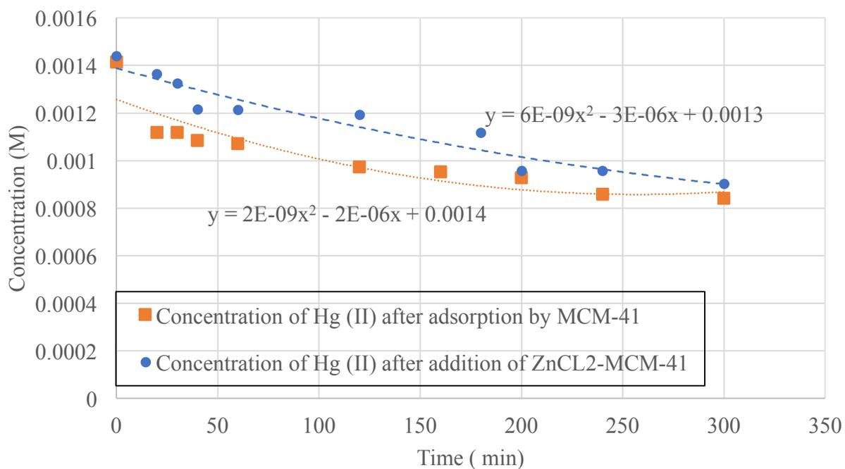
Figure 50 – Experimental: Adsorption of 0.001M Hg (II) by MCM-41 & ZnCl<sub>2</sub>-MCM-41
