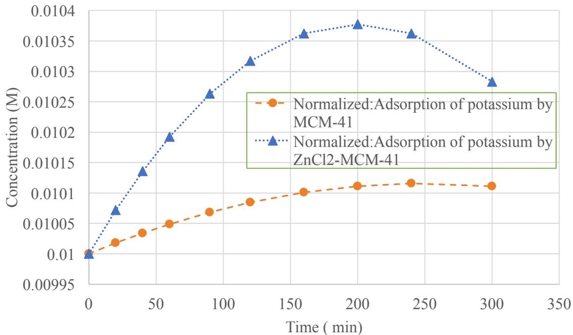
**Figure 94 Normalized: Adsorption of 0.01M K<sup>+</sup> ions by MCM-41 and ZnCl<sub>2</sub>-MCM-41**
