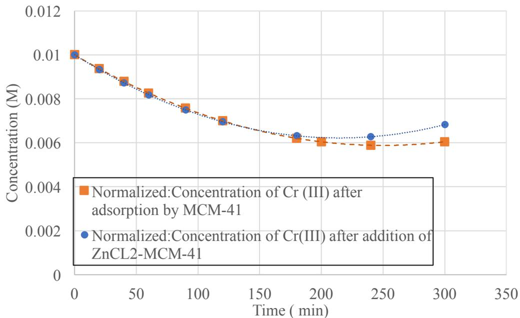
**Figure 60 - Normalized: Adsorption of 0.01M Cr (III) by MCM-41 & ZnCl<sub>2</sub>-MCM-41**
