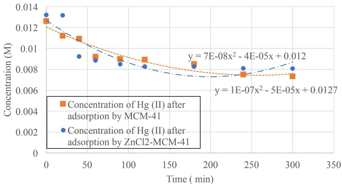
**Figure 46 – Experimental: Adsorption of 0.01M Hg (II) by MCM-41 & ZnCl<sub>2</sub>-MCM-41**
