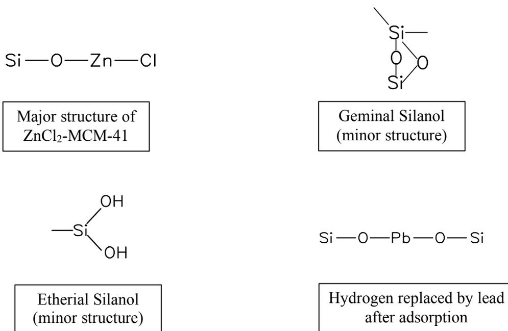
**Figure 28 ZnCl<sub>2</sub>-MCM-41 structure composition before and after adsorption**
