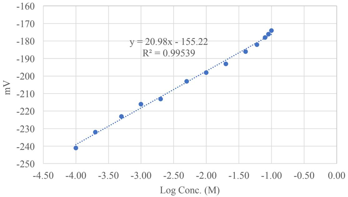
**Figure 125 Calibration curve for lead (before taking 50 & 80 minutes reading)**
