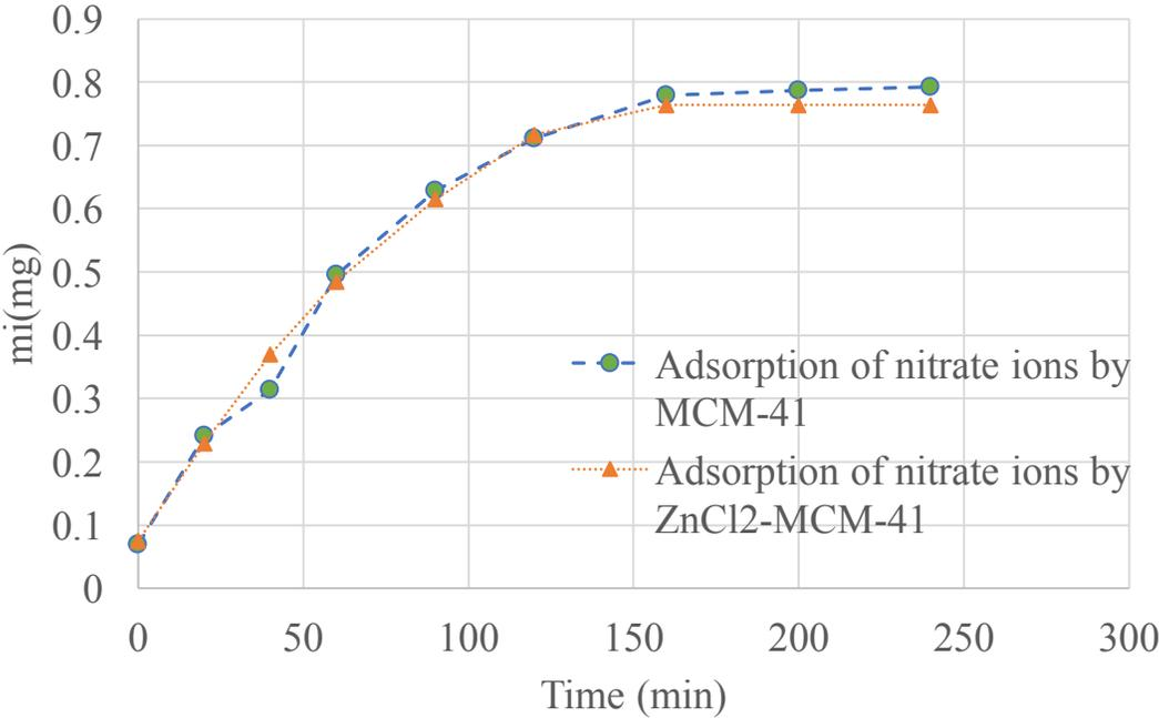
**Figure 102 Mass of 0.001 NO<sub>3</sub><sup>-</sup> ions adsorbed by MCM-41 and ZnCl<sub>2</sub>-MCM-41**
