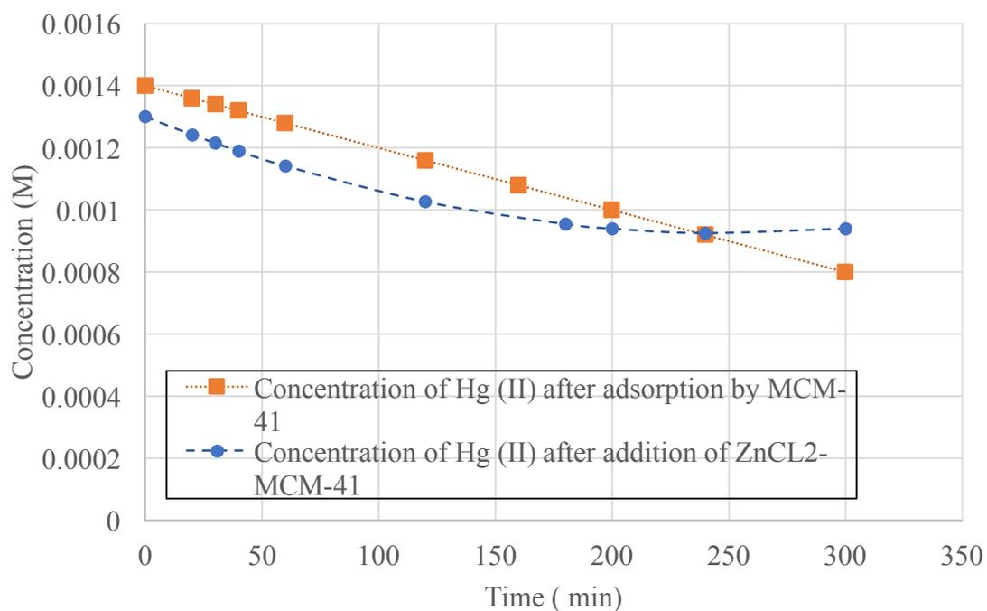
**Figure 51 – Model: Adsorption of 0.001M Hg (II) by MCM-41 & ZnCl<sub>2</sub>-MCM-41**
