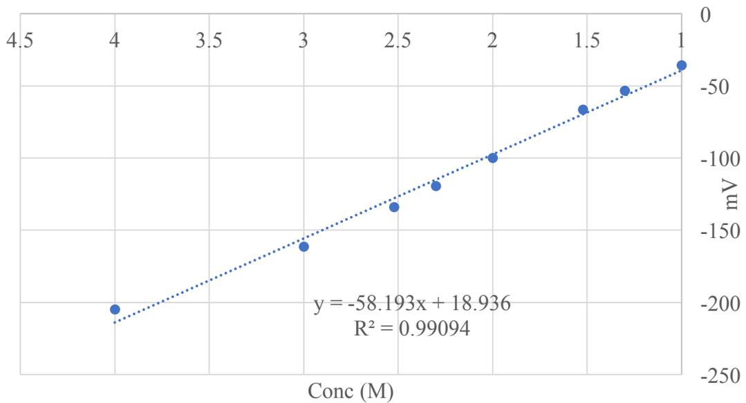
**Figure 138 Calibration curve for potassium (for taking 24 hours reading)**
