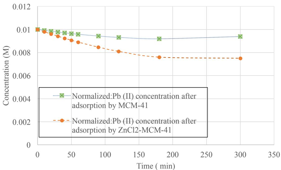
**Figure 36 - Normalized: Adsorption of 0.01M Pb (II) by MCM-41 & ZnCl<sub>2</sub>-MCM-41**
