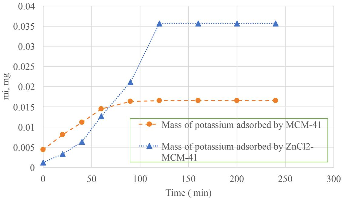
**Figure 91 Mass of 0.001 K<sup>+</sup> ions adsorbed by MCM-41 and ZnCl<sub>2</sub>-MCM-41**
