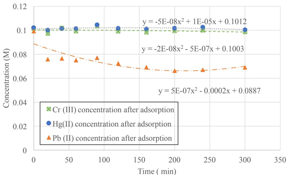
**Figure 70 Experimental: Adsorption of 0.1M heavy metals (Cr<sup>3+</sup>, Hg<sup>2+</sup>, & Pb<sup>2+</sup>) by ZnCl<sub>2</sub>-MCM-41**
