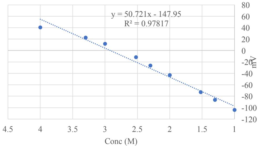
**Figure 139 Initial Calibration curve for nitrate**
