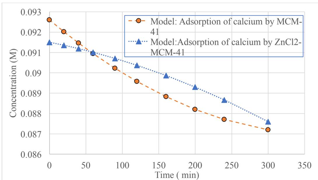
**Figure 84 Model: Adsorption of 0.1M Ca<sup>2+</sup> ions by MCM-41 and ZnCl<sub>2</sub>-MCM-41**
