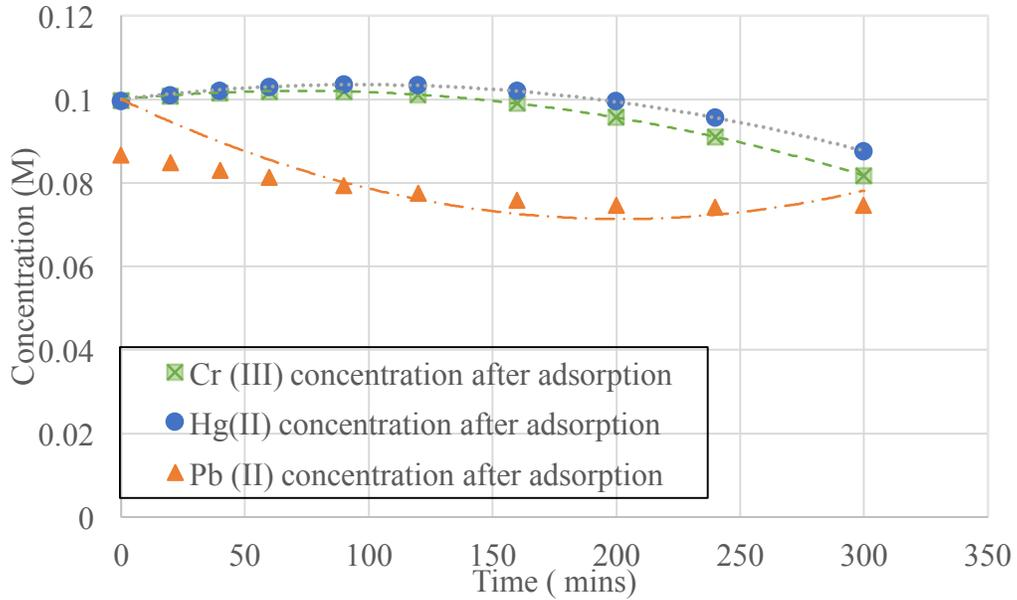
**Figure 67 Model: Adsorption of 0.1M heavy metals (Cr<sup>3+</sup>, Hg<sup>2+</sup>, & Pb<sup>2+</sup>) by MCM-41**
