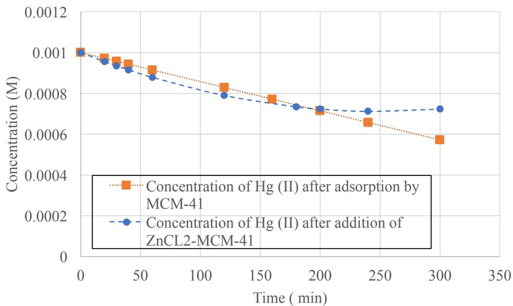
**Figure 52 – Normalized: Adsorption of 0.001M Hg (II) by MCM-41 & ZnCl<sub>2</sub>-MCM-41**
