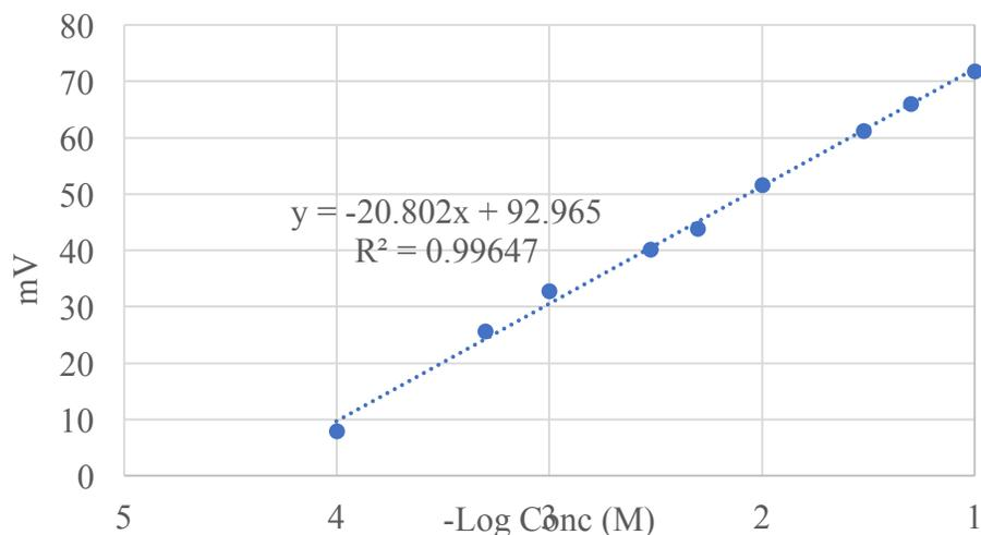
**Figure 74 Initial Calibration Curve for Ca<sup>2+</sup> electrode**
