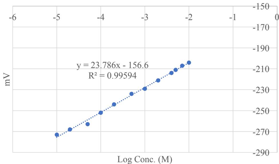
**Figure 120 Initial Calibration curve for lead (taken before 120 minutes reading)**
