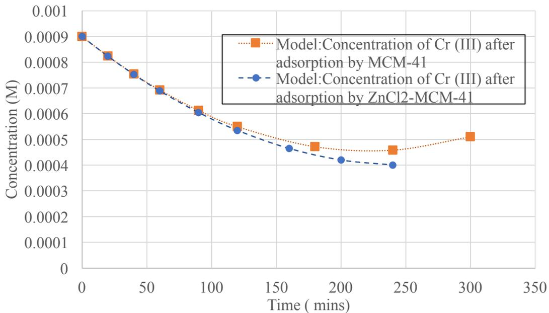
**Figure 63 - Model: Adsorption of 0.001M Cr (III) by MCM-41 & ZnCl<sub>2</sub>-MCM-4**
