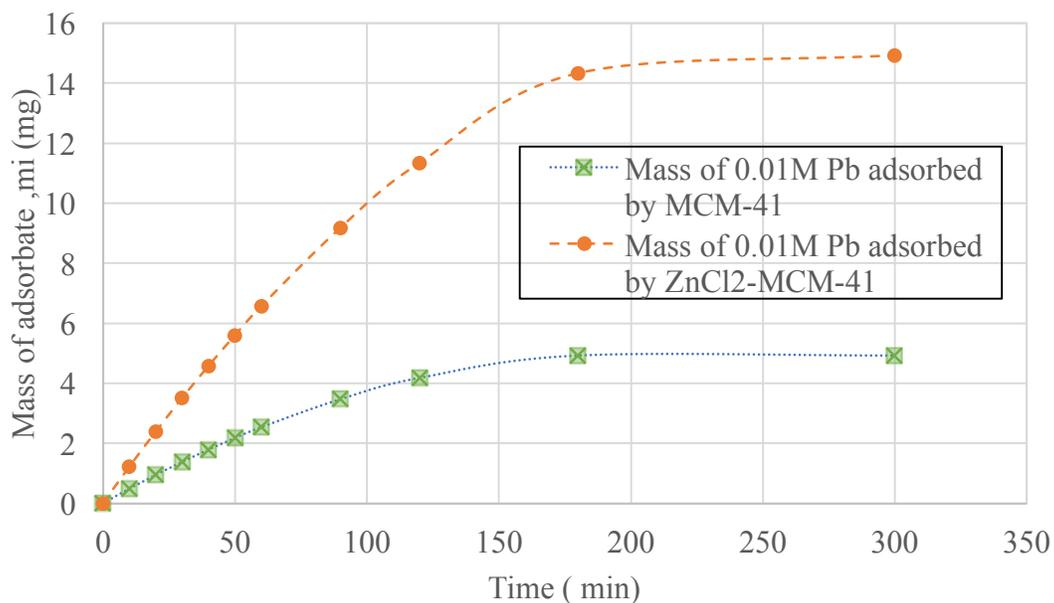
**Figure 37 - Model: Mass of 0.01M Pb (II) adsorbed by MCM-41 & ZnCl<sub>2</sub>-MCM-41**
