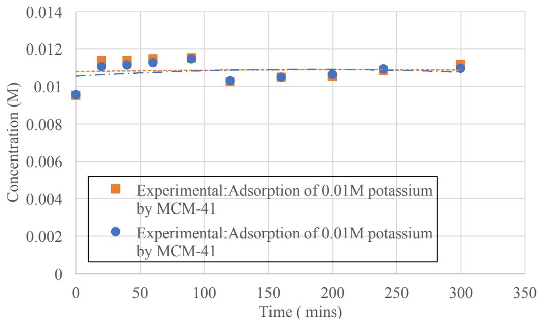
**Figure 92 Experimental: Adsorption of 0.01M K<sup>+</sup> ions by MCM-41 and ZnCl<sub>2</sub>-MCM-41**
