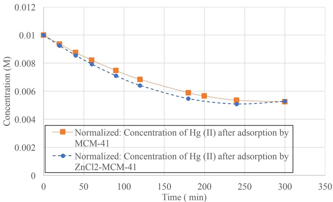
**Figure 48 - Normalized: Adsorption of 0.01M Hg (II) by MCM-41 & ZnCl<sub>2</sub>-MCM-41**
