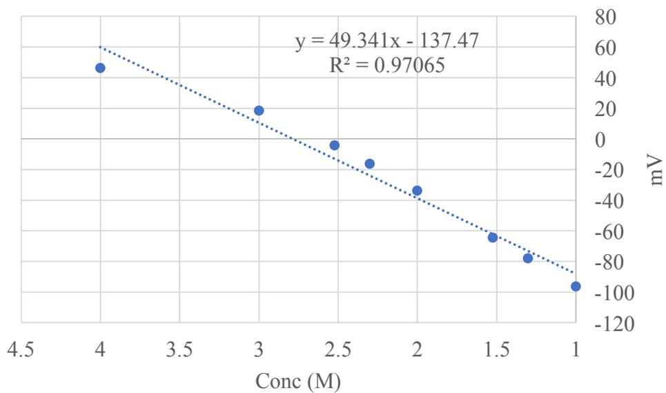
**Figure 141 Initial Calibration curve for nitrate (before taking 24 hours reading for samples with AC)**
