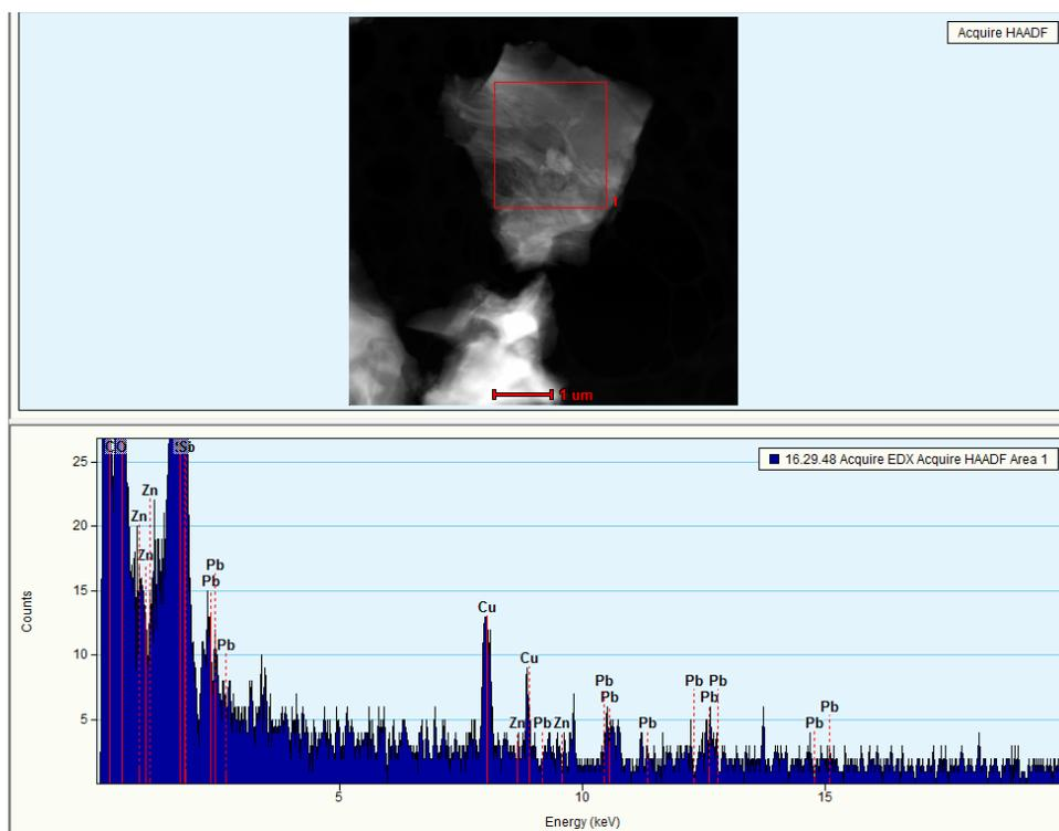
**Figure 24 - STEM Z-contrast image of ZnCl<sub>2</sub>-MCM-41 showing presence of lead**
