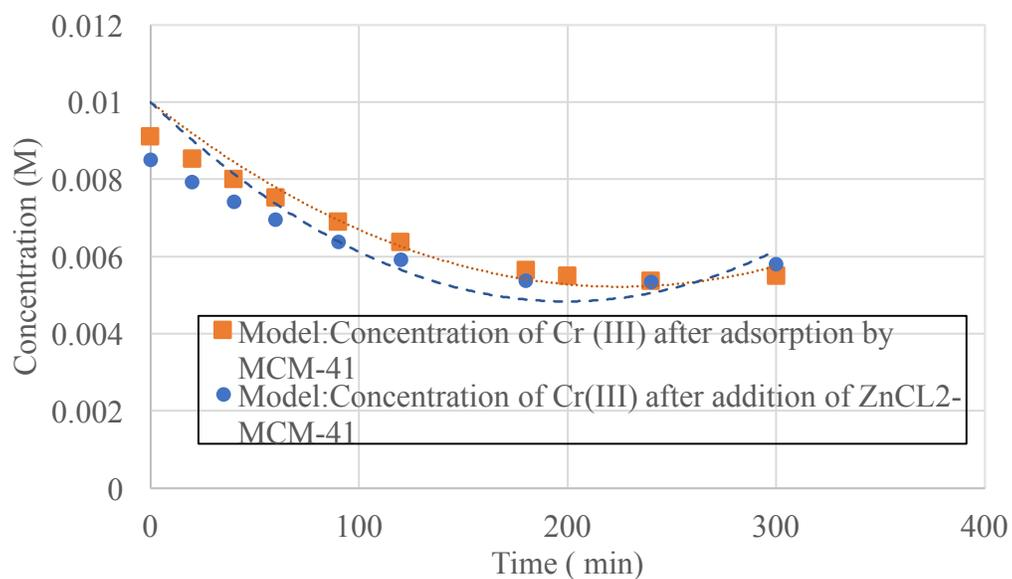
**Figure 59 - Model: Adsorption of 0.01M Cr (III) by MCM-41 & ZnCl<sub>2</sub>-MCM-41**
