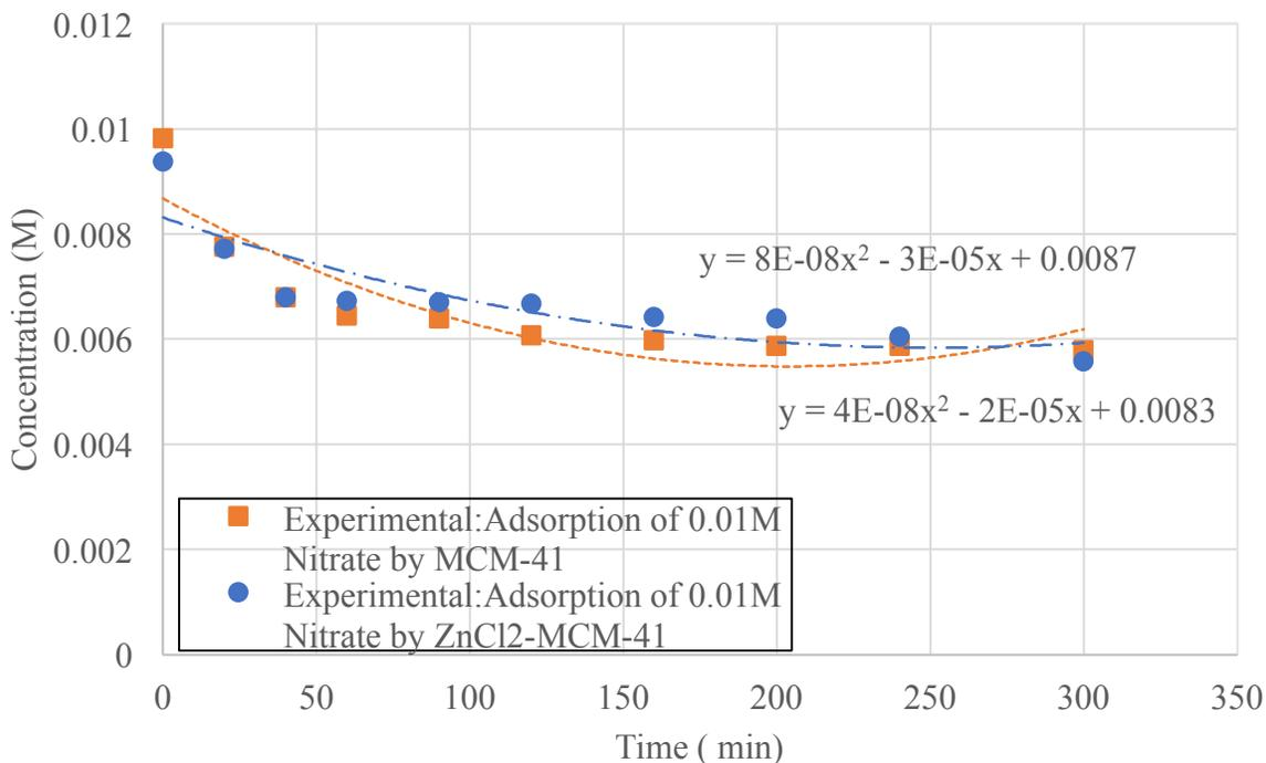
**Figure 103 Experimental: Adsorption of 0.01M NO<sub>3</sub><sup>-</sup> ions by MCM-41 and ZnCl<sub>2</sub>-MCM-41**
