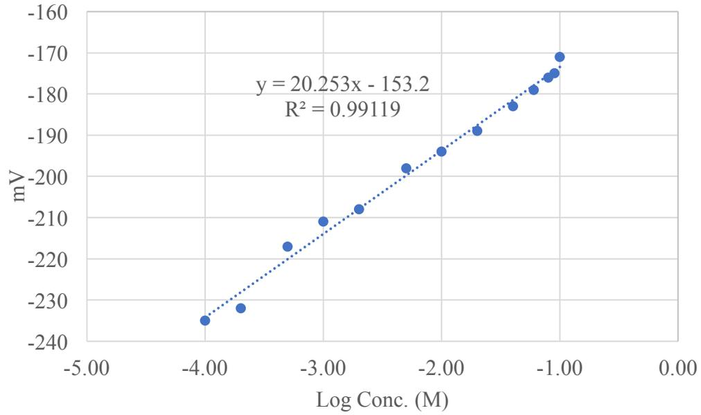
**Figure 129 Initial Calibration curve for lead**
