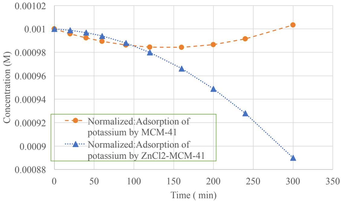
**Figure 90 Normalized: Adsorption of 0.001M K<sup>+</sup> ions by MCM-41 and ZnCl<sub>2</sub>-MCM-41**
