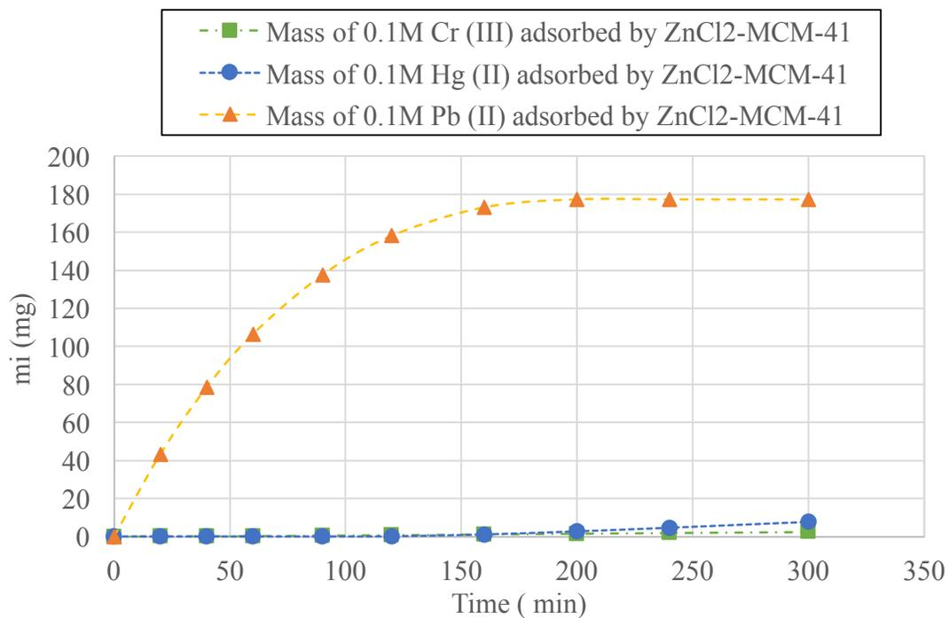
**Figure 73 Model: Mass of the adsorbate (mg) 0.1M heavy metals (Cr<sup>3+</sup>, Hg<sup>2+</sup>, & Pb<sup>2+</sup>) adsorbed by ZnCl<sub>2</sub>-MCM-41**
