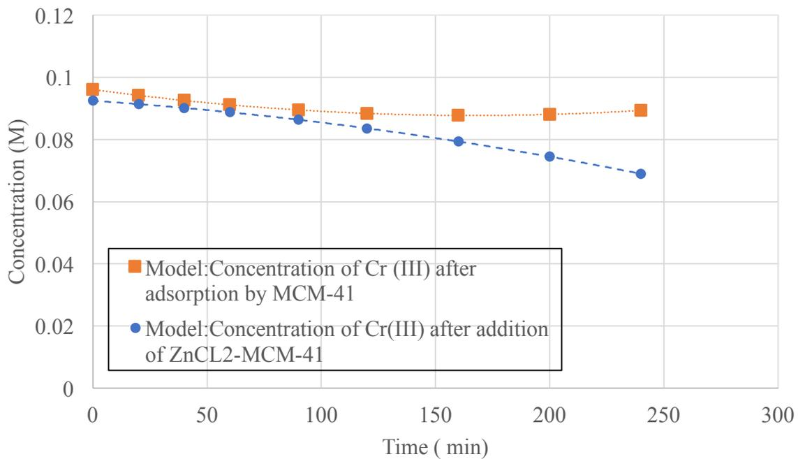
**Figure 55 - Model: Adsorption of 0.1M Cr (III) by MCM-41 & ZnCl<sub>2</sub>-MCM-41**
