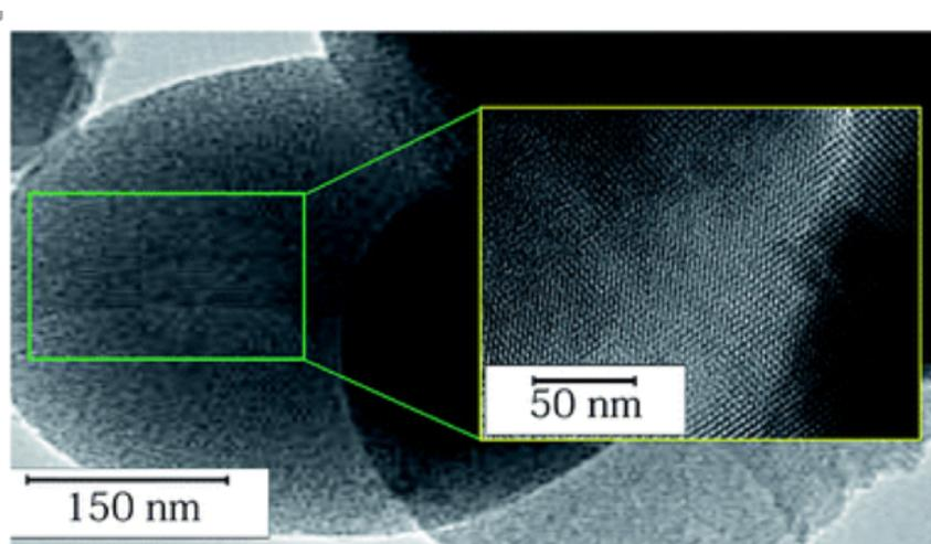
**Figure 7 - TEM image of ZnCl<sub>2</sub>-MCM-41 (Raji et al. 2015)**
