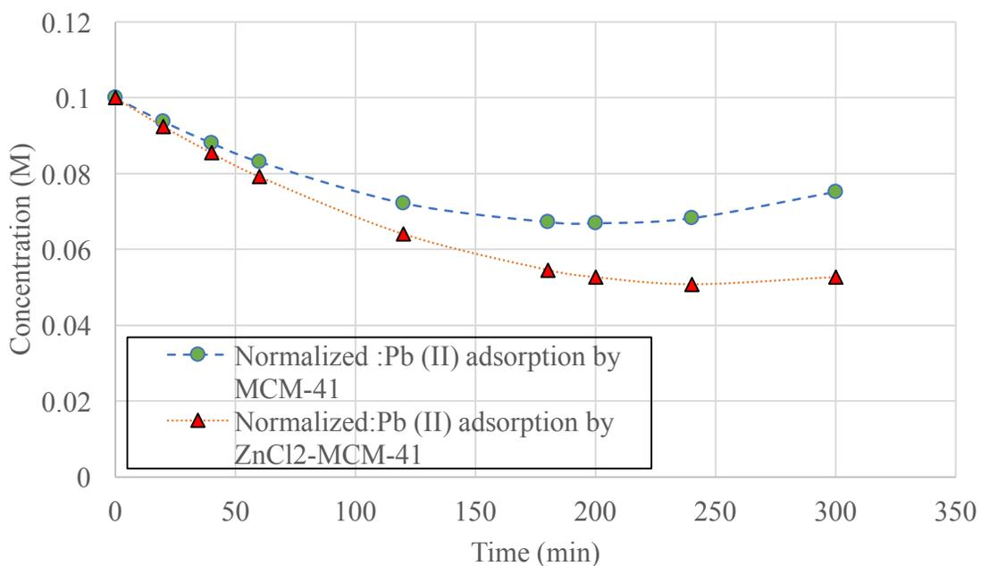
**Figure 32 - Normalized: Adsorption of 0.1M Pb (II) by MCM-41 & ZnCl<sub>2</sub>-MCM-41**
