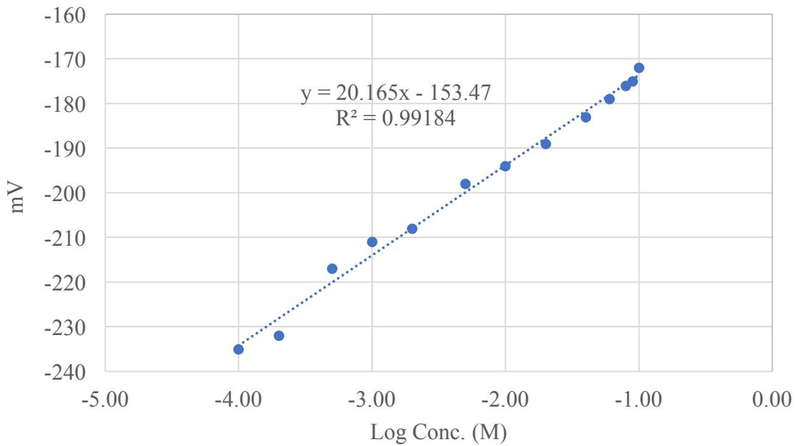
**Figure 124 Calibration curve for lead (before taking 40 minutes reading)**
