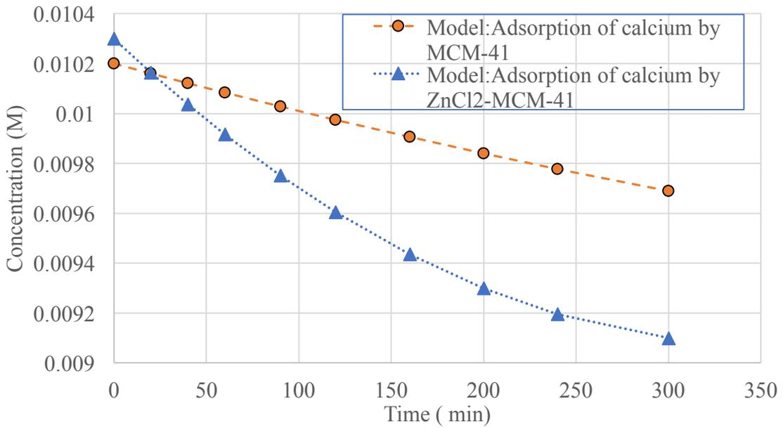
**Figure 80 Model: Adsorption of 0.01M Ca<sup>2+</sup> ions by MCM-41 and ZnCl<sub>2</sub>-MCM-41**
