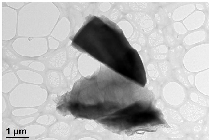
**Figure 16 - TEM image of MCM-41 taken at low magnification (the sample overlays with Lacey Carbon film)**
