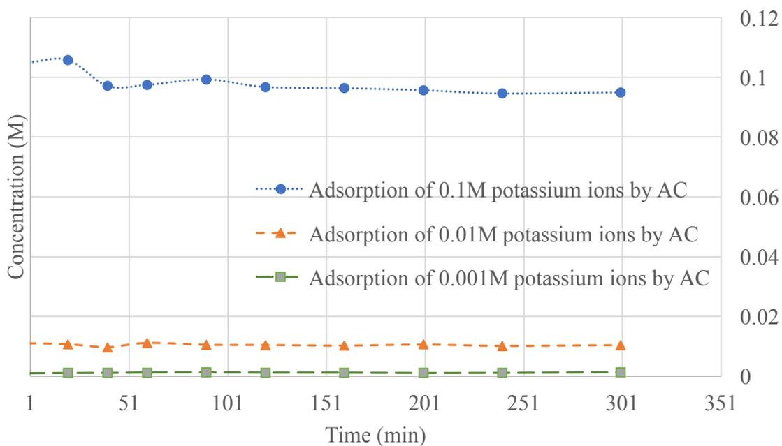
**Figure 113 Adsorption of K<sup>+</sup> ions by AC**
