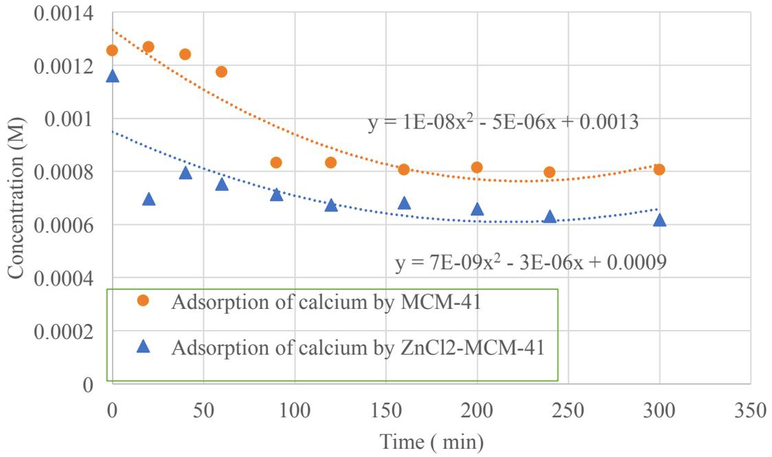
**Figure 75 Experimental: Adsorption of 0.001M Ca<sup>2+</sup> ions by MCM-41 and ZnCl<sub>2</sub>-MCM-41**
