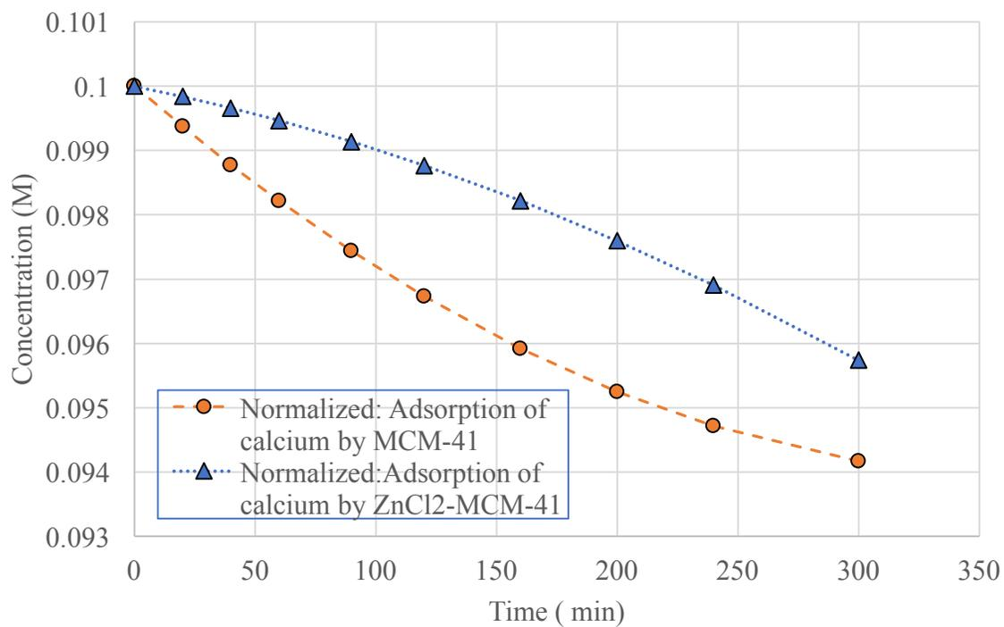
**Figure 85 Normalized: Adsorption of  $0.1\text{M Ca}^{2+}$  ions by MCM-41 and ZnCl<sub>2</sub>-MCM-41**
