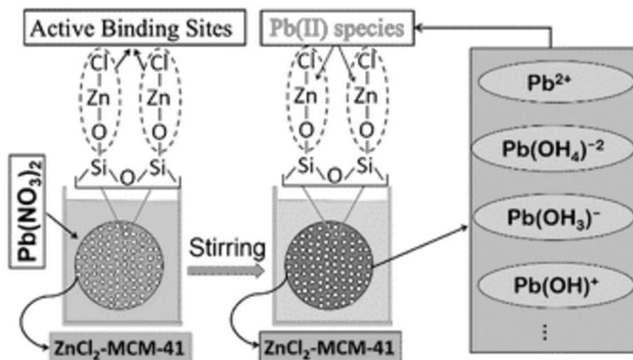
Figure 8 - Adsorption mechanism of Pb (II) species by  $ZnCl_2$ -MCM-41 (Raji et al. 2015)
