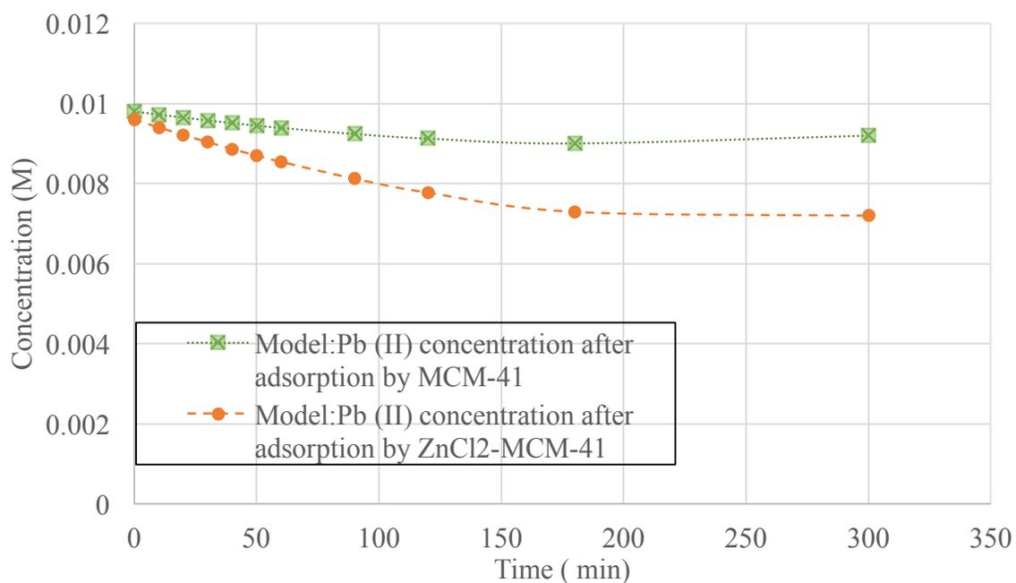
**Figure 35 - Model: Adsorption of 0.01M Pb (II) by MCM-41 & ZnCl<sub>2</sub>-MCM-41**
