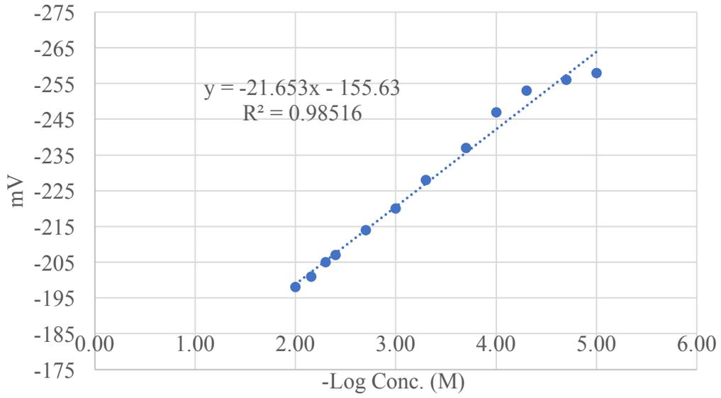
**Figure 116 Initial Calibration curve for lead (taken before taking 2 hours reading)**
