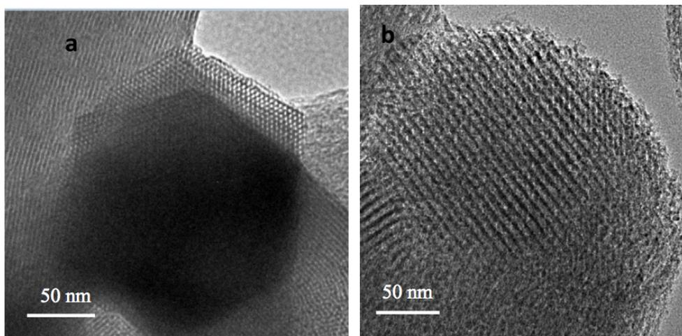
**Figure 4 -a) TEM image of MCM-41 b) TEM image NH<sub>2</sub>-MCM-41 (Bao et al. 2015)**
