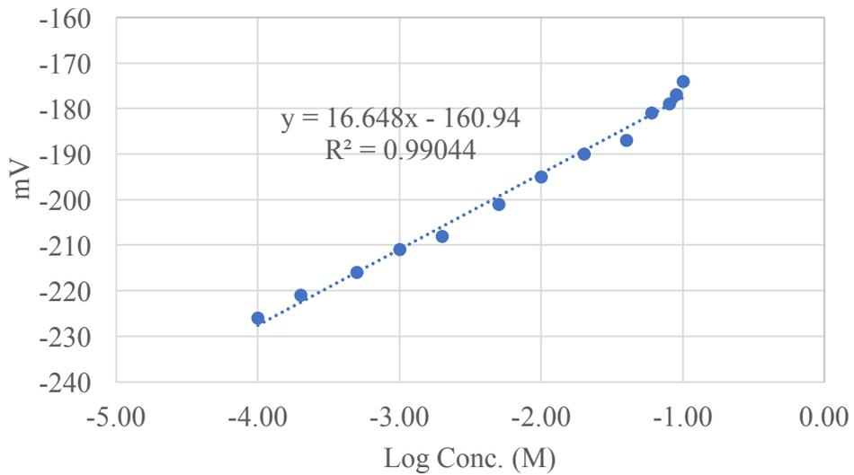
**Figure 132 Calibration curve for lead (taken before 300 minutes reading)**
