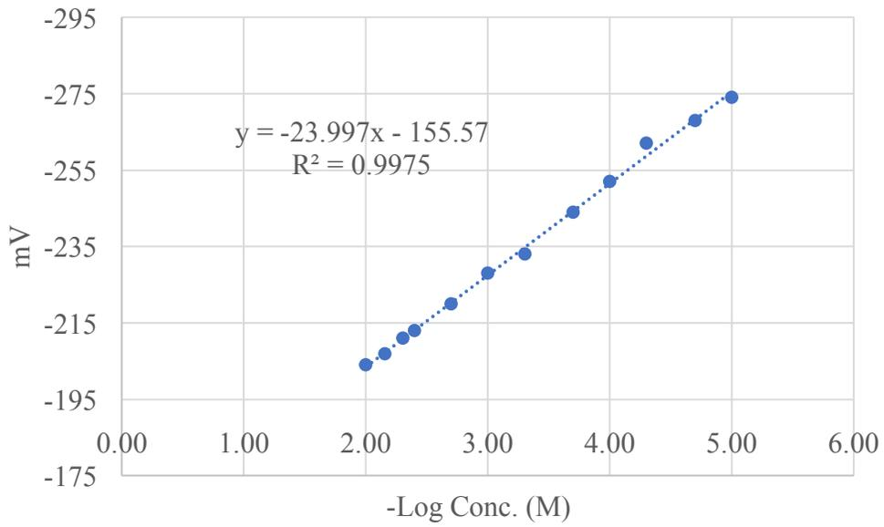
**Figure 117 Initial Calibration curve for lead (taken before taking 24 hours reading)**
