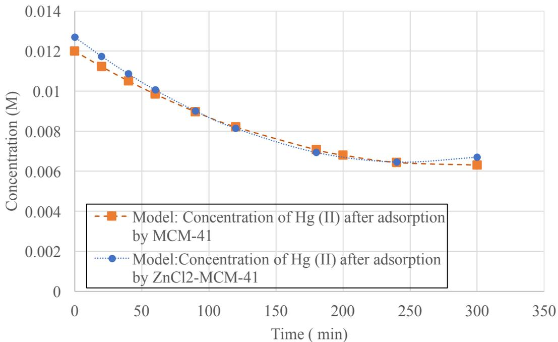
**Figure 47 - Model: Adsorption of 0.01M Hg (II) by MCM-41 & ZnCl<sub>2</sub>-MCM-41**
