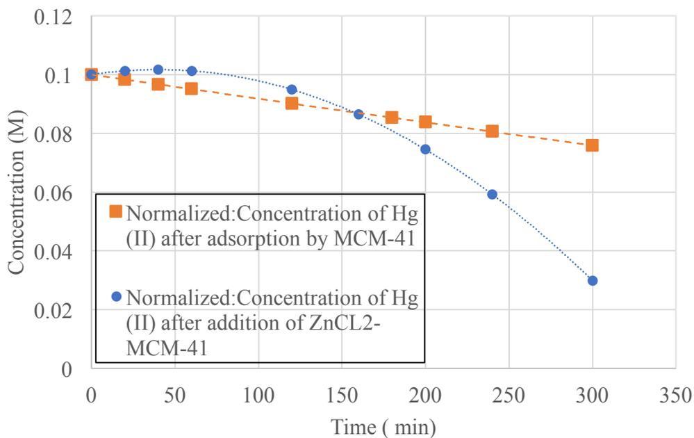
**Figure 44 - Normalized: Adsorption of 0.1M Hg (II) by MCM-41 & ZnCl<sub>2</sub>-MCM-41**
