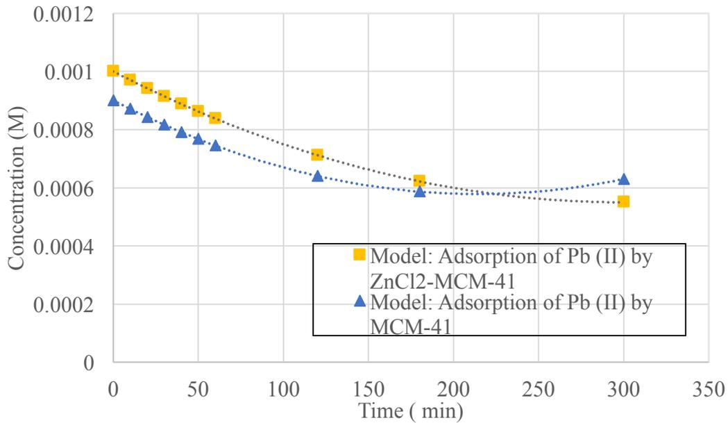
**Figure 39 - Model: Mass of 0.001M Pb (II) adsorbed by MCM-41 & ZnCl<sub>2</sub>-MCM-41**
