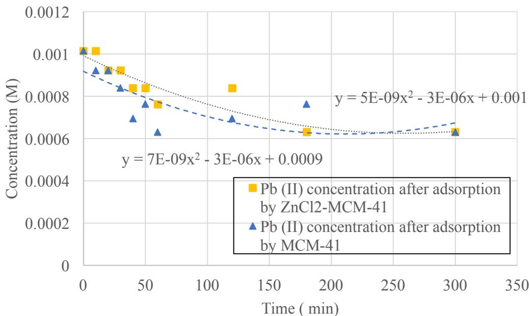
**Figure 38 - Model: Mass of 0.001M Pb (II) adsorbed by MCM-41 & ZnCl<sub>2</sub>-MCM-41**
