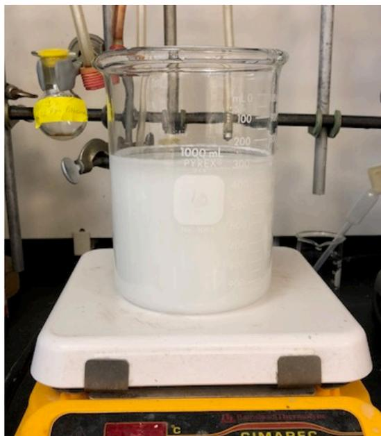
**Figure 11 – Synthesis of MCM-41 (Solution with CTAB, TMAOH, and TEOS after stirred together for 4 hours)**
