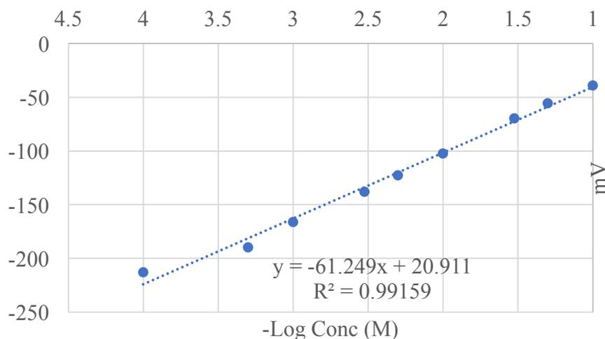
**Figure 87 Initial Calibration Curve for K<sup>+</sup> electrode**
