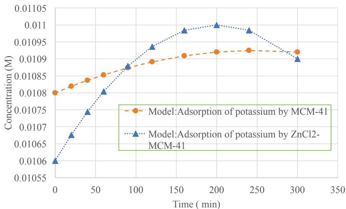
**Figure 93 Model: Adsorption of 0.01M K<sup>+</sup> ions by MCM-41 and ZnCl<sub>2</sub>-MCM-41**
