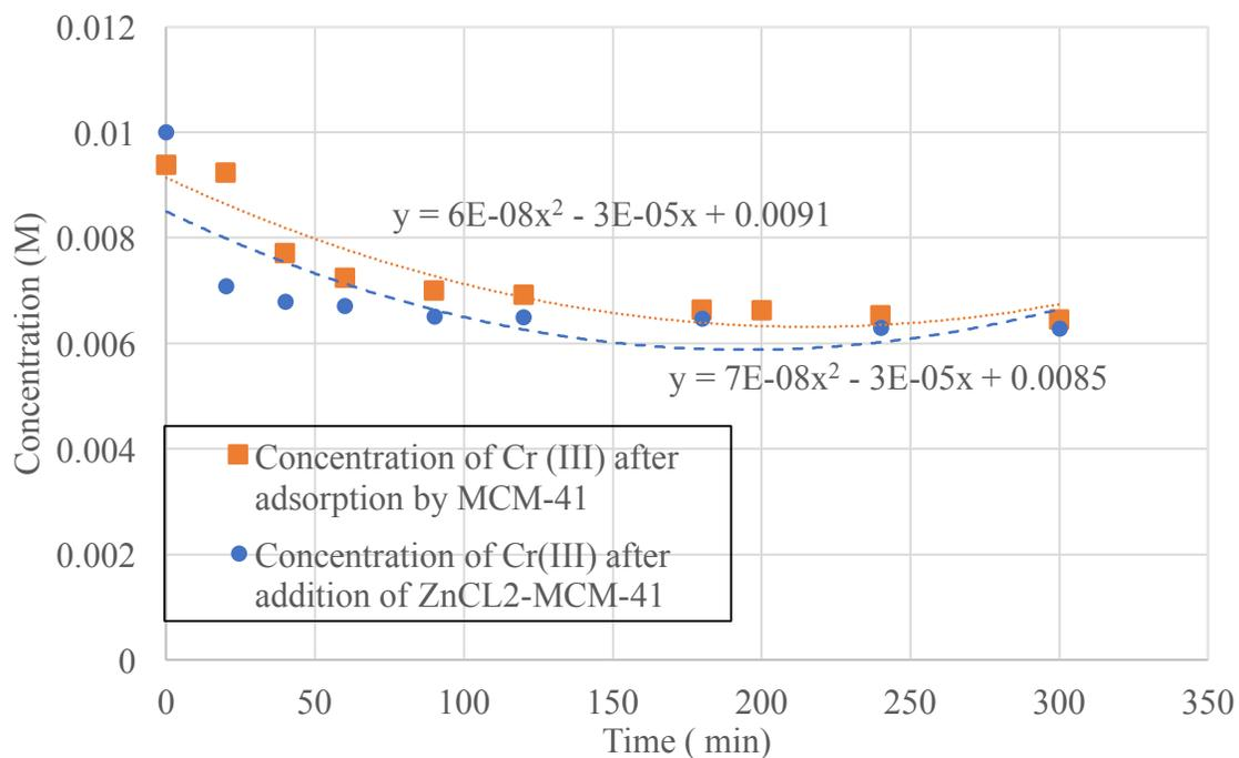
**Figure 58 - Experimental: Adsorption of 0.01M Cr (III) by MCM-41 & ZnCl<sub>2</sub>-MCM-41**
