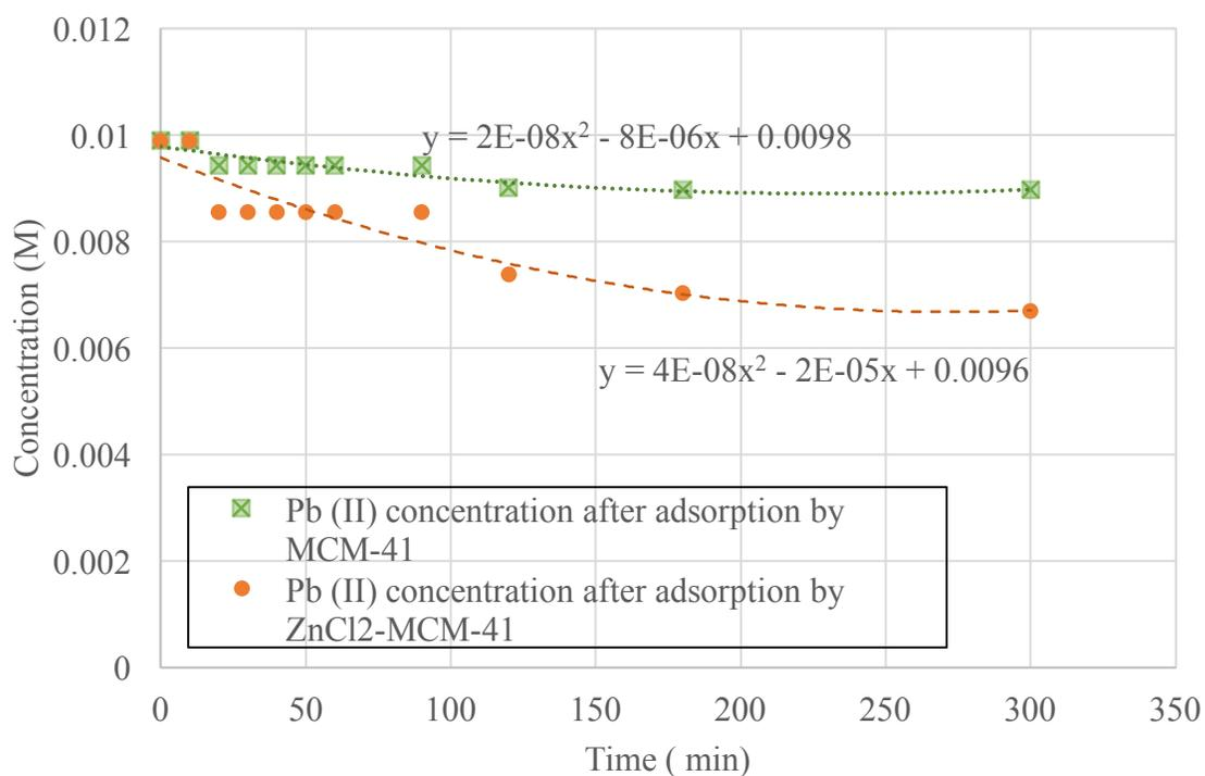
**Figure 34 - Experimental: Adsorption of 0.01M Pb (II) by MCM-41 & ZnCl<sub>2</sub>-MCM-41**
