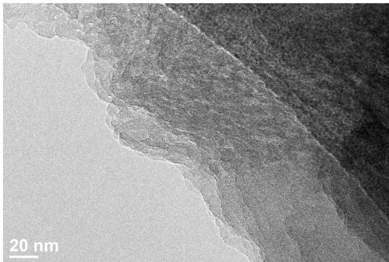
**Figure 18 - TEM image of MCM-41 taken at higher magnification (20 nm), showing the morphologies in the sample**
