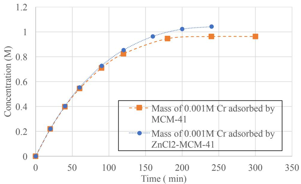
**Figure 65 - Model: Mass of 0.001M Cr (III) adsorbed by MCM-41 & ZnCl<sub>2</sub>-MCM-41**
