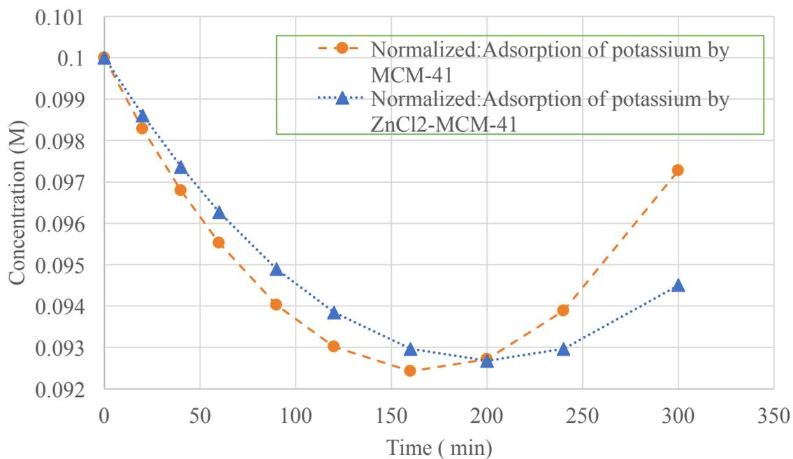
**Figure 98 Normalized: Adsorption of 0.1M K<sup>+</sup> ions by MCM-41 and ZnCl<sub>2</sub>-MCM-41**
