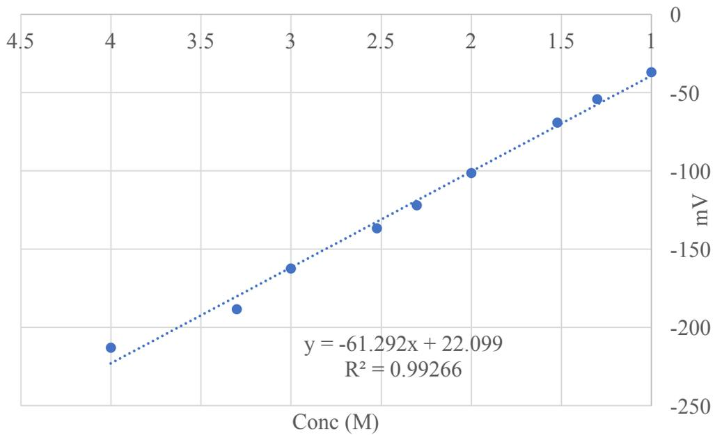
**Figure 137 Calibration curve for potassium (for taking 5 hours reading)**
