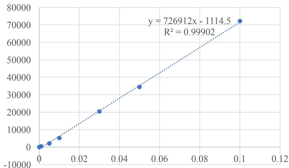
Figure 144 Calibration curve for Cr (with wavelength 267.716)
