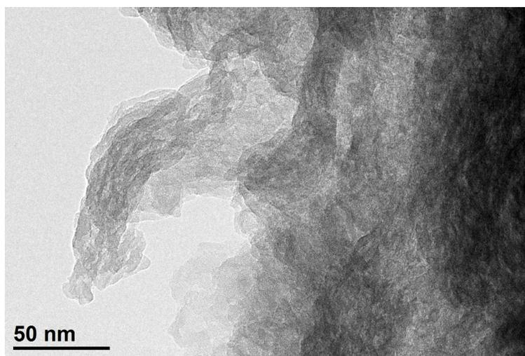
**Figure 20 - TEM image of ZnCl<sub>2</sub>-MCM-41, taken at higher magnification (50nm), showing the morphologies in the sample**
