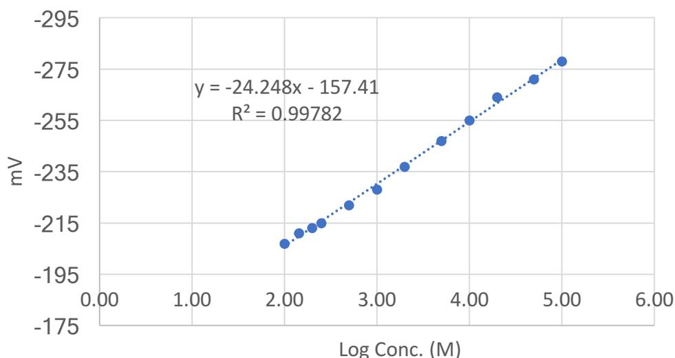
**Figure 29 – Initial Calibration Curve for Lead**
