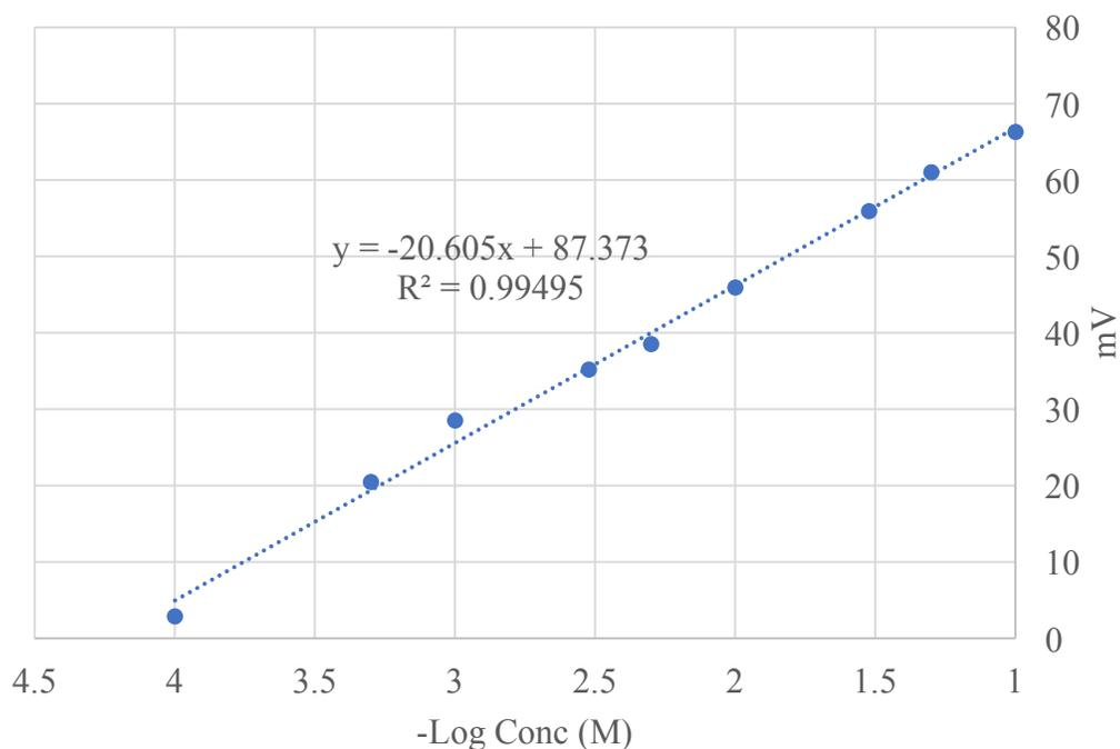
**Figure 134 Calibration curve for calcium (for 24 hours)**
