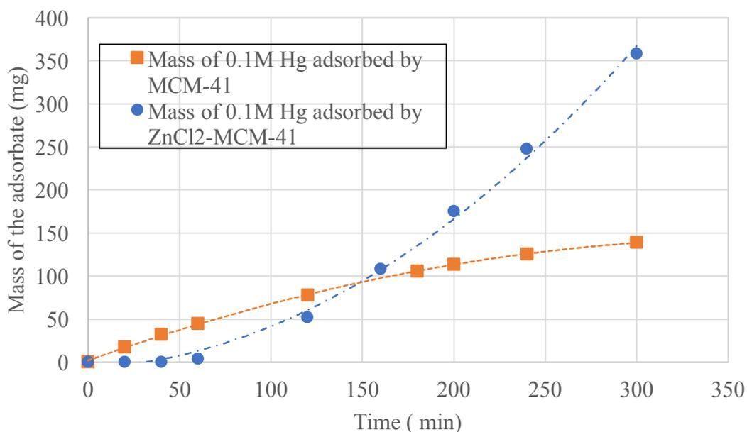
**Figure 45 - Model: Mass of 0.1M Hg (II) adsorbed by MCM-41 & ZnCl<sub>2</sub>-MCM-41**
