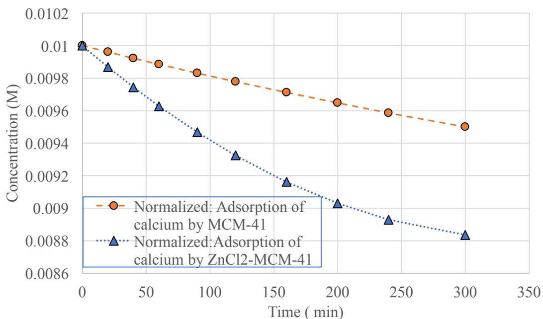
**Figure 81 Normalized: Adsorption of 0.01M Ca<sup>2+</sup> ions by MCM-41 and ZnCl<sub>2</sub>-MCM-41**
