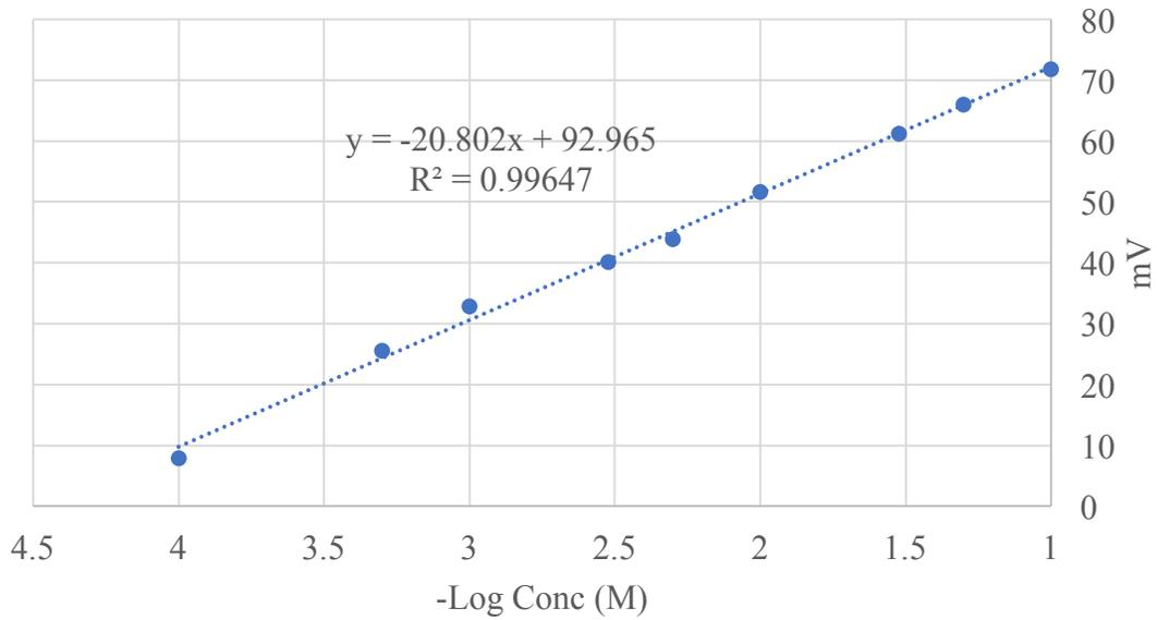
**Figure 133 Initial Calibration curve for calcium**
