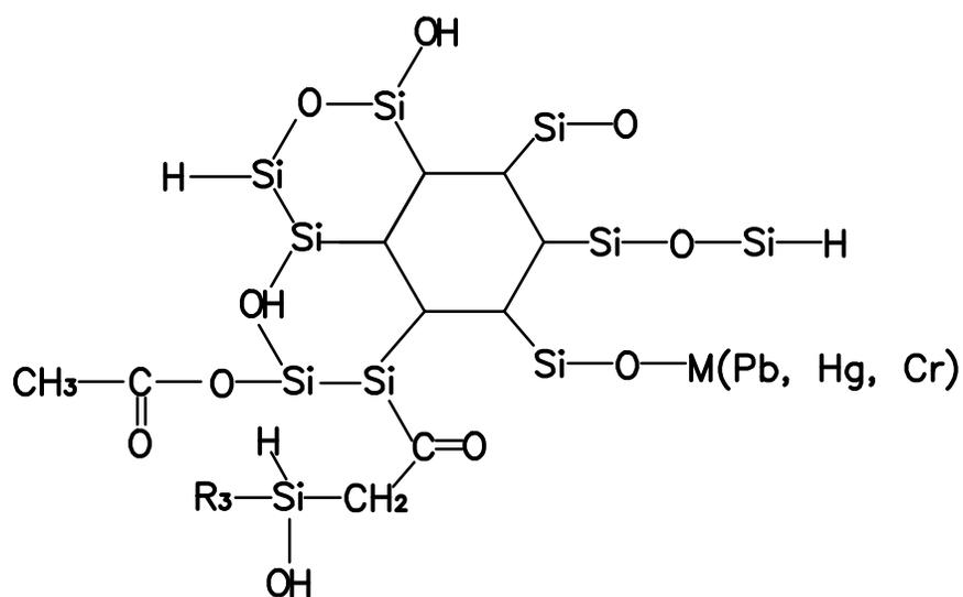
Figure 27 MCM-41 structure after adsorption of heavy metals
