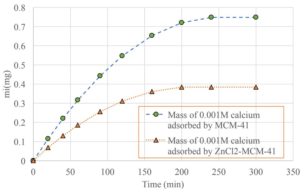
**Figure 78 Mass of 0.001  $Ca^{2+}$  ions adsorbed by MCM-41 and ZnCl<sub>2</sub>-MCM-41**
