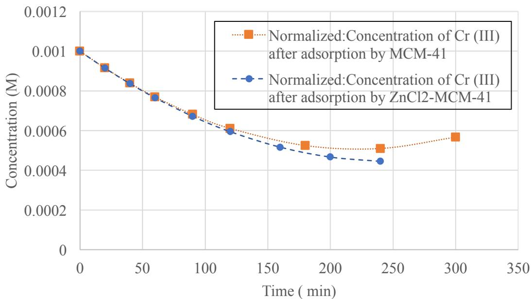
**Figure 64 - Normalized: Adsorption of 0.001M Cr (III) by MCM-41 & ZnCl<sub>2</sub>-MCM-41**
