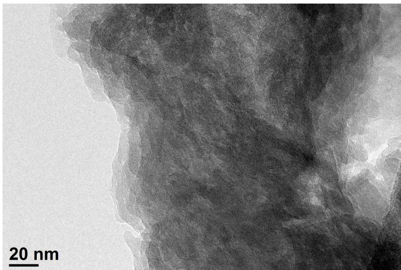
Figure 21 - TEM image of ZnCl<sub>2</sub>-MCM-41, taken at higher magnification (20nm), showing the morphologies in the sample
