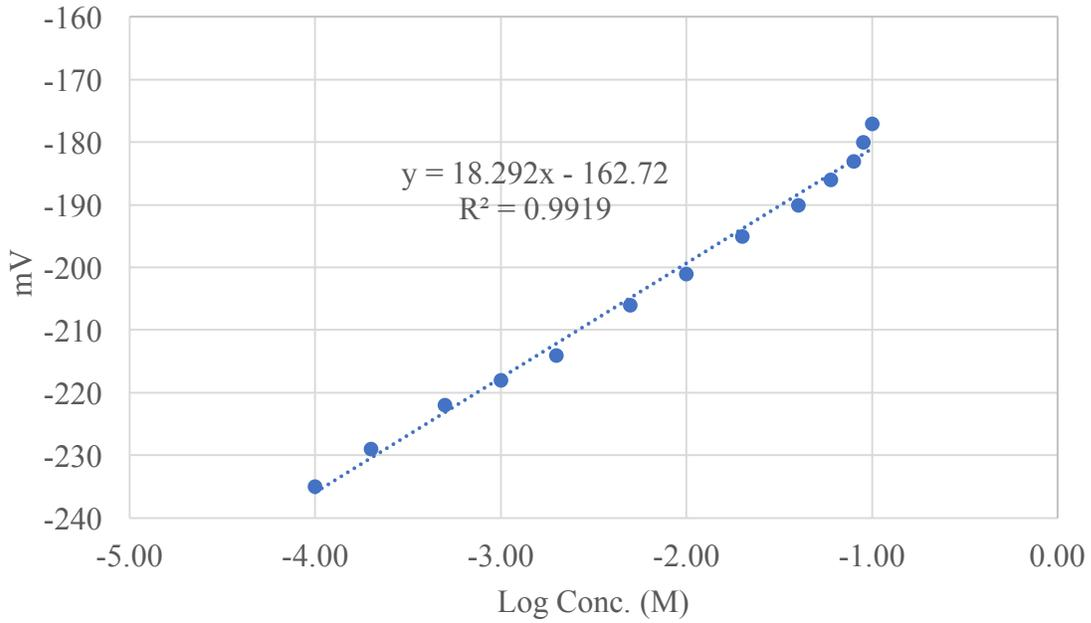
**Figure 123 Initial Calibration curve for lead**
