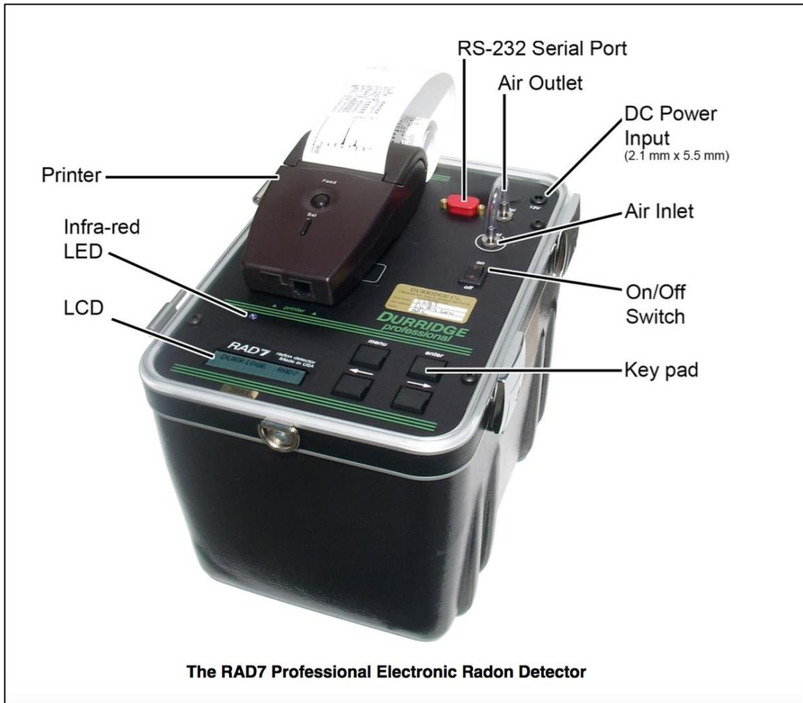
Figure 3.1: RAD7 Professional Electronic Radon Detector
