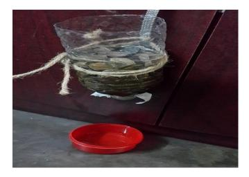
Figure 24. Filtration in Sand-Stone Turbidity Filter
