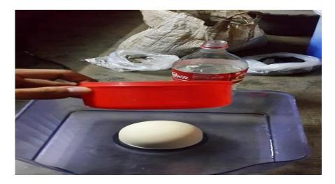
Figure 25. Filtration Using Ceramic Filter
