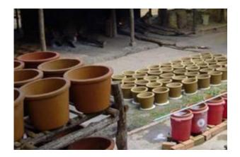
Figure 7. Clay Water Filter (Engineering for Change, 2012)
