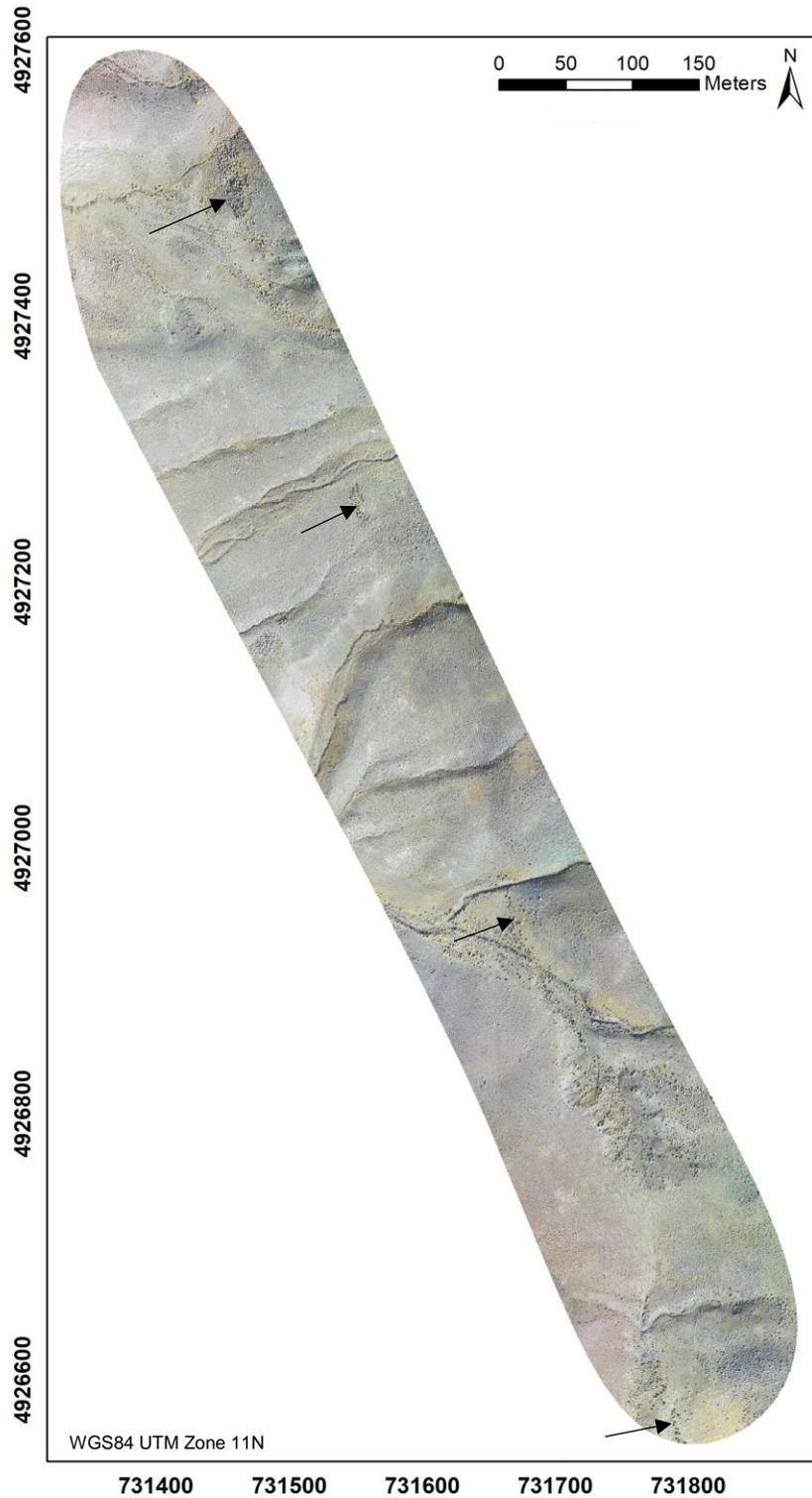
**Figure 37:** The orthophoto produced using Pix4Dmapper 4.0, from the UAS data collection. The arrows point to locations where linear vegetation patterns were observed.
