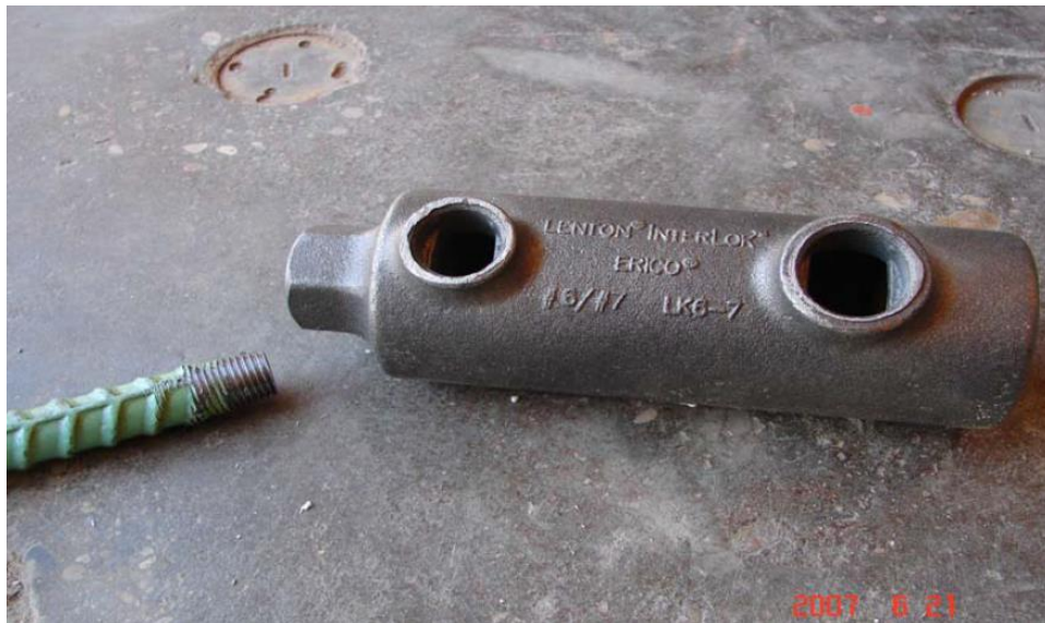
Figure 2-1. Lenton Interlok for No. 6 steel reinforcing bar (Jansson 2008)
