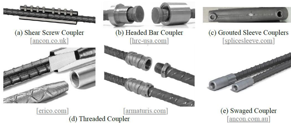
Figure 2-28. Mechanical reinforcing bar couplers (Tazarv and Saiidi, 2015)
