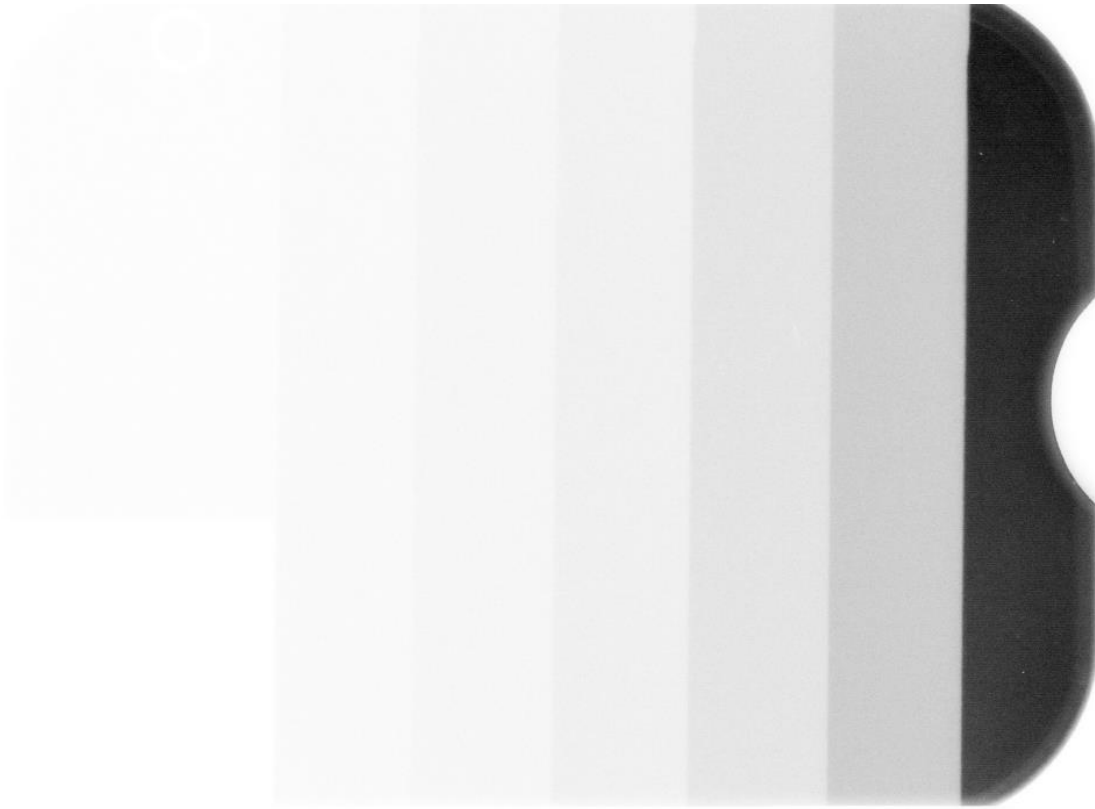
Figure 6.3-1. Al step-wedge image from 2x30- \mu\text{m} W x pinch.
