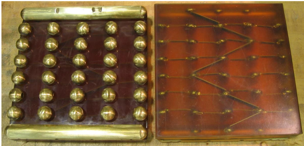
Figure 3.1-2. The LTD/NRL brick switch.
