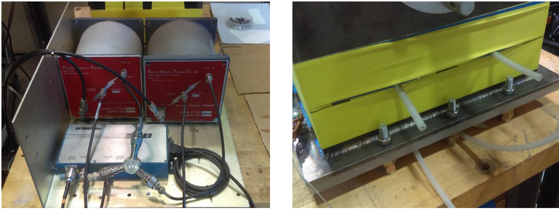
Figure 4.1-4. An x-pinch driver trigger system: trigger box (left); end of the through-housing trigger-line (right).
