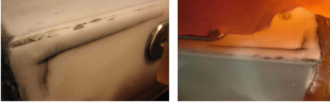
Figure 4.1-7. Cracks in a brick's capacitor: front crack (left), top crack (right).
