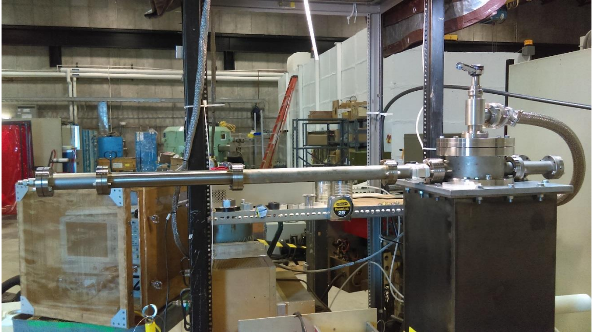
Figure I-2. Vacuum chamber with two output ports.
