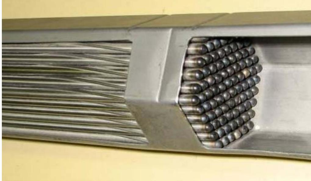
Figure 2. EBR-II Element Bundle with Wire Wraps<sup>(9)</sup>.
