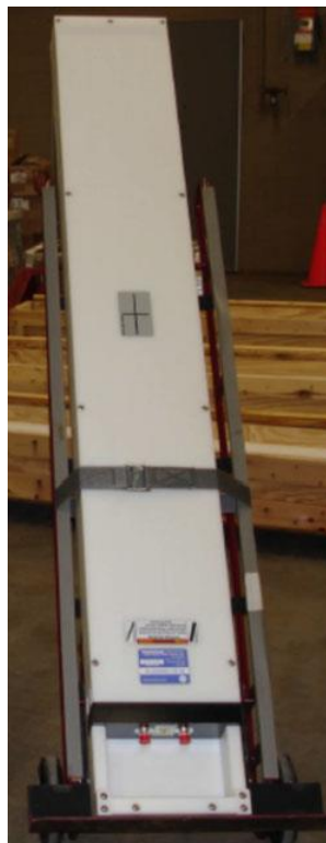
Figure 2.10 GE Reuter Stokes NDM panel containing an array of boron-lined proportional counters [22].
