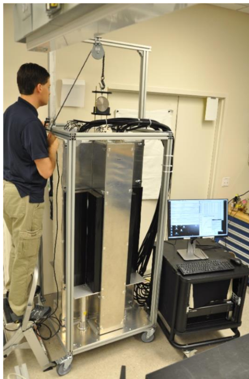
Figure 6.3 Photograph of the completed LiNMC and associated DAQ. A sample is on the sample holder and ready to be lowered into the sample chamber.
