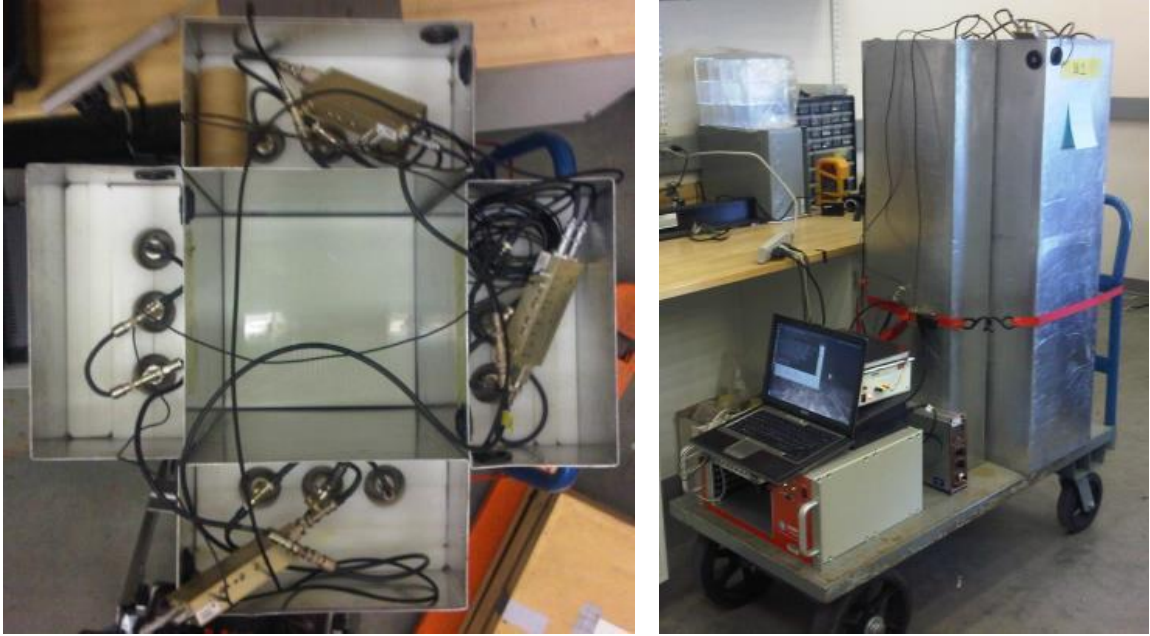
Figure 5.1 (Left) top view and (right) side view of the NCC12 multiplicity counter (set up for an unrelated polyethylene experiment) [49].
