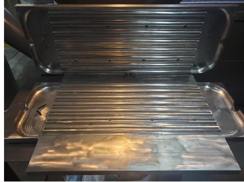
(b) Bottom volume of the circular flow path HX shown before welding. The bottom plate (top) and center plate (bottom) are shown here.
