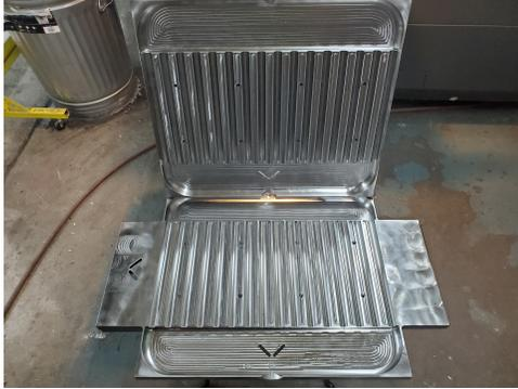
(a) Top volume of the circular flow path HX shown before welding. The top plate (top) and center plate (bottom) are shown here.
