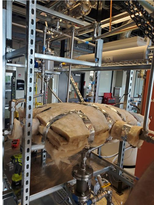
(b) A test section shown installed and insulated with two sheets of fiberglass insulation top and bottom.
