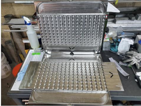
(a) Top volume of the oval twisted flow path HX shown before welding. The top plate (top) and center plate (bottom) are shown here.
