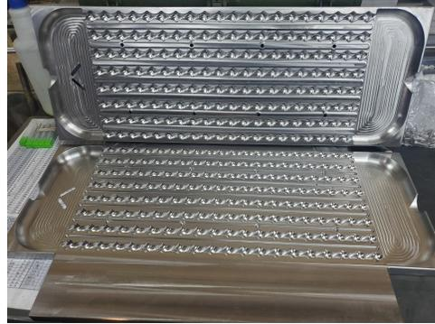
(b) Bottom volume of the oval twisted flow path HX shown before welding. The bottom plate (top) and center plate (bottom) are shown here.
