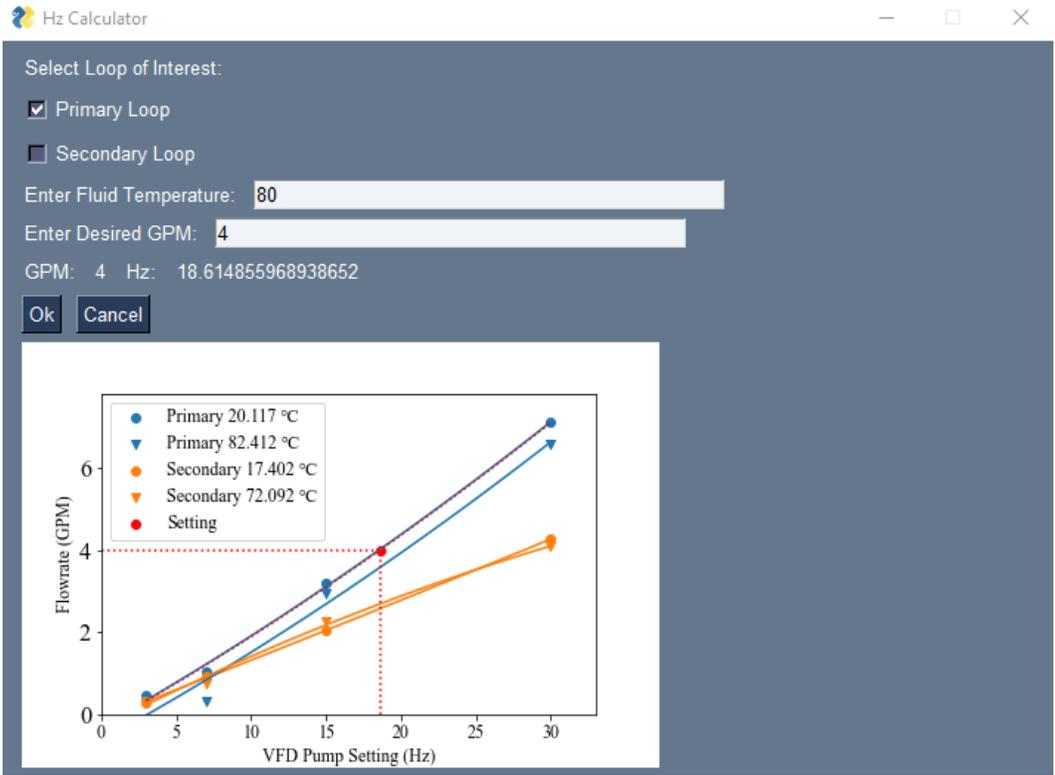
Figure 43: The calibration curves for the primary and secondary loops at 20 and 80 °C with the oval twisted heat exchanger installed.
