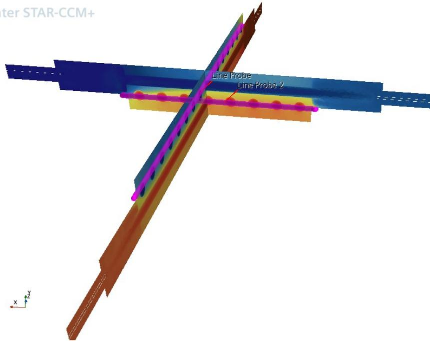
Figure 16: An isometric view indicating where the temperature profiles are collected for the hot and cold sides of the HX.
