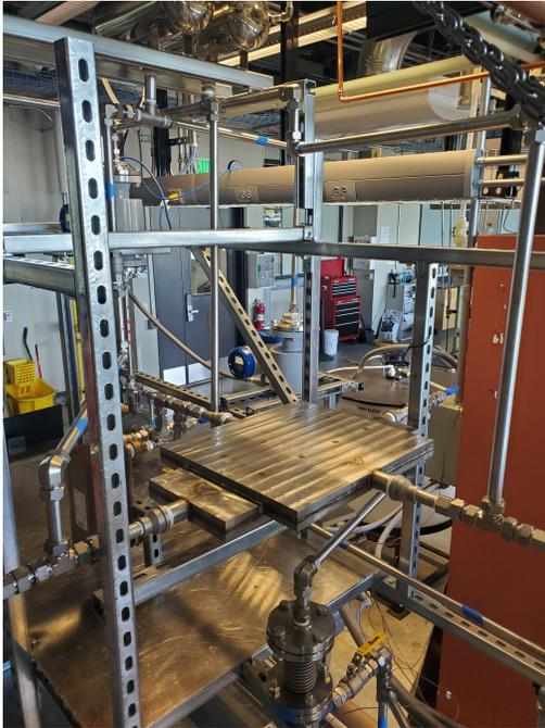
(a) A test section shown installed and uninsulated.
