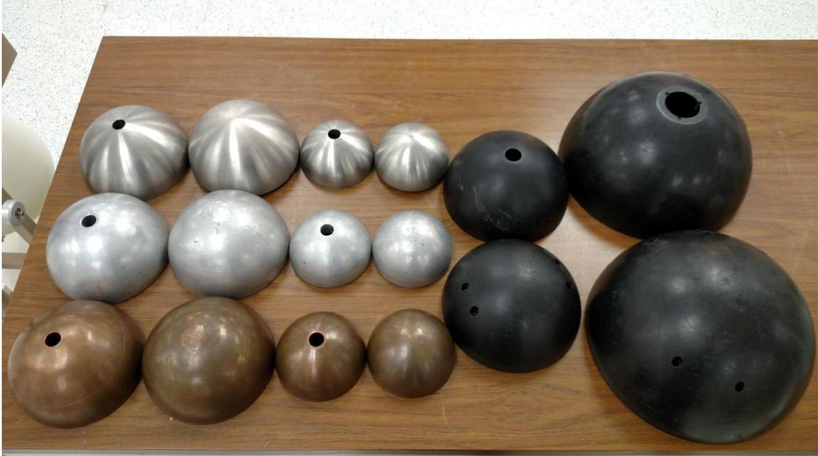
Figure 10: BSE hemispheres: copper (bottom), lead (middle), tungsten (top), HDPE covers (right)
