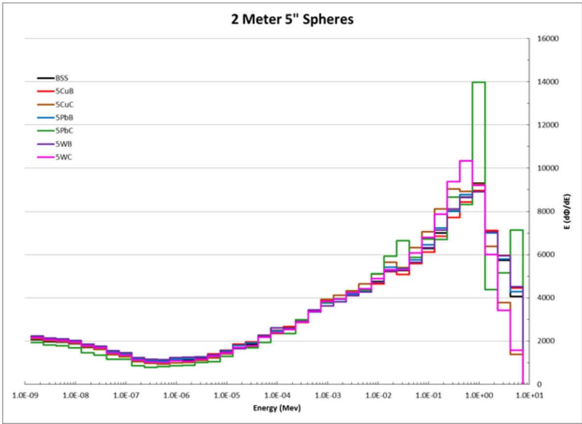
Figure 27: Unfolded spectra for all 5" BSE spheres at the 2 meter location
