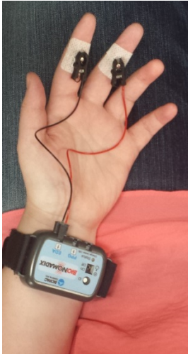
Figure A1: Representation of Skin Conductance Electrode Placement
