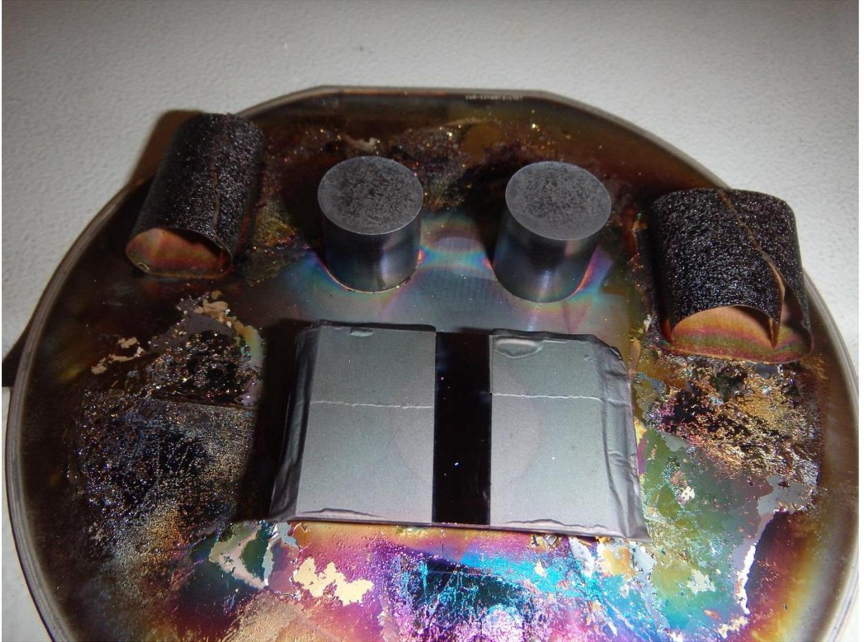
Figure 4.4 Completed samples coated with SiC
