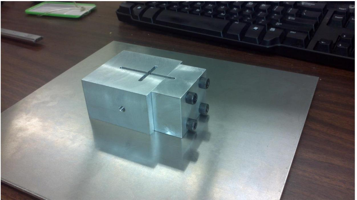
Figure 4.1 Aluminum jig used for holding graphite cylinder sample for hydraulic and laser cutting.
