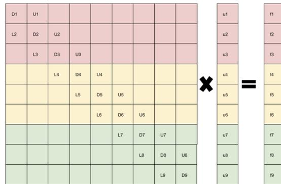
Figure 6.3: Distributed matrix-vector multiplication over three processors
