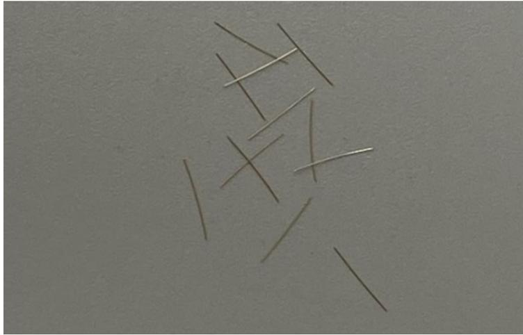
*Figure 13 - Stainless steel fibers*
