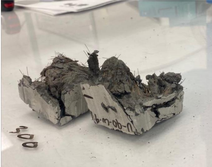
Figure 30 - An explosively spalled UHPC sample
