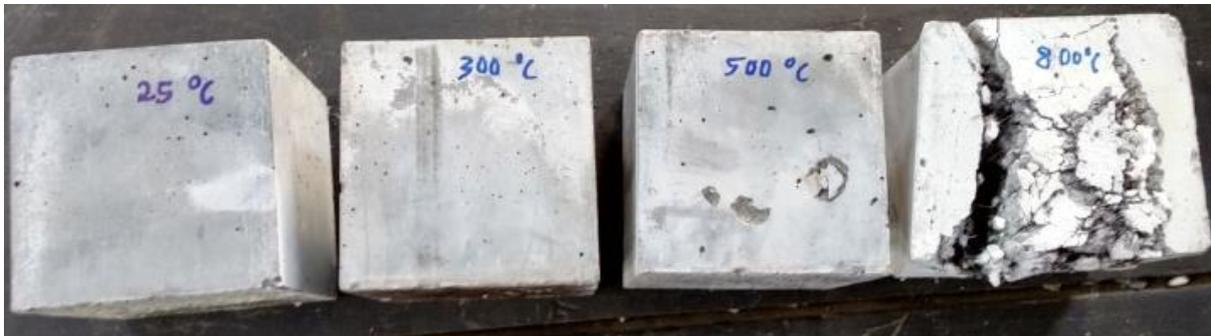
Figure 11 - Spalled UHPC sample from Raizal S.M. Rashid's work
