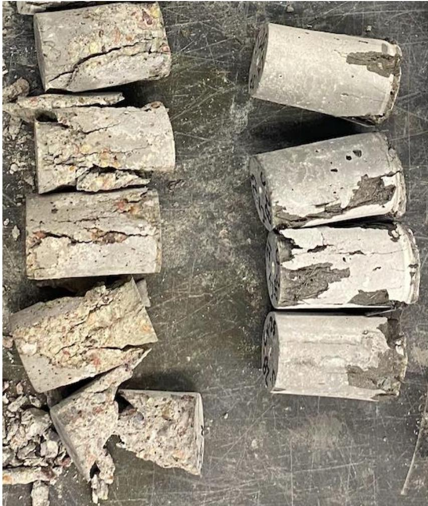
*Figure 29 - Cylindrical samples after compression testing*
