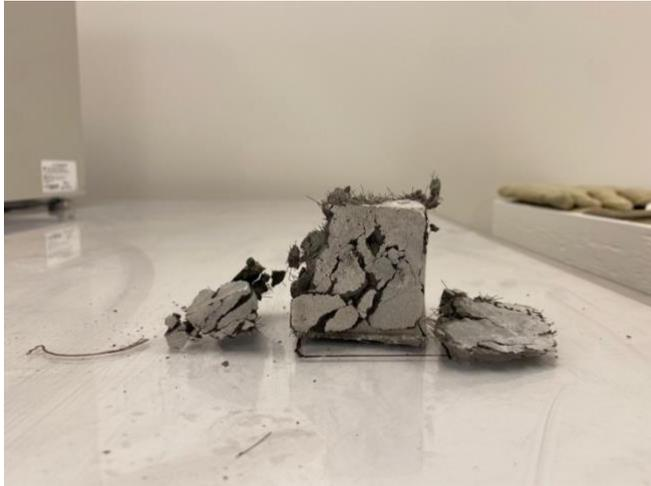
*Figure 10 - Spalled UHPC sample from this research*
