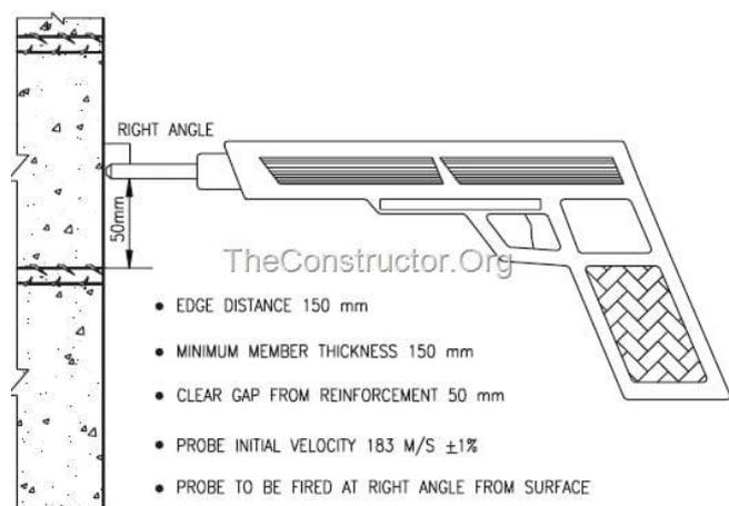
Figure 6 - Diagram of penetration testing equipment
