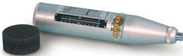
Figure 5 - A rebound hammer used to test for concrete hardness
