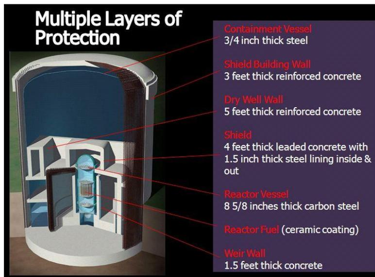
Figure 1 - Diagram of common materials in a reactor containment building
