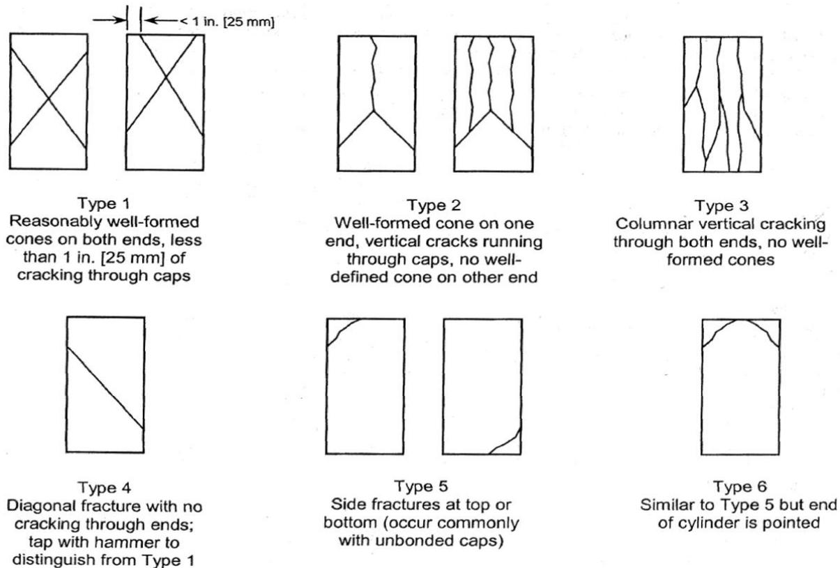
Figure 22 - ASTM fracture types
