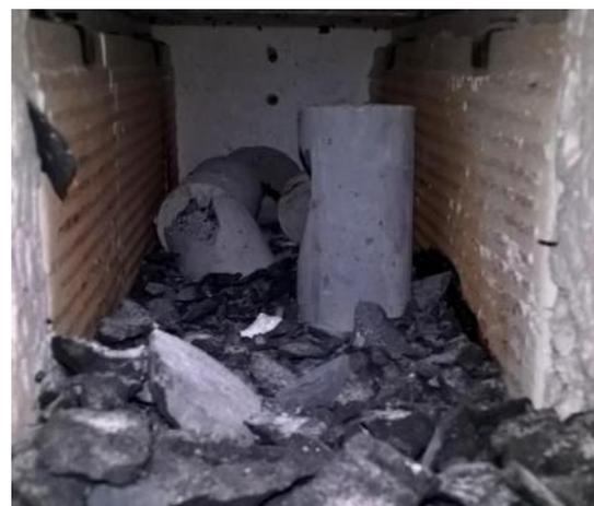
*Figure 9 - Spalled UHPC sample from Jamshaid Sawab's research*
