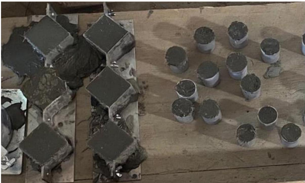
*Figure 14 - UHPC in sample molds*
