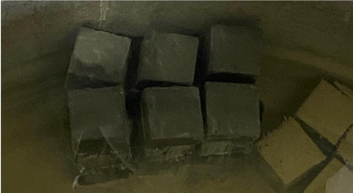
*Figure 15 - UHPC samples in water bath*
