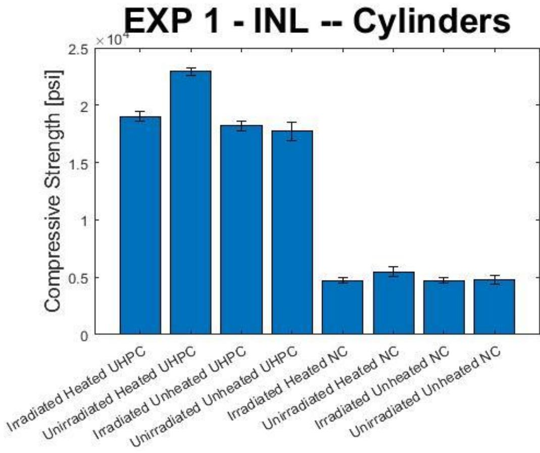
Figure 24 - EXP 1 - INL results for cylinder samples
