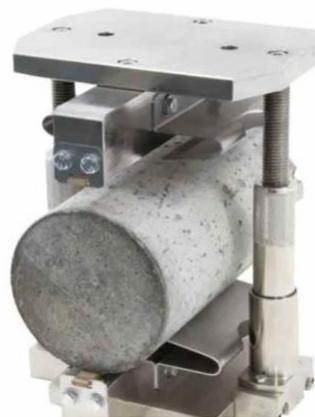
Figure 8 - Split tension test
