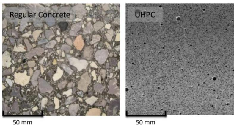
Figure 3 - Comparison of normal concrete and UHPC grain structures
