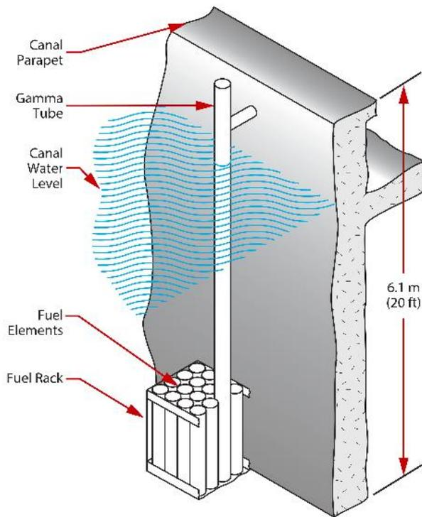
*The ATR Gamma Facility enables irradiation of experiments up to  $5 \times 10^6$  R/hr.*
