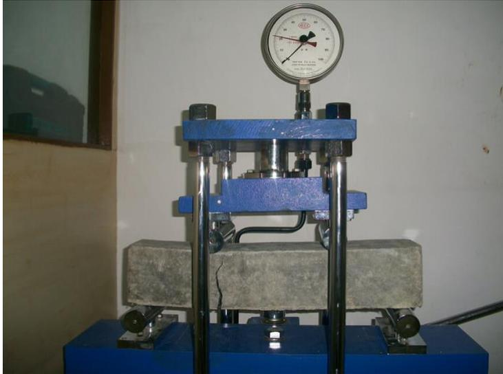
Figure 7 - Flexure strength test
