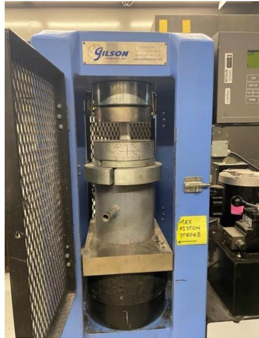
Figure 4 - Sample being compression tested
