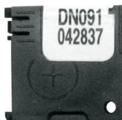
Figure 3.15: Image of a nanoDot used in the dosimetry measurements. Notice the top row alpha numeric sequence; the DN091 stands for a sensitivity correction of 0.91
