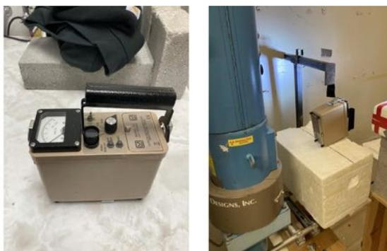
Figure B.3: left) is an image of the Ludlum model 9-4 ion-chamber right) Image of the the experimental set up. The Ludlum detector sits window side facing the source window, on top of a Styrofoam block attached to a sliding platform connected to the rotary stage at the bottom.
