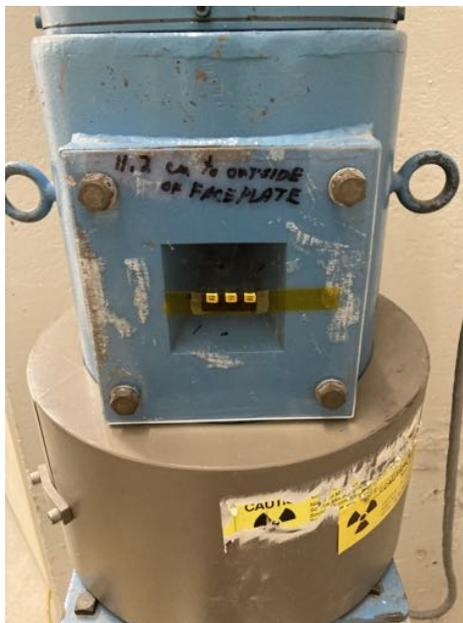
Figure B.7: An array of OSLs taped to the cesium source window 11.2 cm from the source.
