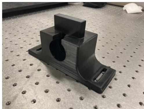
(b) Sleeve inserted into the stand
