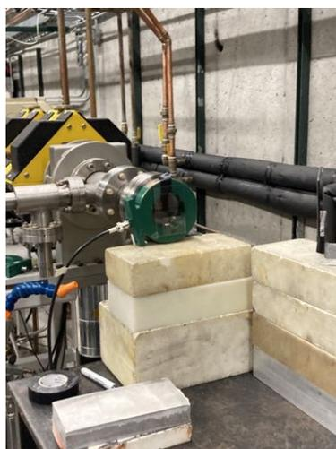
(a) Pearson coil in front of the  $0^\circ$  beam pipe window
