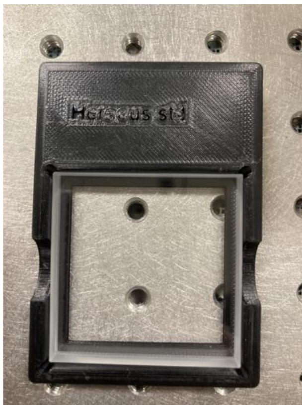
Figure 2.7: HPFS sample inside a custom holder designed for our radiation hardness tests.
