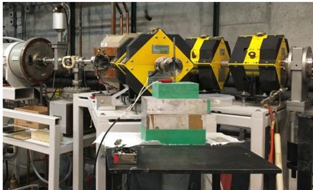
Figure 3.18: The 45°Port. A tungsten rod (oriented vertically) located at beamport exit window measures the current for the beam energy scan.
