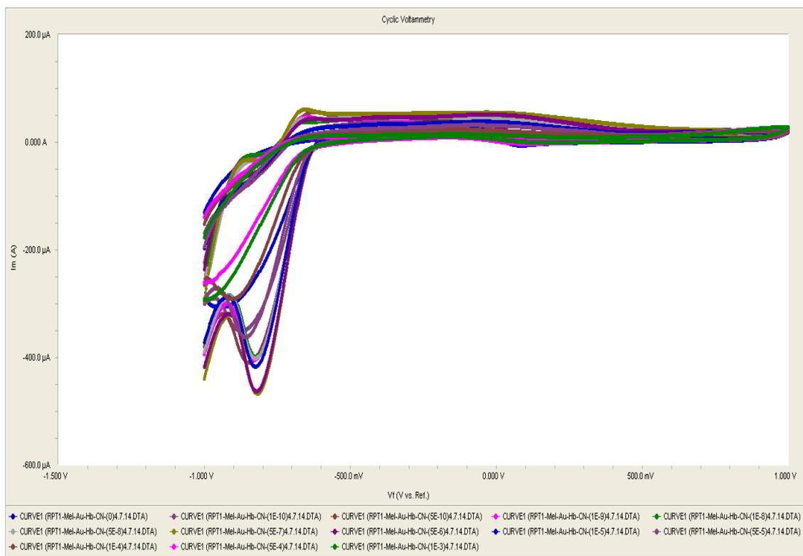
Figure C.69 Platinum Electrode II Ran With CN From Concentration  $1e-10$  to  $1e-3$ , [-1.0, 1.0] V, 04.07.2014
