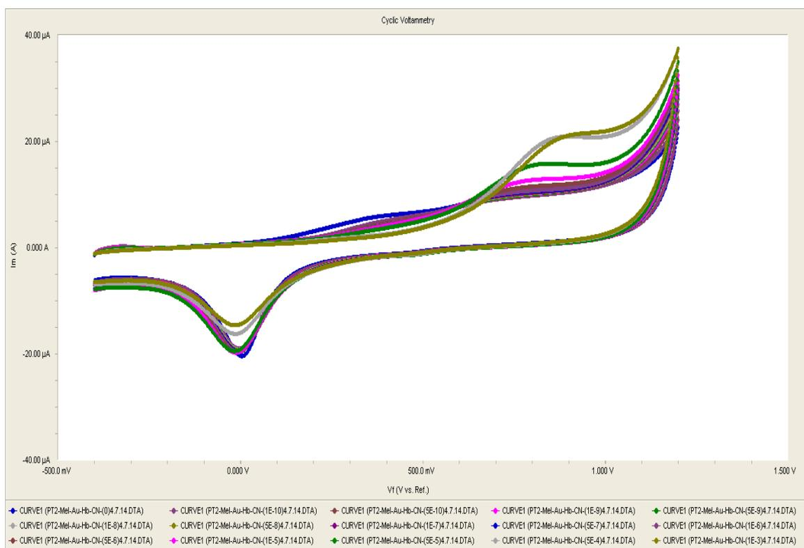
Figure C.68 Platinum Electrode I Ran With CN From Concentration  $1e-10$  to  $1e-3$ , [-1.0, 1.0] V, 04.07.2014
