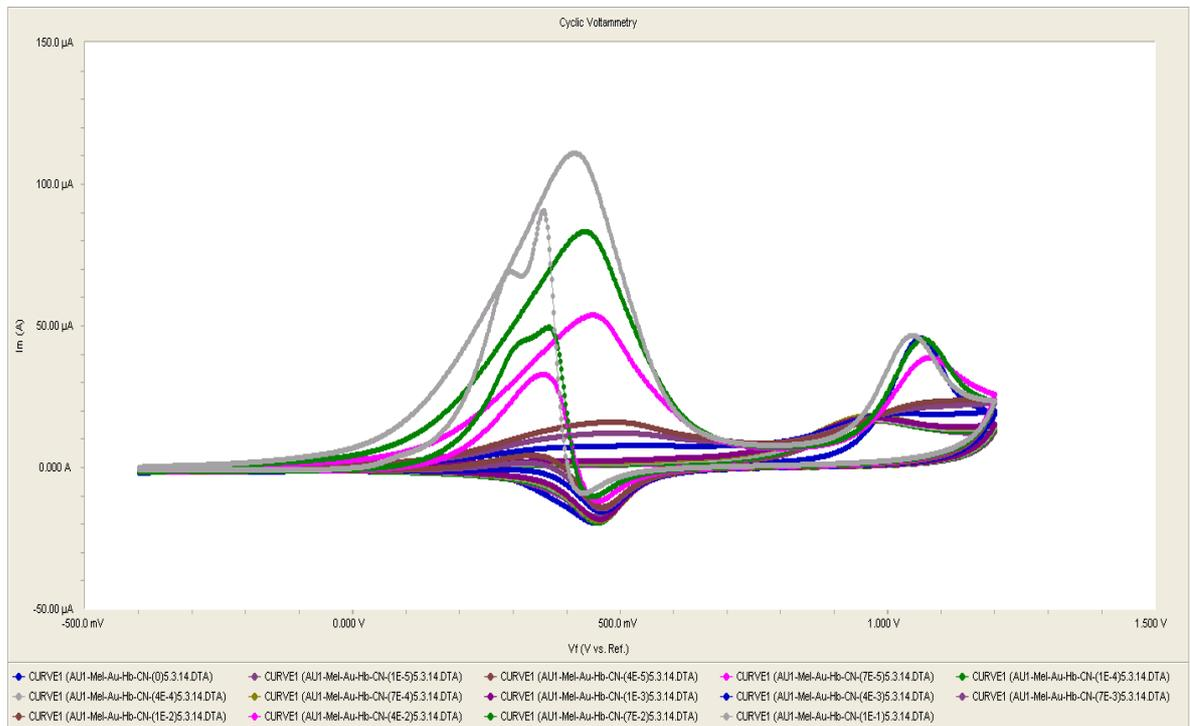
Figure C.39 Gold Electrode II Ran With CN From Concentration  $1e-5$  to  $1e-1$ , [-0.4, 1.2] V, 05.03.2014
