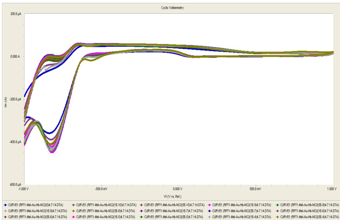
Figure C.63 Platinum Electrode II Ran With  $\text{NO}_2$  From Concentration  $1e-10$  to  $1e-3$ , [-1.0, 1.0] V, 04.07.2014
