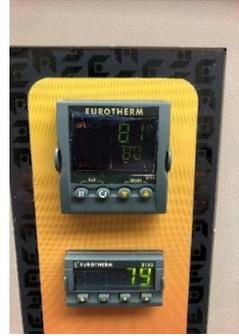
b) The temperature and set point during the 1-hour bake out.
