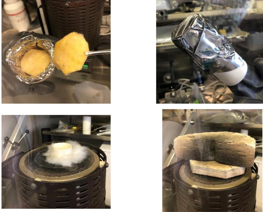
FIGURE 44 NEW CONFIGURATION EXPERIMENT WHERE THE INSULATION SAMPLE IS HALVED TO PLACE SODIUM METAL INSIDE WITH ALUMINA BEAKER PLACED ON TOP TO ADD PRESSURE.
