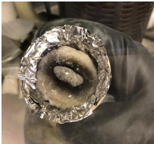
FIGURE 48 INSULATION HOLE CONFIGURATION WITH ALUMINA BEAKER APPLYING PRESSURE.
