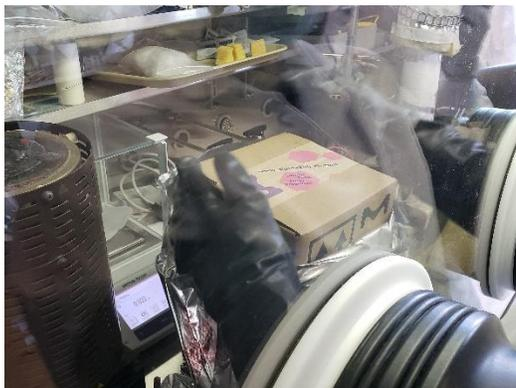
a) Removal of sealed bag from sodium metal packaging
