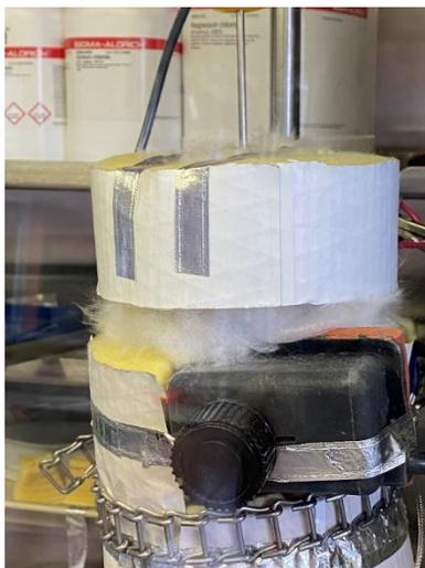
a) Insulation material inserted into gaps around the cap
