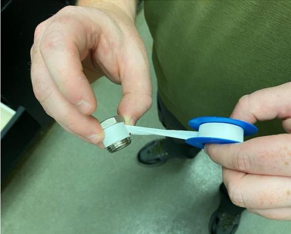
b) Threads were wrapped with PTFE pipe tape.
