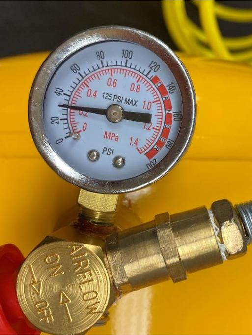
a) Air tank was pressurized to about 30 psi.
