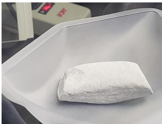
d) Sodium chunk removed for observation revealing oxide layer
