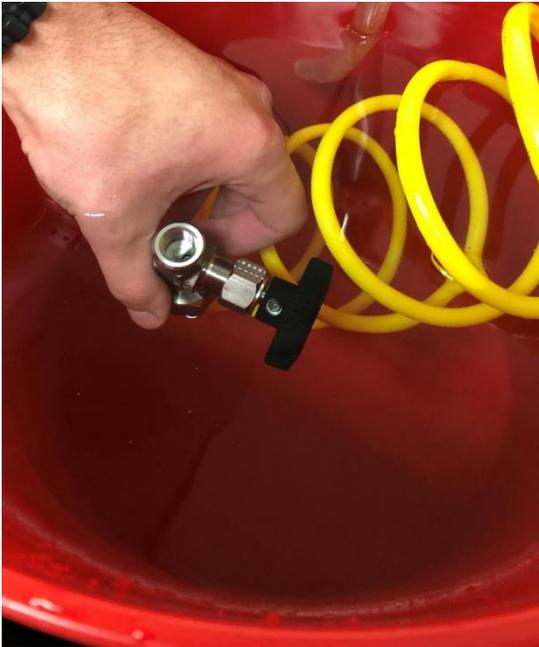
d) Pressurized parts were submerged under water and observed for bubbles.
