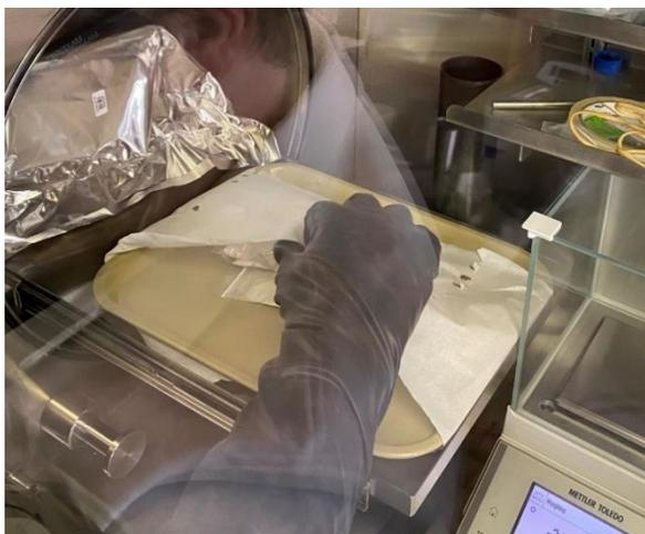
a) Met-L-X bags being transferred into the glovebox via the antechamber tray.
