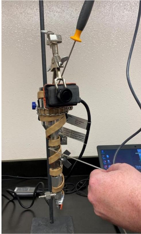
FIGURE 23. HEAT TAPE BEING TESTED ON THE ASSEMBLY.
