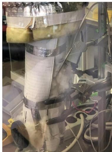
b) Insulation material inserted around ball valve handle
