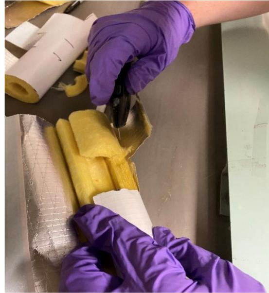
b) A box cutter knife and scissors were used for making the cutouts.
