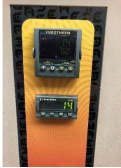
a) Front display showing the temperature and set point just after being turned on.
