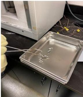
c) Small pieces removed via tongs into stainless steel container.
