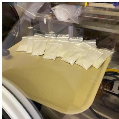
c) Arraying the open bags for long term outgassing in the glovebox.
