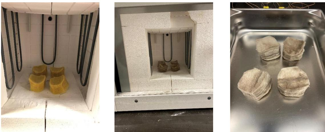
FIGURE 46 INSULATION SAMPLES BEING PLACED INSIDE THE INDUSTRIAL OVEN AND LATER REMOVED ONCE DONE BAKING.
