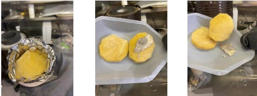
FIGURE 45 NEW CONFIGURATION RESULTS AFTER COOLDOWN SHOWING THE SODIUM METAL NOT INTERACTING WITH THE INSULATION AND SPREADING OUT INSTEAD.
