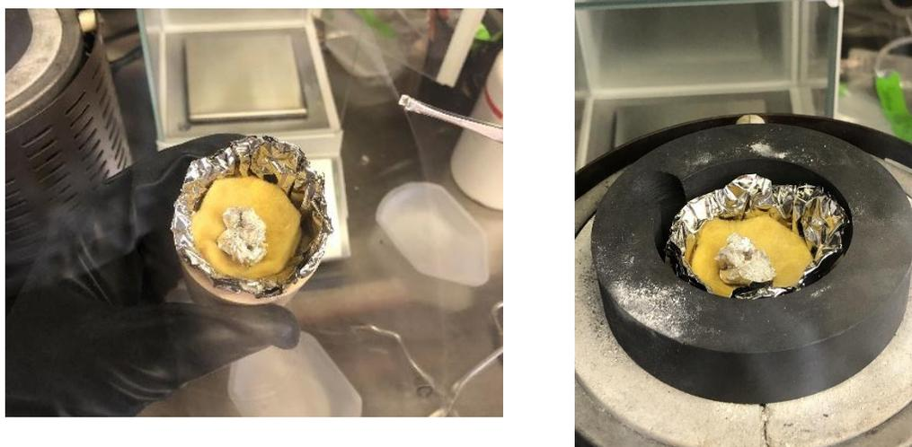
FIGURE 42 SODIUM METAL PIECE SET ATOP INSULATION SAMPLE AND PLACED INSIDE GRAPHITE MANTLE OF THE JEWELER'S FURNACE.
