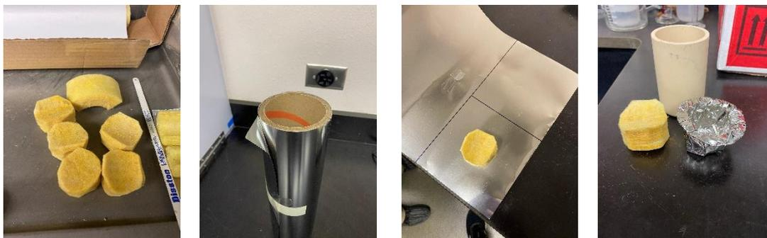
FIGURE 41 INSULATION SAMPLE, STAINLESS STEEL FOIL, AND ALUMINA CRUCIBLE FABRICATION FOR THE JEWELER'S FURNACE.
