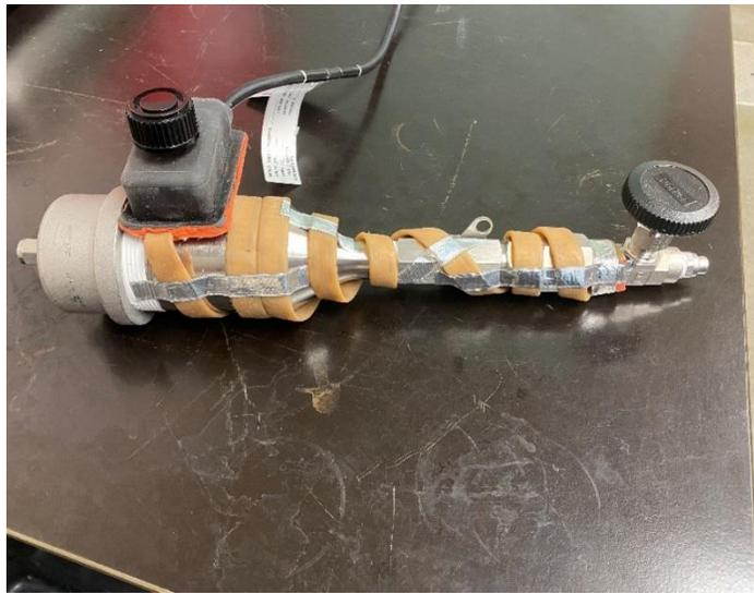
c) Heat tape is helically wrapped around the final assembly and secured using aluminum tape.
