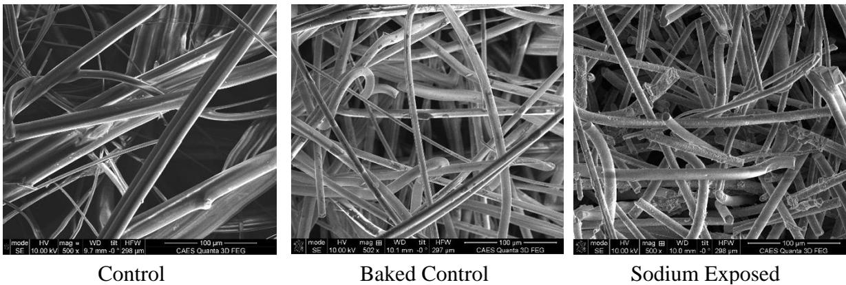
FIGURE 59 IMAGES OF A CONTROL, BAKED CONTROL, AND SODIUM EXPOSED SAMPLE. SODIUM EXPOSED SAMPLE SHOWS DEVIATIONS COMPARED TO THE OTHERS.
