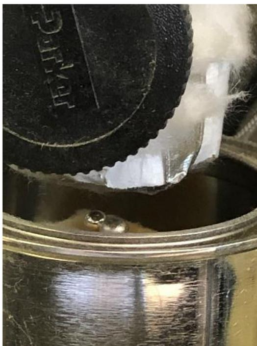
FIGURE 39 SODIUM METAL DROPLETS OBSERVED SITTING ON INSULATION SAMPLE.
