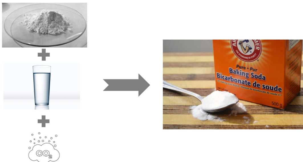
FIGURE 9 SODIUM CARBONATE, CARBON DIOXIDE AND WATER REACTION INTO SODIUM BICARBONATE.
