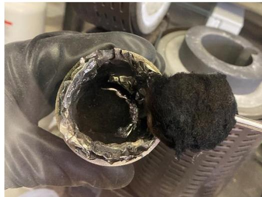
FIGURE 50 VARIATION OF THE SANDWICH METHOD WHERE SODIUM METAL IS BELOW THE INSULATION.
