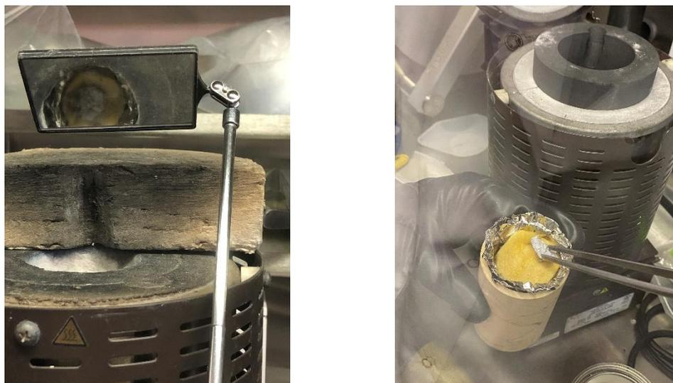
FIGURE 43 RETRACTABLE MIRROR USED TO OBSERVE SODIUM METAL INSIDE JEWELER'S FURNACE. STAINLESS STEEL TWEEZERS USED TO INVESTIGATE SODIUM METAL AFTER COOLDOWN.
