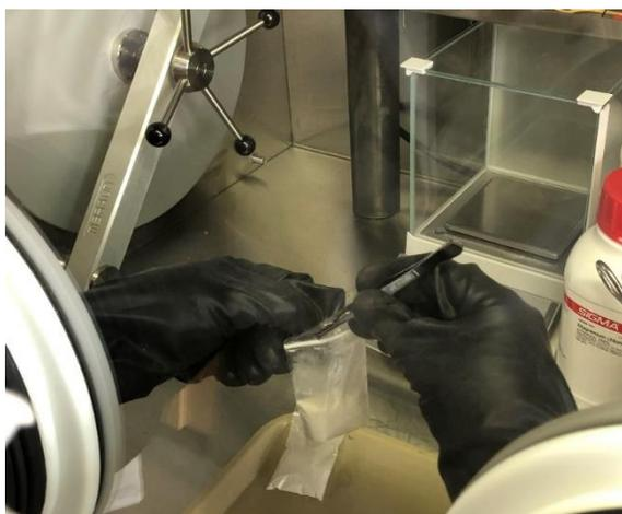
b) Opening the Met-L-X bags for outgassing with the help of tweezers
