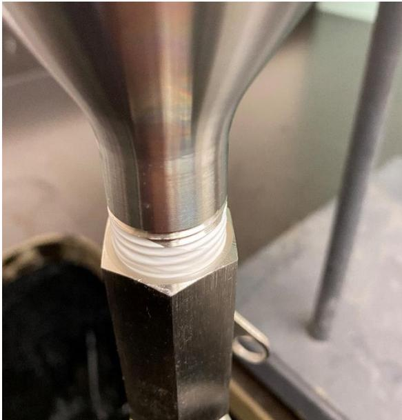
c) Inspect threads to make sure water is not seeping through.
