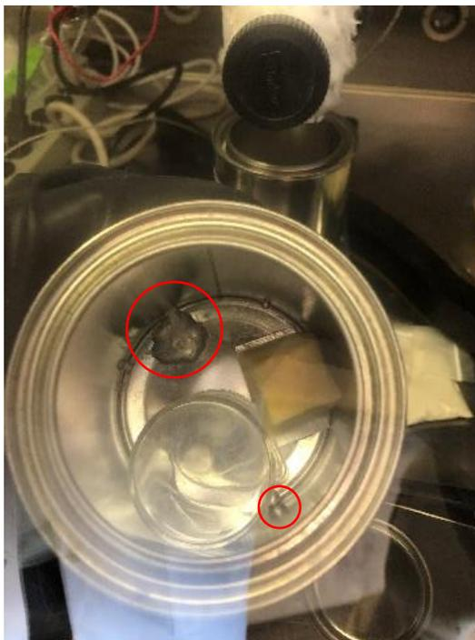
FIGURE 40 INSIDE VIEW OF THE PAINT CAN AFTER SODIUM DROPLETS FORMED.
