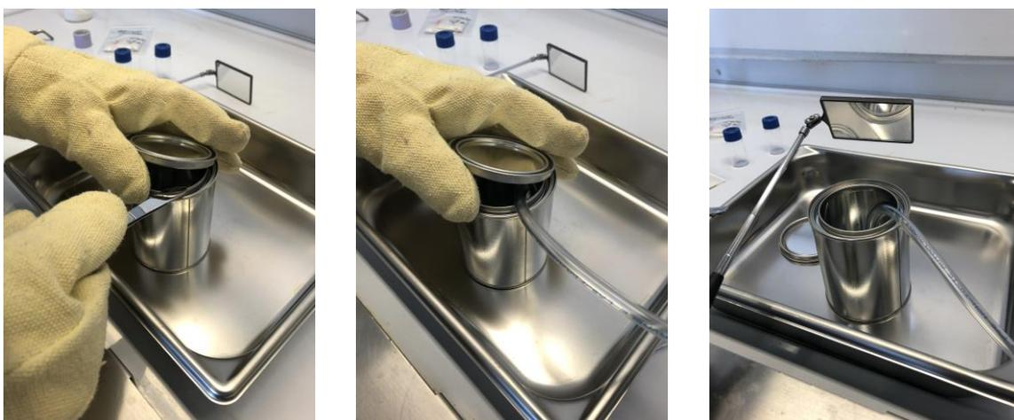
FIGURE 53 OPENING OF THE PAINT CAN FOR THE ARGON FEED TO BE INSERTED. THE SAMPLE IS VISUALLY CHECKED UTILIZING A RETRACTABLE MIRROR.
