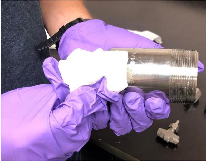
a) Parts are wiped down with 'Kimwipes' to remove any excess oils or residues.
