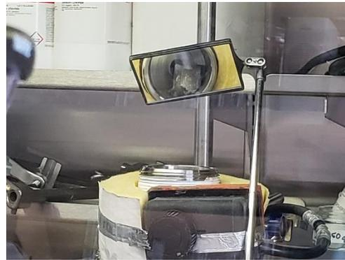
FIGURE 38 SODIUM PIECE PLACED INTO THE DRIP ASSEMBLY VESSEL AND VISUALLY CONFIRMED USING A MIRROR.
