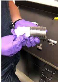
c) Wipe down of the assembly prior to entry into the furnace
