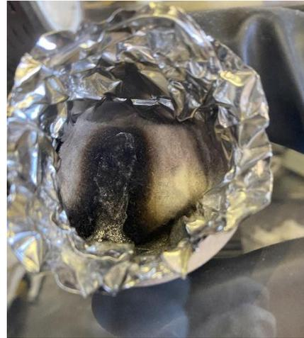
FIGURE 49 SANDWICH METHOD WITH BAKED INSULATION.
