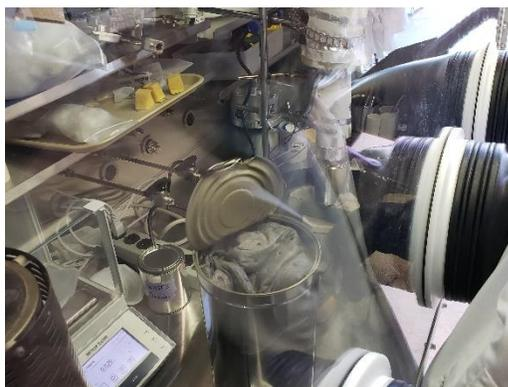
c) Opening of metal canister to reveal packing material
