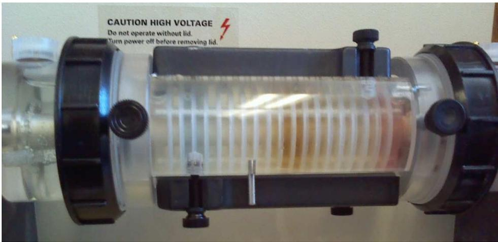
**Figure 2.1. The Rotofor® with the test proteins showing the separation of the known proteins to their prospective pI range.**
