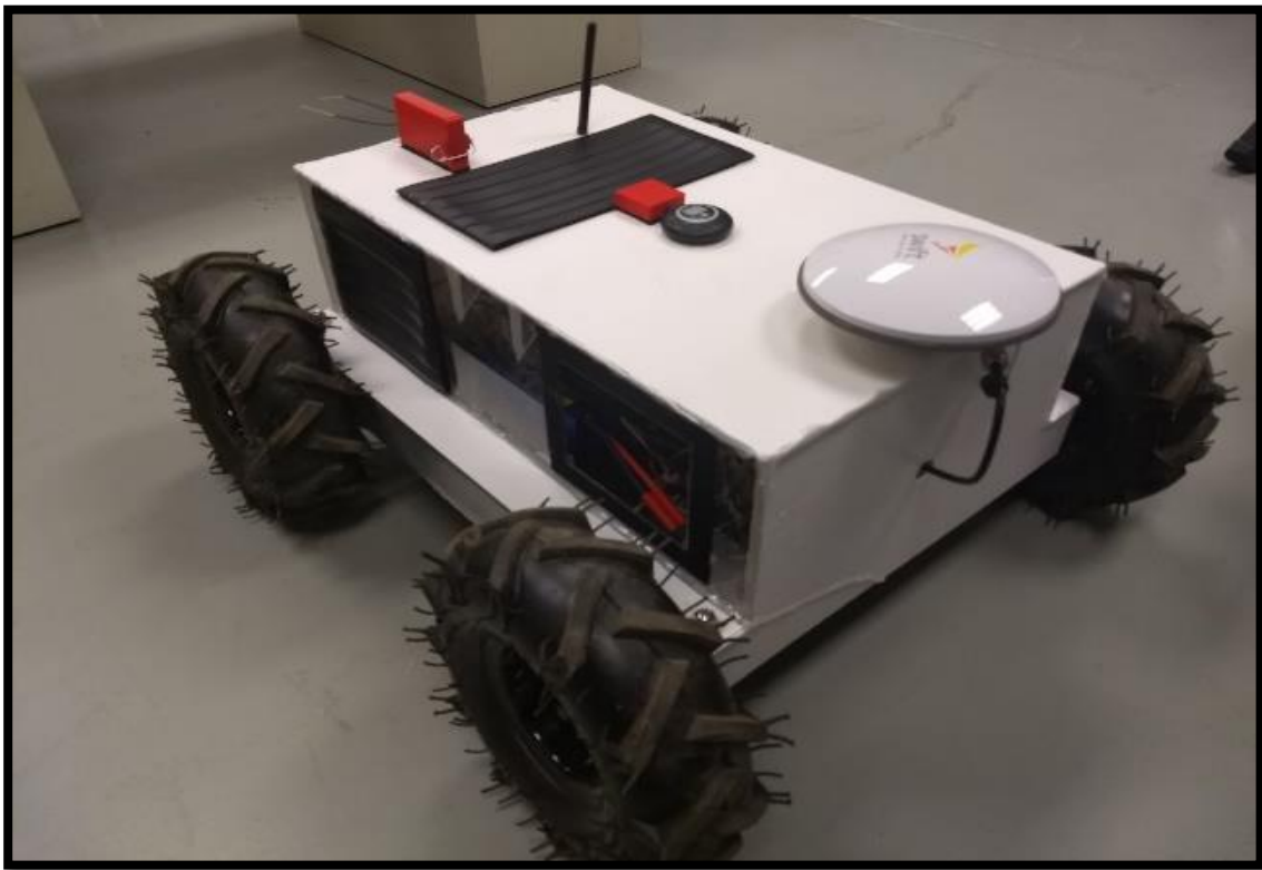
Figure 26: Assembled and painted enclosure, placed on top of robot chassis
