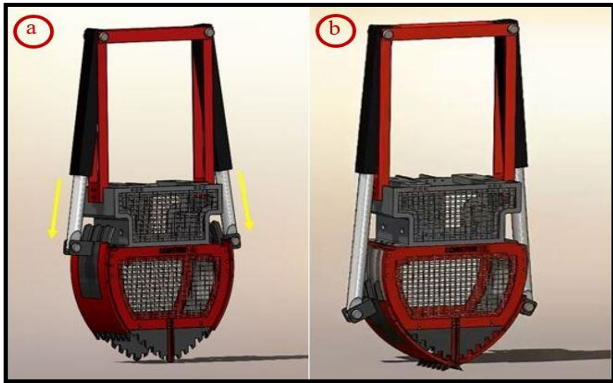
Figure 59: Actuation of blades by a hydraulic system in the final design
