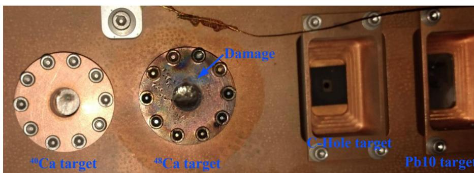
Figure 3.21: Photograph of accidental damage to  $^{48}\text{Ca}$  target. An accidental mis-steering of the beam causes it to hit the copper frame of the  $^{48}\text{Ca}$  target, causing the target to melt (photo taken from Dave Meekins’s logbook).
