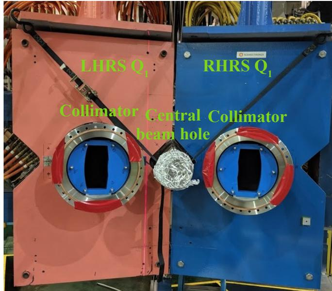
Figure 3.23: Photograph during installation of the PREX-2/CREX acceptance-defining collimators for the left and right HRSSs. The left and right collimators are symmetric with respect to the beamline which is shown in between the two collimators.
