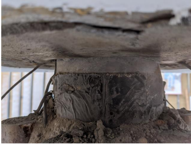
a) Bulging HSS Pipe
