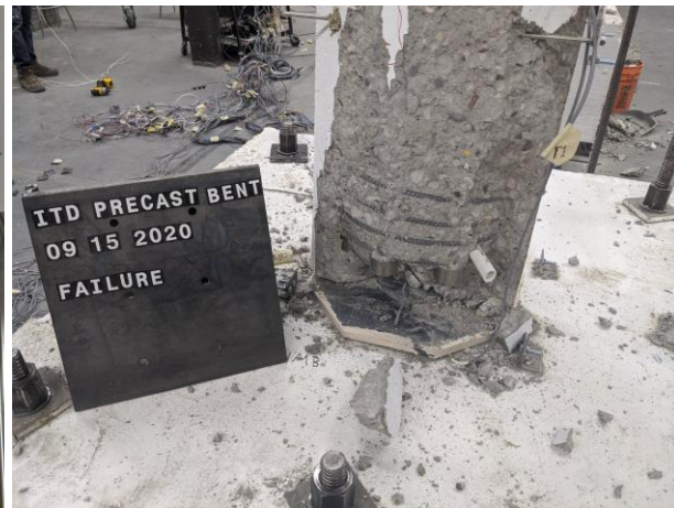
d) Cycle 24: Failure
