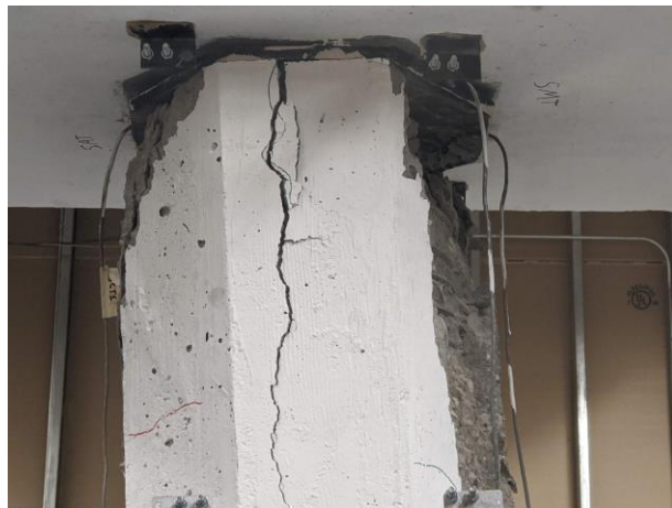
c) Cycle 24: Confinement Failure
