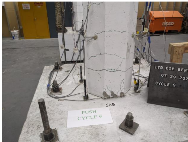
e) Cycle 9: Base Connection Spalling
