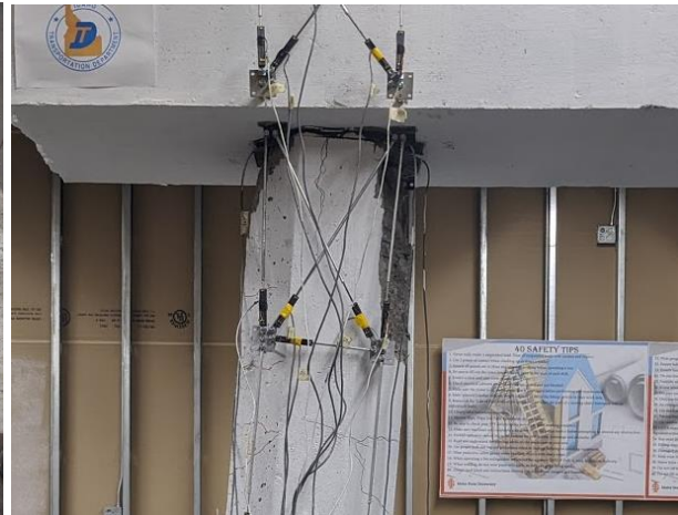
b) Cycle 19: Perpendicular Face Cracking
