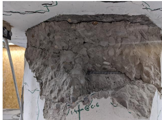
f) Cycle 13: Spiral Exposure
