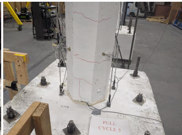
b) Cycle 5: Vertical Hairline Cracking
