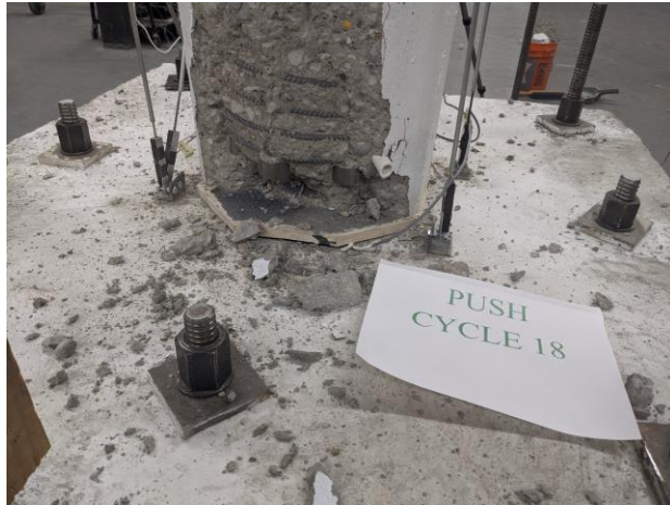
a) Cycle 18: HSS Pipe Exposure
