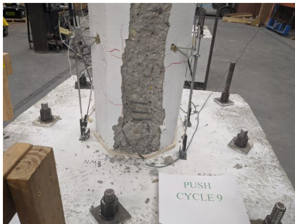
e) Cycle 9: Slab Spalling Bottom
