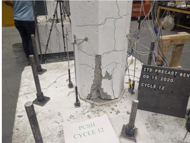
g) Cycle 12: Slab Spalling North
