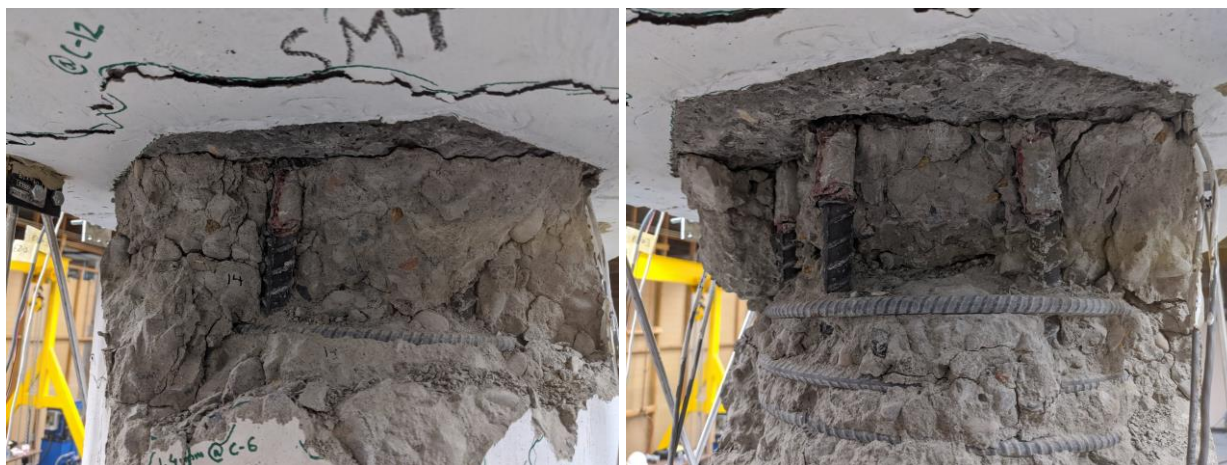
g) Cycle 14: Longitudinal Exposure
