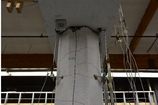
c) Cycle 6: Spalling Development
