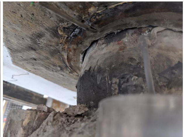
d) HSS Bulging and Separation
