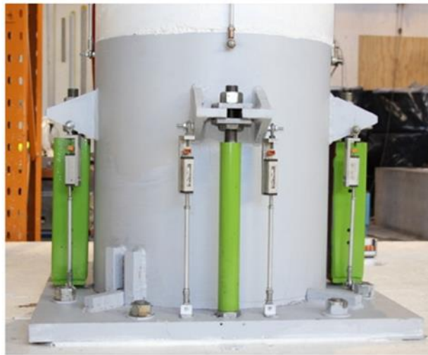
Figure 2-1: Low-Damage Seismic Connection Detail (courtesy of Mashal and Palermo 2019a)
