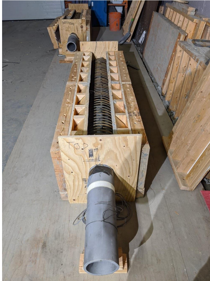
Figure 4-11: Precast Bent Pier Prepared for Concrete
