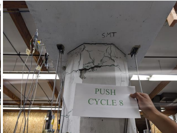
d) Cycle 8: Spalling and 2.5 mm cracking
