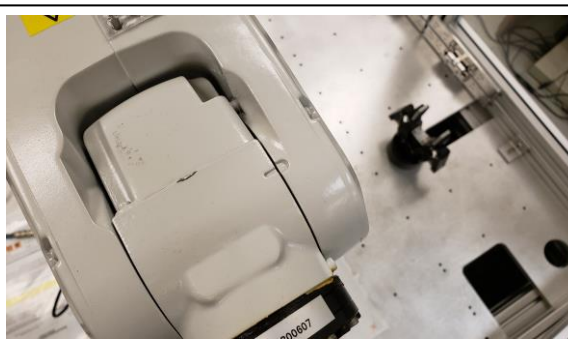
Figure 5-8: Calibration marks for Axis 5
