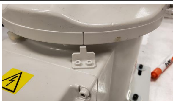
Figure 5-9: Calibration marks for Axis 1
