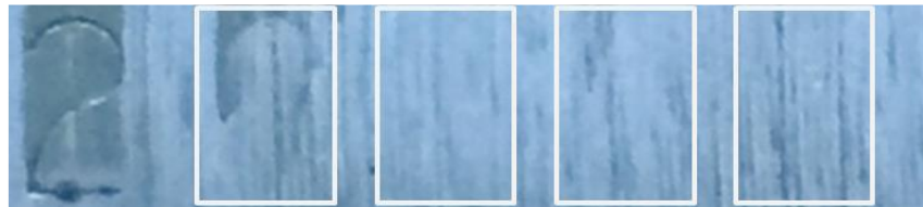
Figure 3-2 Non-defaced two, partly defaced six, and completely defaced two, five and zero [1]
