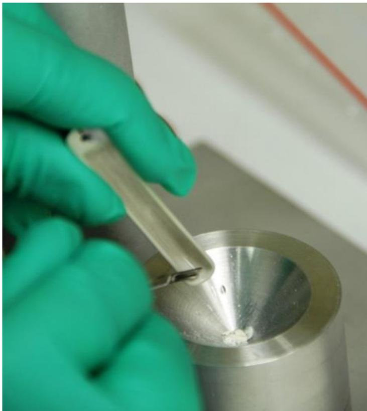
Figure 1.5.4.3 Funnel setup used to fill the vials with samples
