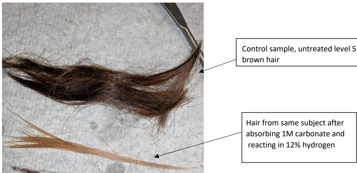
Figure 20. Results of sodium carbonate and hydrogen peroxide on level 5 brown hair.
