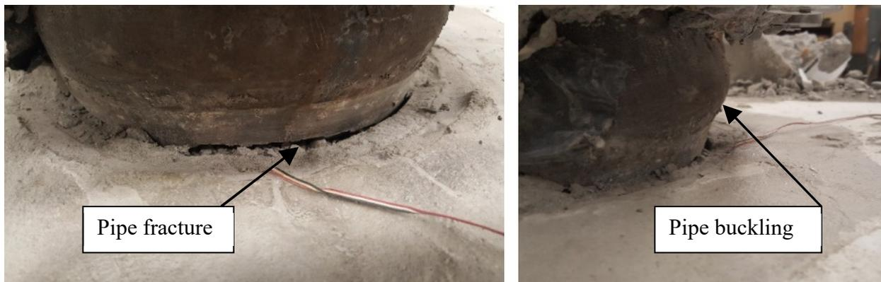
Figure 4.8: Pipe failure during the testing procedure.
