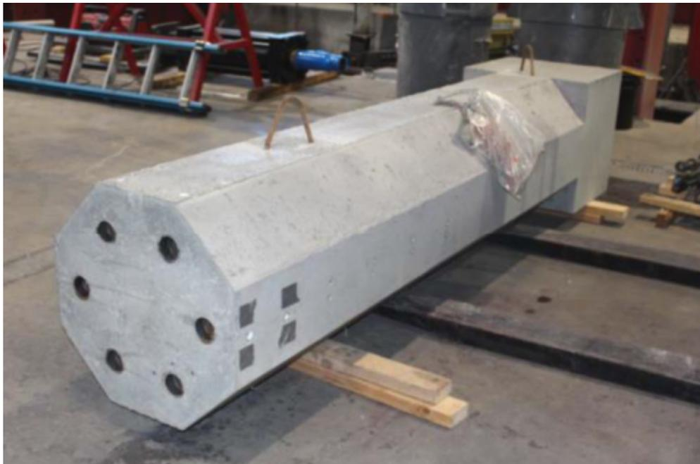
Figure 2.4: Precast column for testing mechanical bar splices (courtesy of Tazarv and Saiidi 2015b).
