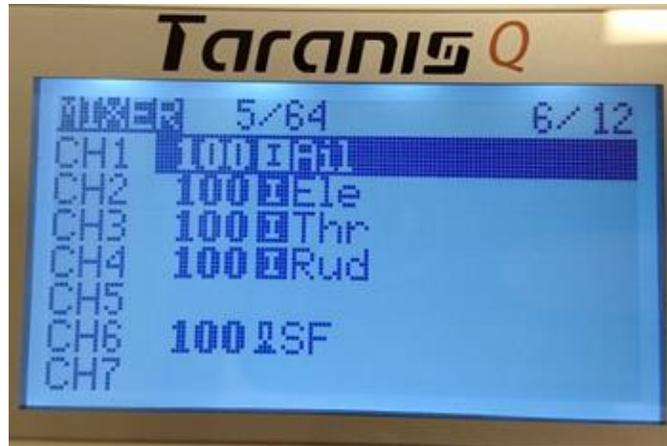
Fig 9. Configuration for channel mixing on the Taranis transmitter. The switch used channel 6.
