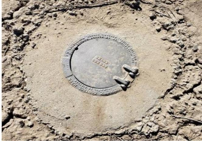
Fig 12. A photograph of a geodetic marker, taken by the author.
