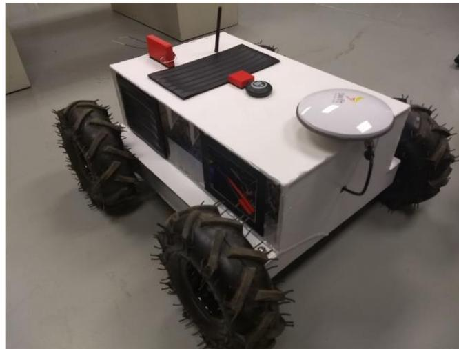
Fig 4. Ensembled and painted enclosure, with electrical components mounted and placed on top of robot chassis.
