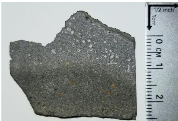
**Figure 9.** Billet cross section displaying the light colored exterior with dominantly white vesicle infill and dark interior with dominantly red-orange infill. This section also displays a ~mm thick pyrite rind on the exterior (NA100-31).
