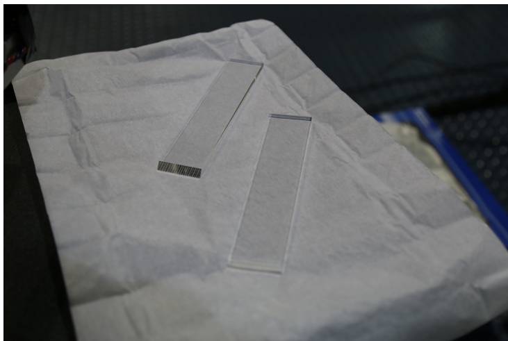
Figure 25: Polished quartz tiles for PREX-II/CREX detector.
