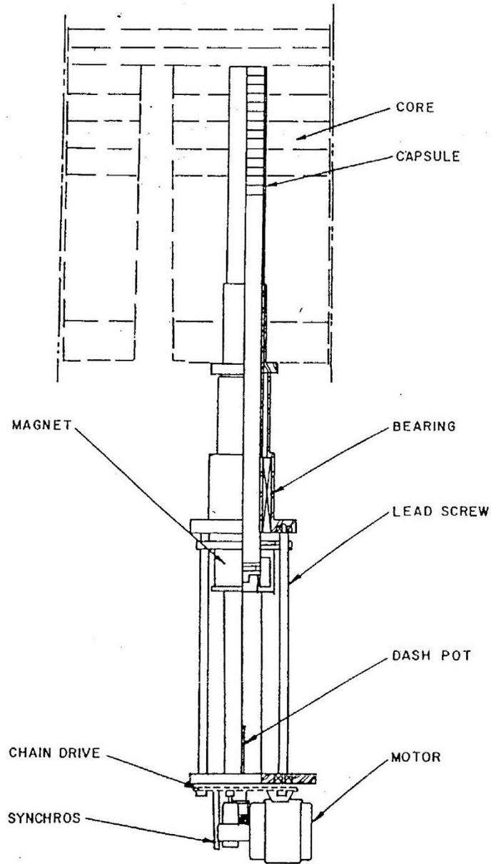
Figure 2. Control Rod Drive [3]
