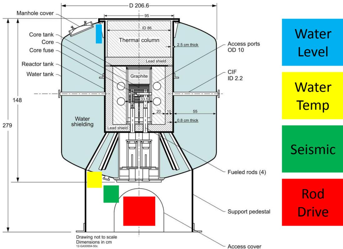
Figure 8. Reactor cross section (with Interlock locations added) [1]
