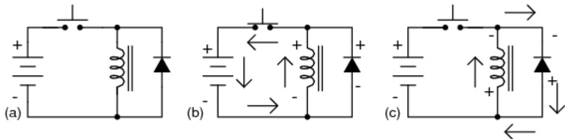
Figure 11. Reverse Biased Diode Circuit [2]
