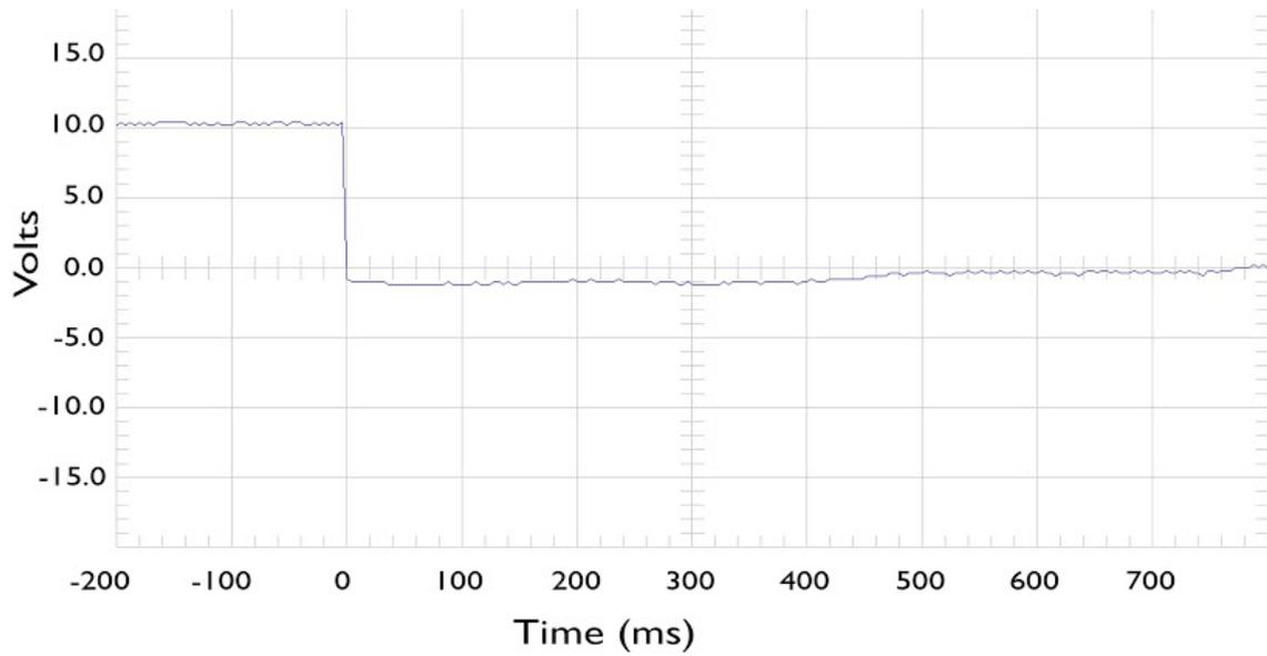
Figure 21. SR2 Voltage Spiking (Reverse Biased Diode in Parallel)
