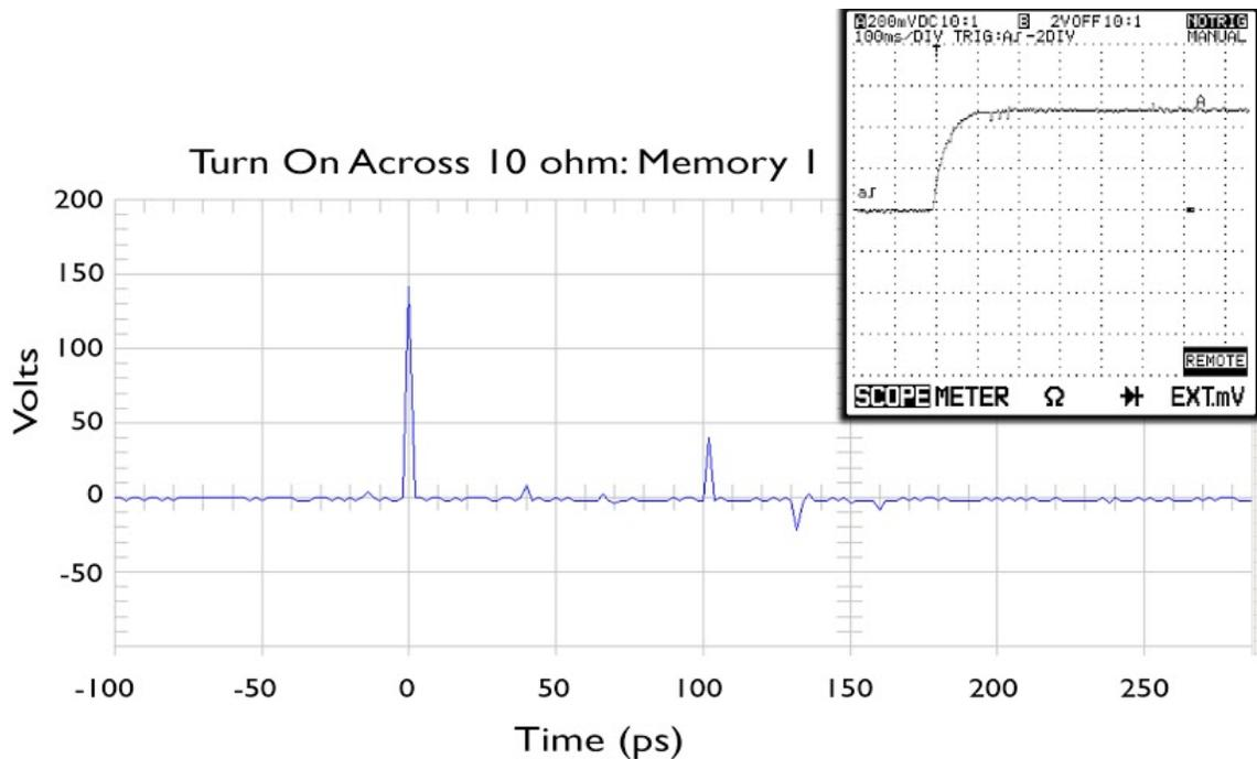
Figure 14. Oscilloscope trace across magnet during power up
