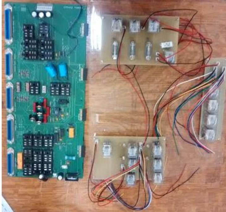
*Figure 25. PCB Safety Circuit (left) Modular Safety Circuit (right)*
