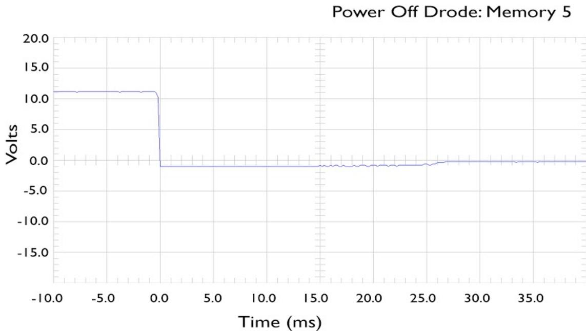
*Figure 13. Magnetic field breakdown with reverse biased diode*
