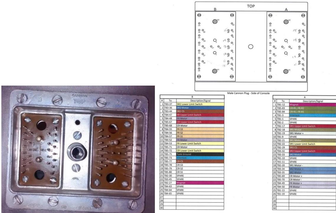
Figure 7. Reactor Plug (left) & Cable Pinouts (right) (Full size in Appendix C)
