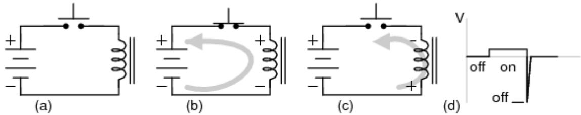
Figure 10. Power off magnetic current diagram [2]
