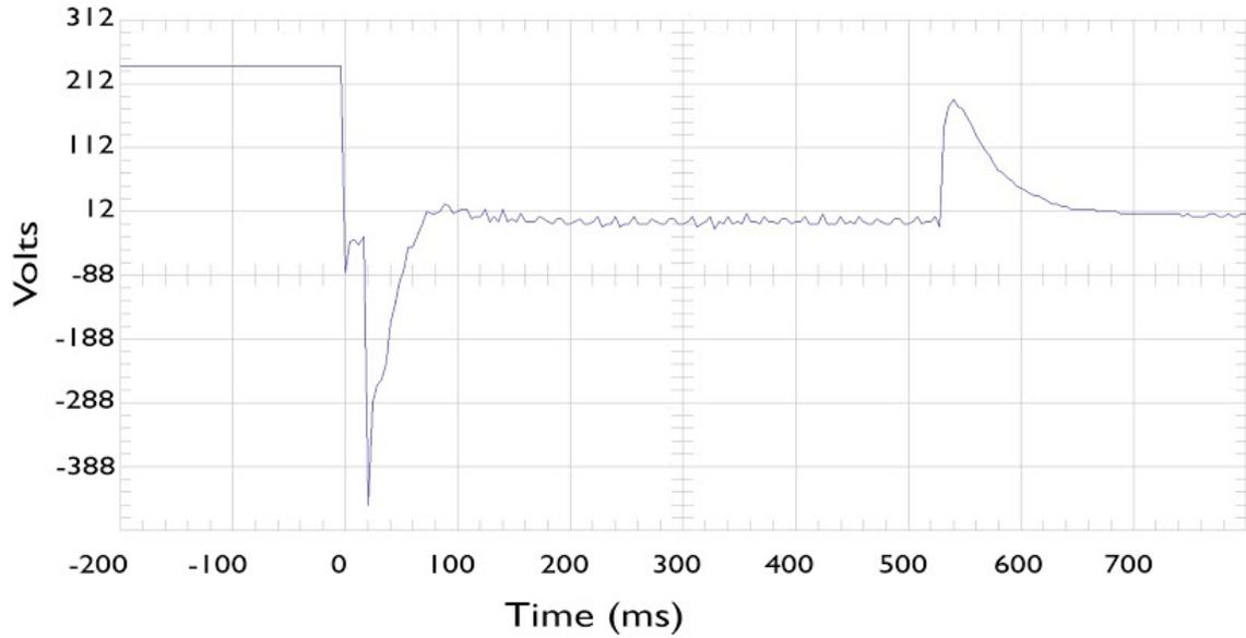
Figure 18. Ch. 1 (Oscilloscope) Manual SCRAM Button Trigger (with Reverse Biased Diode)
