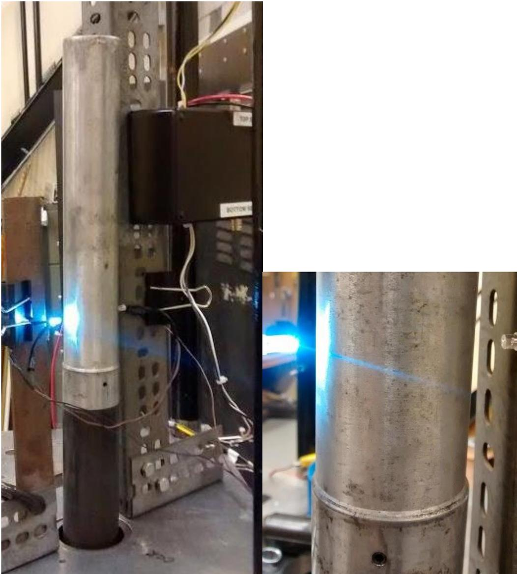
*Figure 15. SR2 Rod Drop Testing Rig (left) & Lower Rod Position Close-Up (right)*
