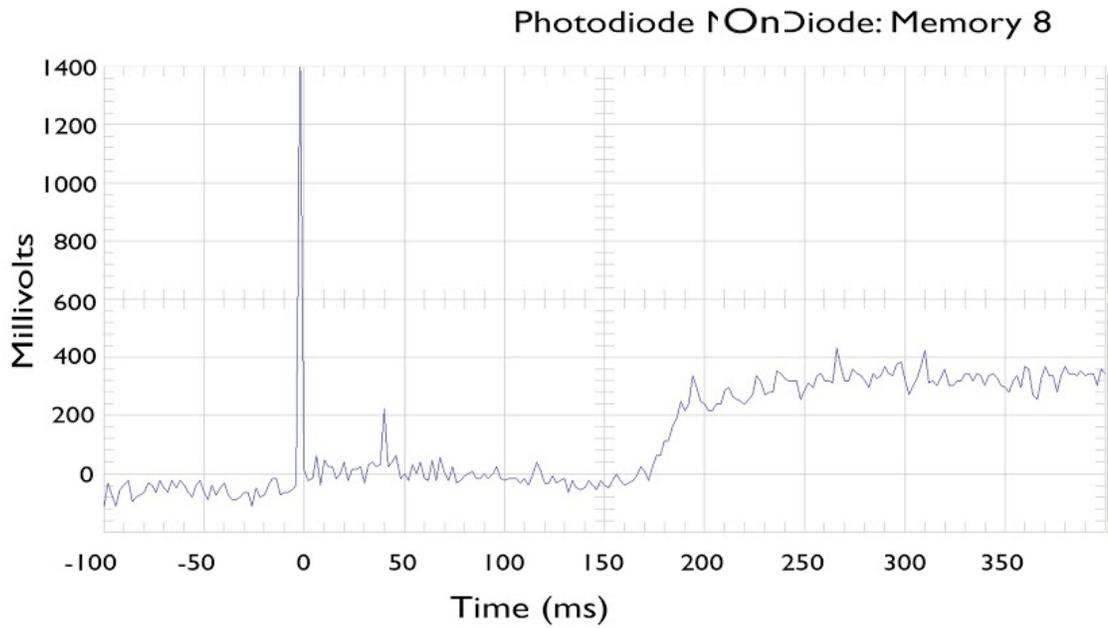
Figure 17. Ch. 2 Photo Diode Trigger (Original Circuitry with no reverse biased diode)
