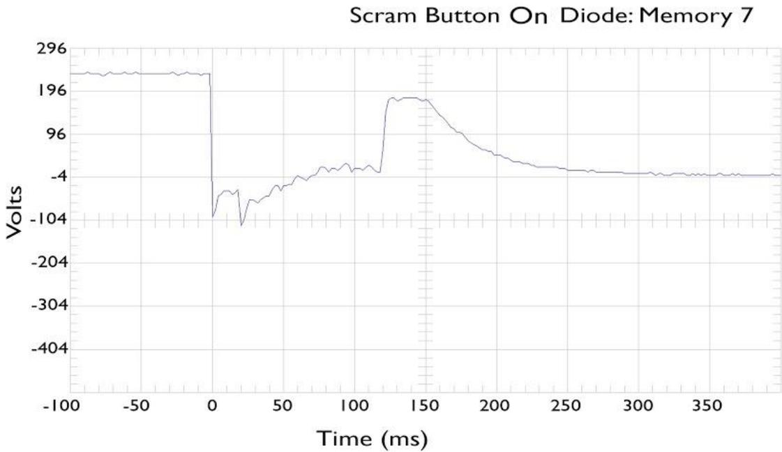
Figure 16. Ch 1 SCRAM Button Trigger (Original Circuitry with no reverse biased diode)
