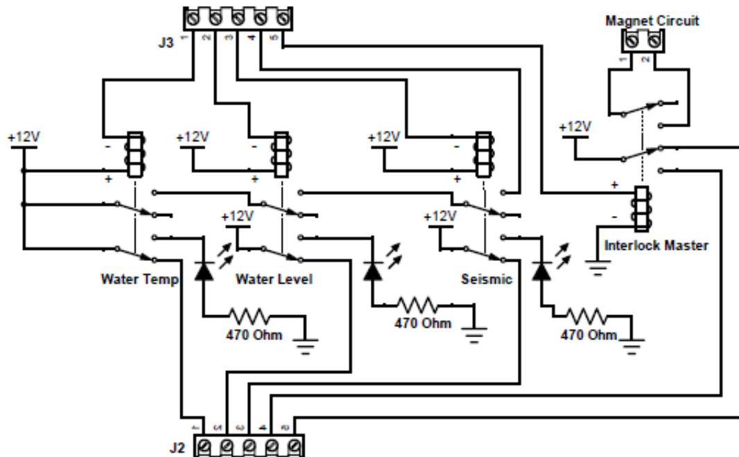
Figure 23. Interlock Circuit (See Appendix A)
