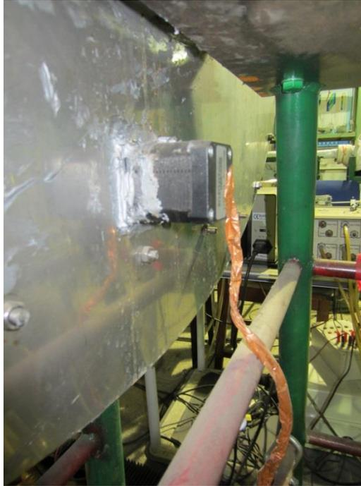
**Figure 2.5: Stepper Motor for Throttle Ring Actuation (Mounted on Compressor Exterior)**
