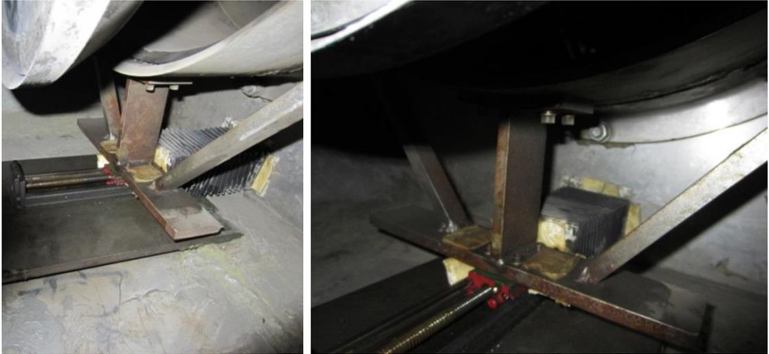
**Figure 2.4: Screw Mechanism for Throttle Actuation Side View (Left) and Frontal View (Right)**
