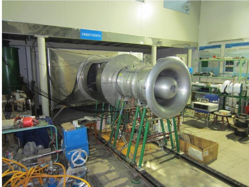
**Figure 2.1: Experimental Axial Compressor Setup at the Advanced Energy and Technology Laboratory at the Institute of Engineering Thermophysics, CAS**
