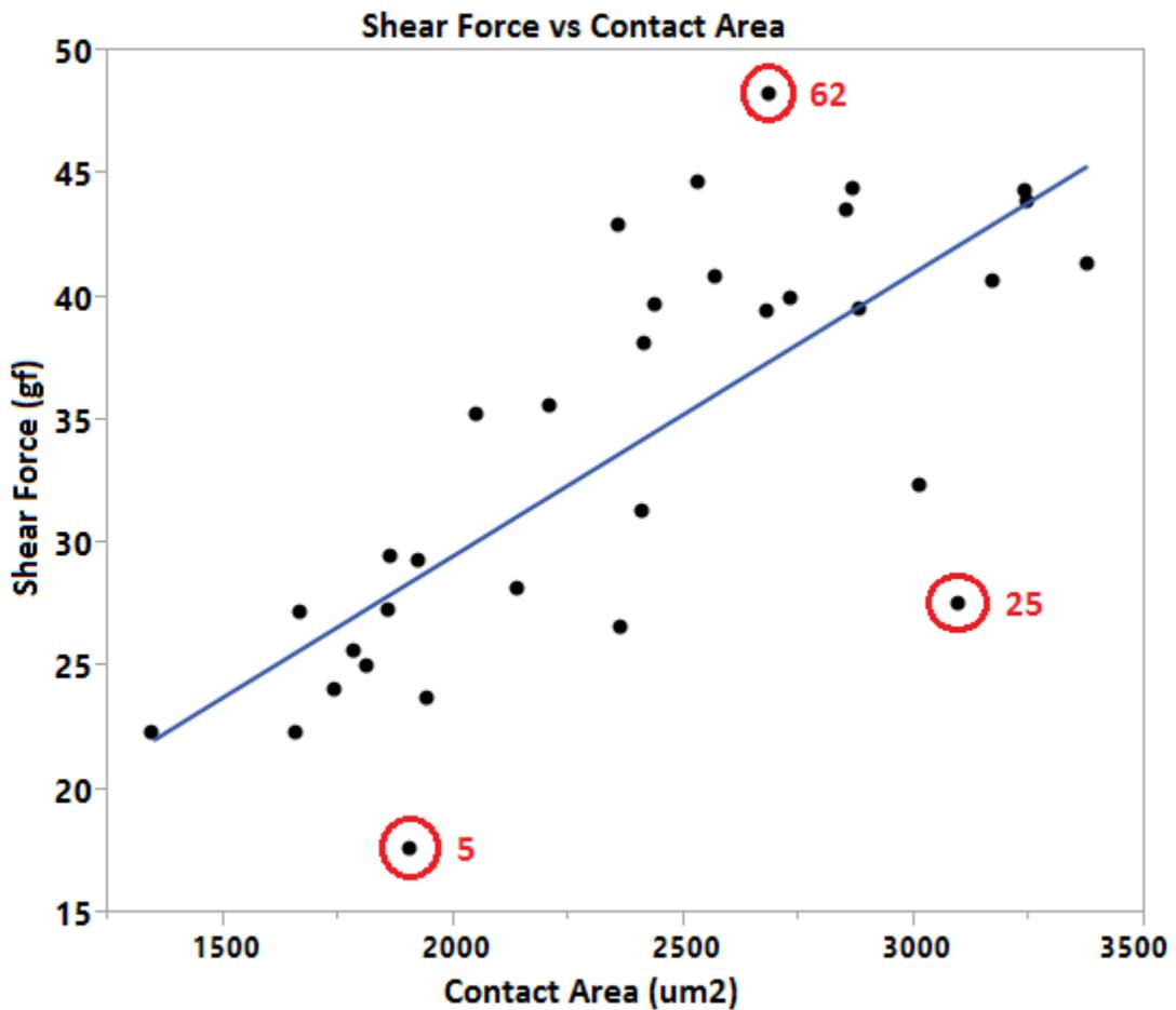
Figure 34 Shear Force vs Contact Area - BN Capillary
