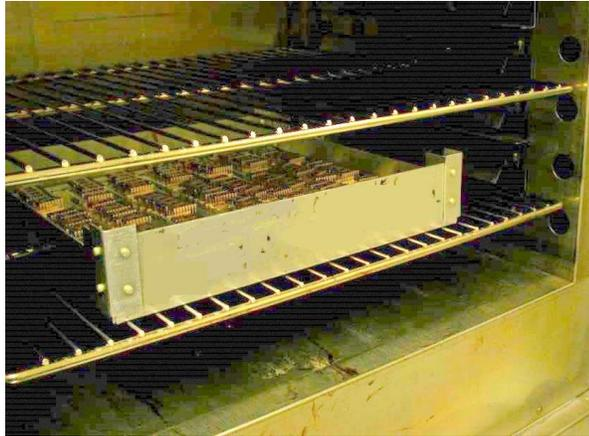
**Figure 12 Package Baking Machine**
