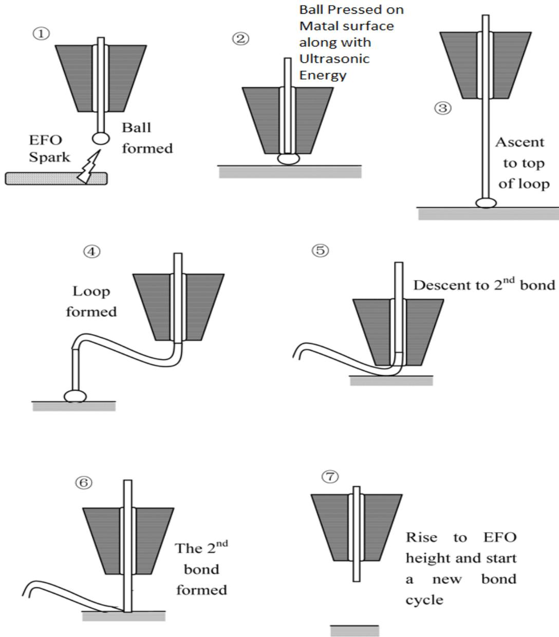
**Figure 7 Au Ball Bonding Cycle [23]**
