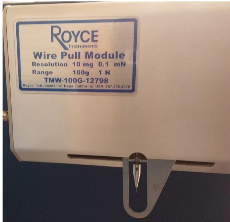
**Figure 22 Royce Instruments Wire Pull Module**
