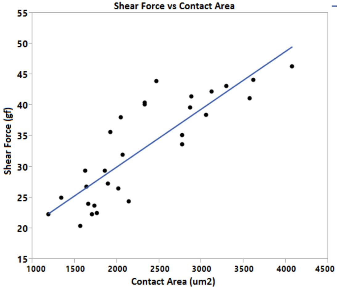
**Figure 33 Shear Force vs Contact Area - HF Capillary**
