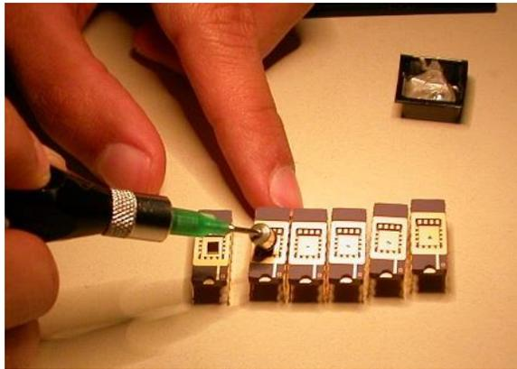
**Figure 11 Die Attach Process using Epoxy**
