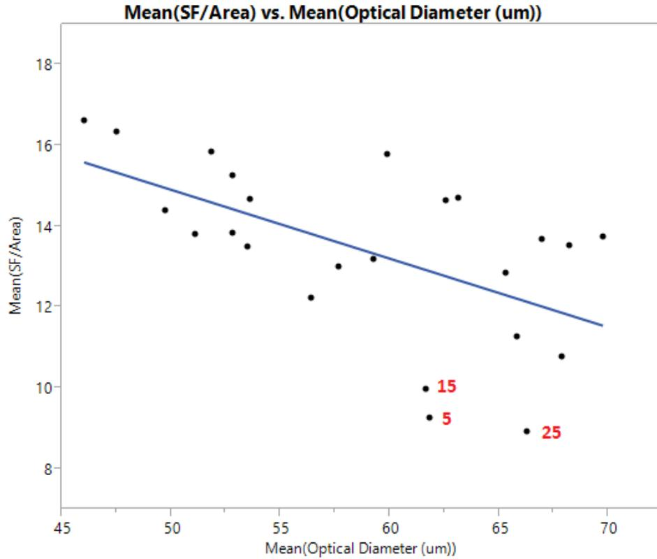
**Figure 38 Shear Force/Area vs Ball Diameter for BN Capillary**
