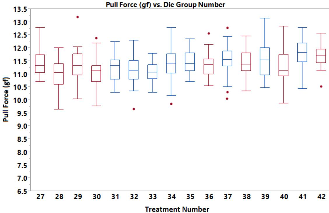
**Figure 26 Experiment 2 - Pull Force vs Treatment Box Graph**
