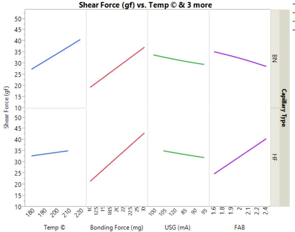
**Figure 36 Shear Force vs Factors**
