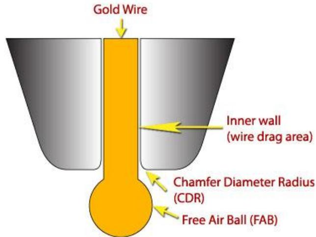
**Figure 6 Cross Section of a Capillary**
