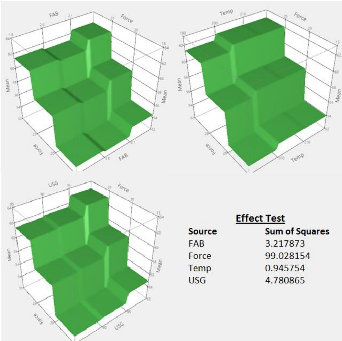
**Figure 44 Ball Dia. vs Factors Surface Profile for HF capillary**
