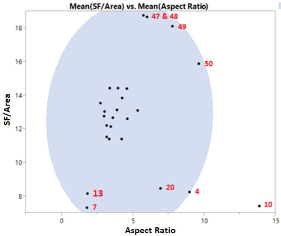
Figure 39 Shear Force per Area vs Aspect Ratio for HF Capillary
