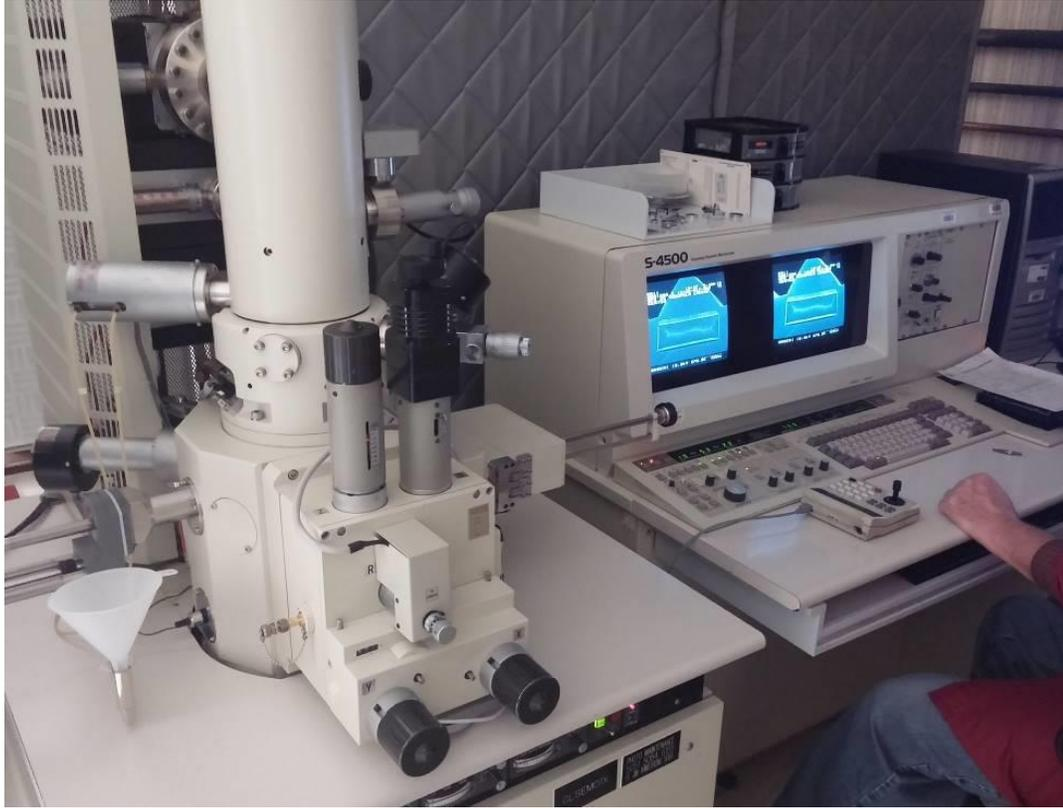
**Figure 19 Scanning Electron Microscope**
