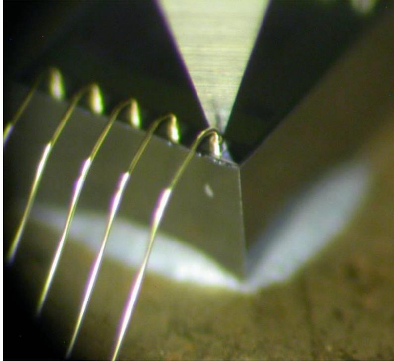
**Figure 16 Ball Shear Test**
