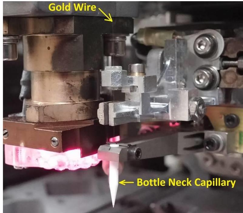
**Figure 13 Wire Bonder with Bottle Neck Capillary Mounted**
