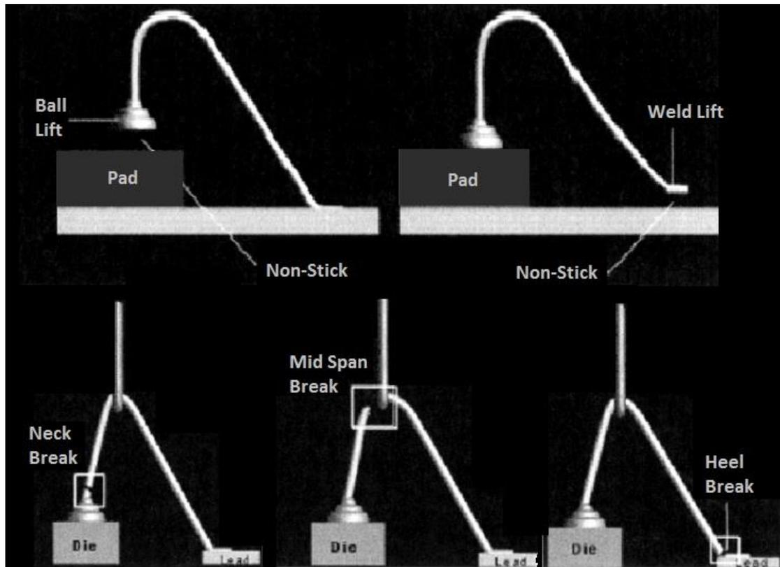
**Figure 15 Ball Pull Failures [23]**
