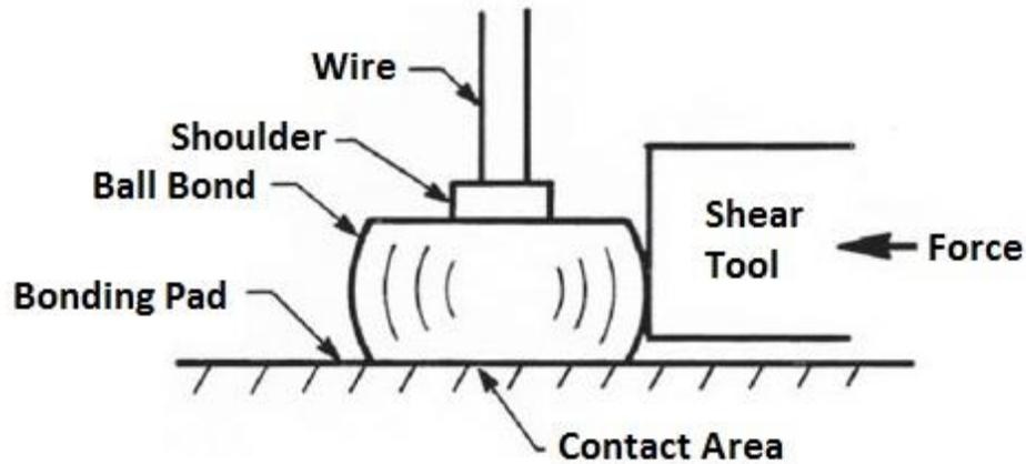
**Figure 17 Shearing Process**
