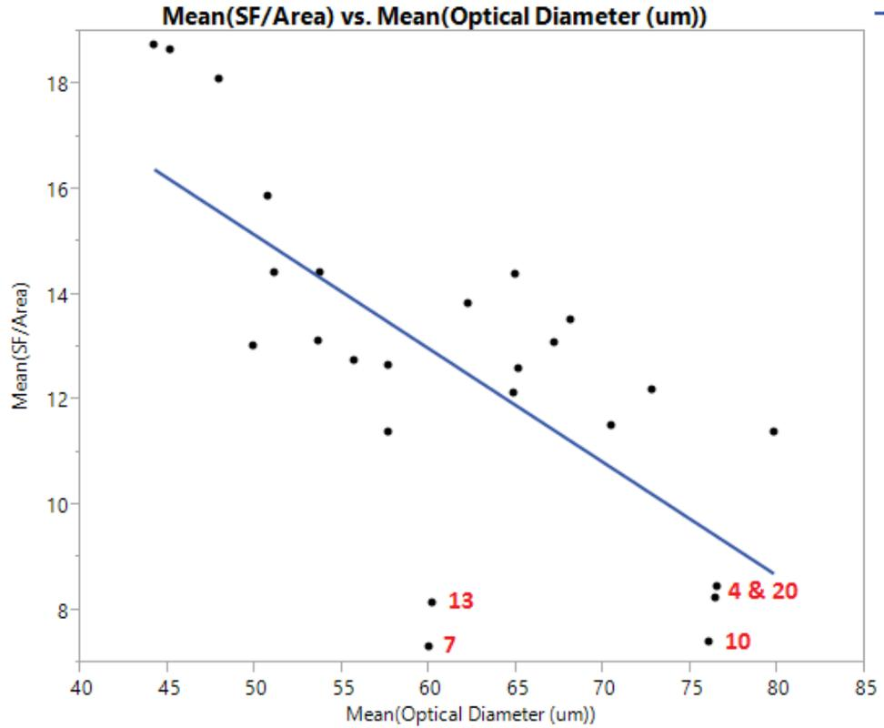
**Figure 39 Shear Force/Area vs Ball Diameter for HF Capillary**
