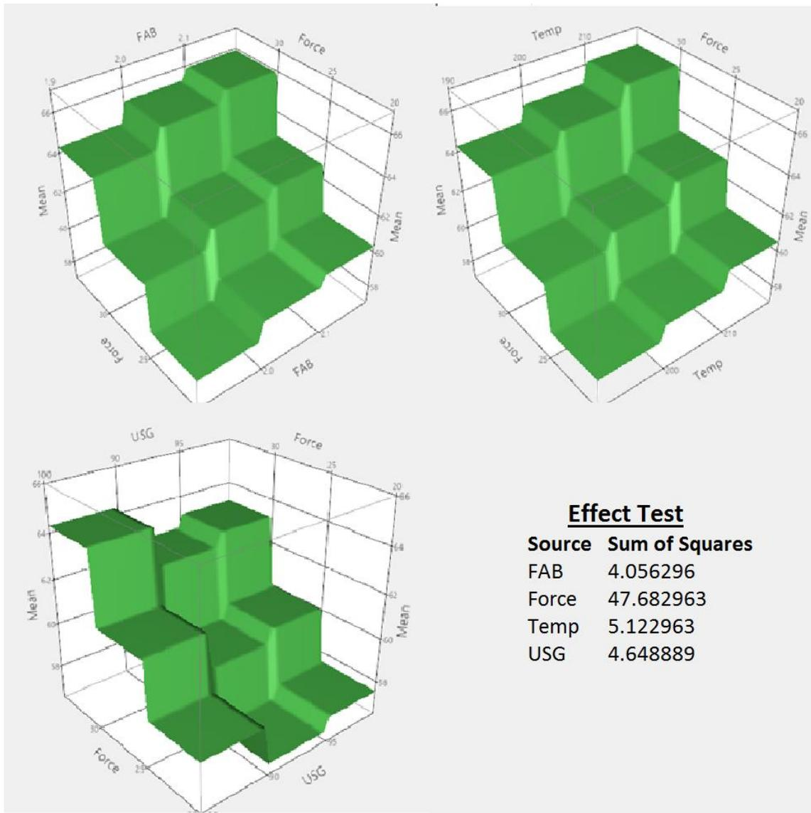
**Figure 45 Ball Dia. vs Factors Surface Profile for BN Capillary**
