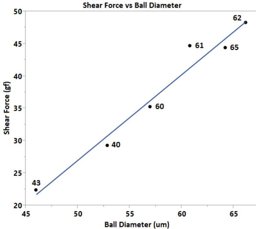
**Figure 38 Optimum BN - Shear Force vs Ball Diameter**
