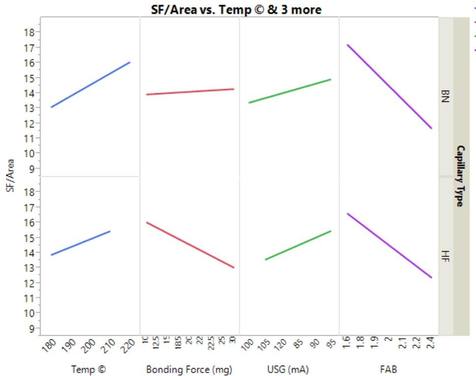
**Figure 35 Shear Force per Area vs Factors**
