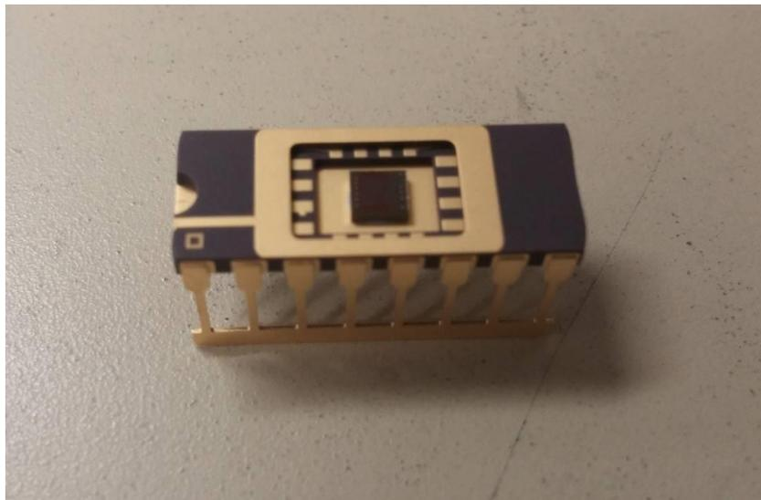
**Figure 10 16 Pin Dual-in-line Ceramic Package**
