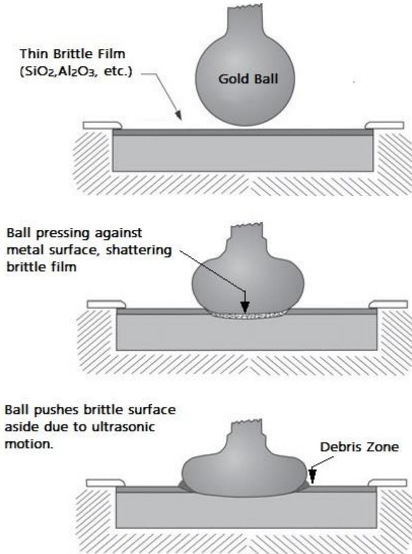
**Figure 1 US Energy Cleaning Surface Oxide Film**
