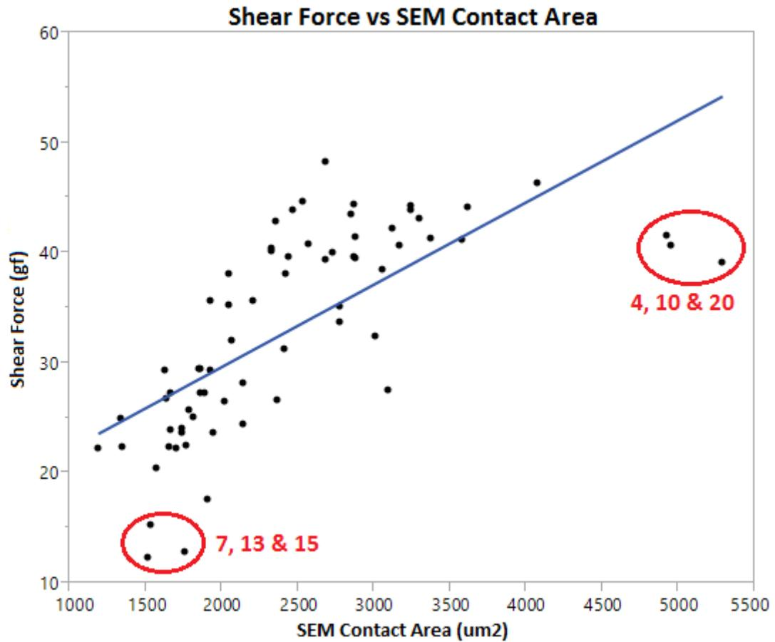
**Figure 32 Shear Force vs Contact Area**
