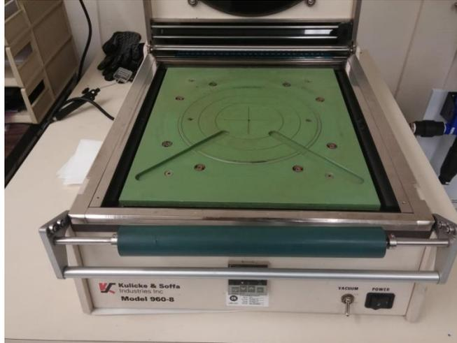
**Figure 8 Wafer film mounting machine**
