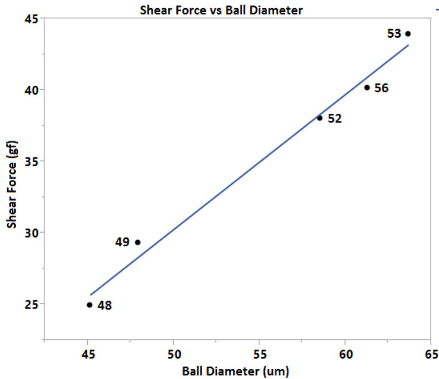
Figure 37 Optimum HF - Shear Force vs Ball Diameter
