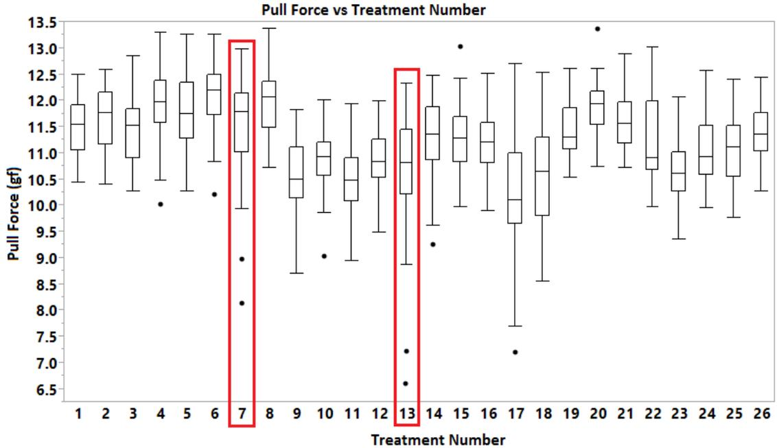
**Figure 23 Experiment 1 - Pull Force vs Treatment Box Graph**
