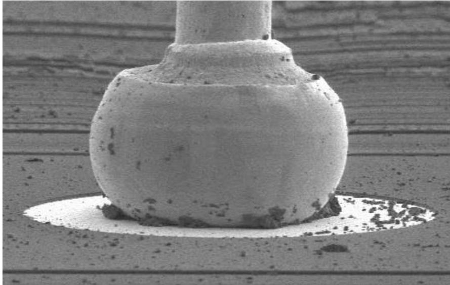
**Figure 2 Large Ball Bond with Small Contact Area**
