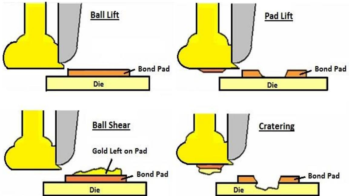
**Figure 18 Shear Test Failures**
