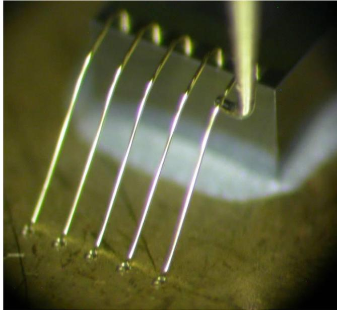
**Figure 14 Ball Pull Test**
