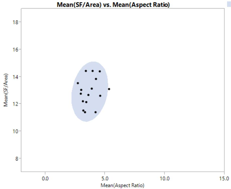
**Figure 40 Shear Force per Area vs Aspect Ratio for HF Capillary (Without Failures)**
