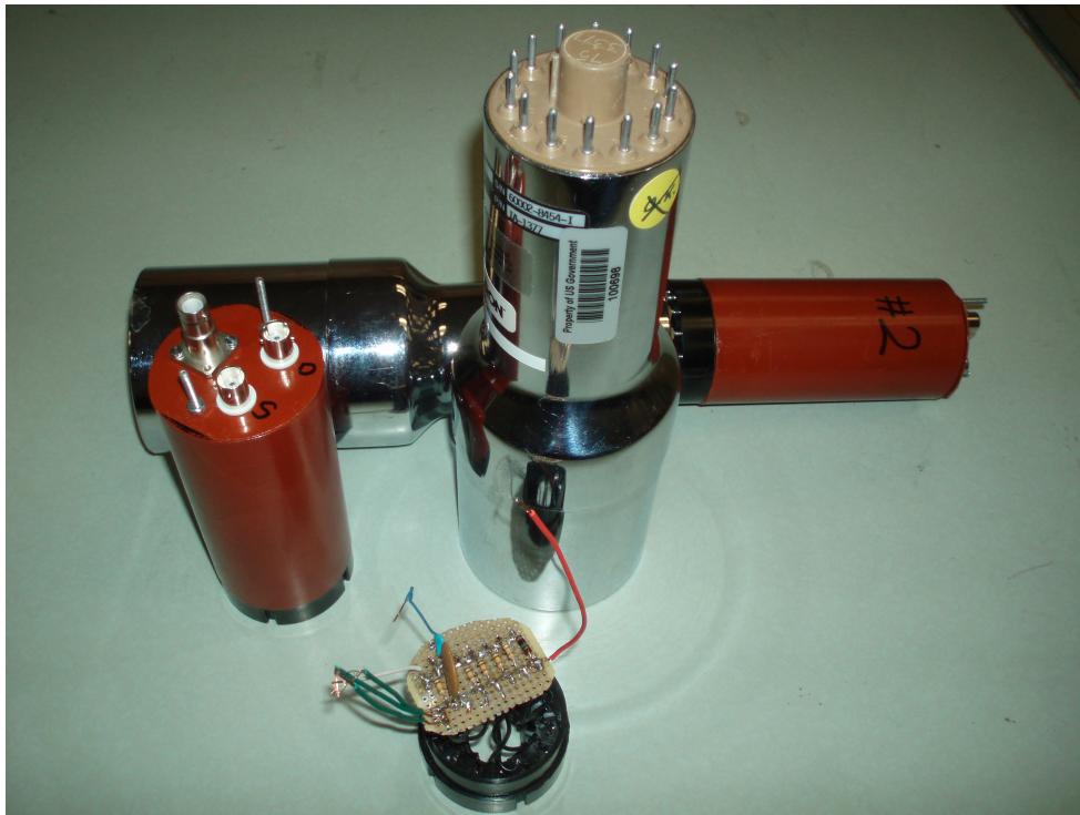
Figure 2.4: Sodium Iodine (NaI) detector and parts.
