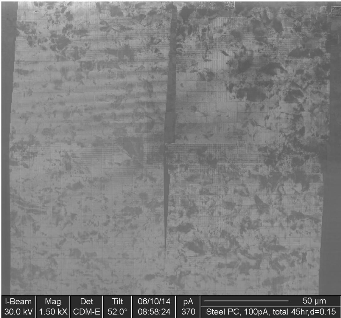
*Figure 37 - A large array of 4 arrays of 225 photonic crystals each milled on steel at 100pA. The data bar has an error – total milling time was closer to 145 hours for this array*
