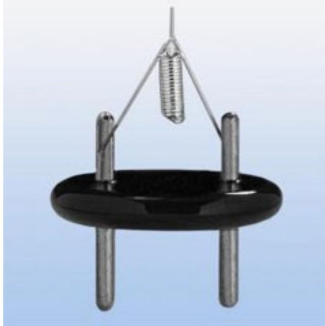
*Figure 9 - An FEI liquid metal ion source (LMIS). There is a large helical wire wrapped around the gallium reservoir for heating with a single wire at the top for the gallium to flow along or through to form the tip. [23]*
