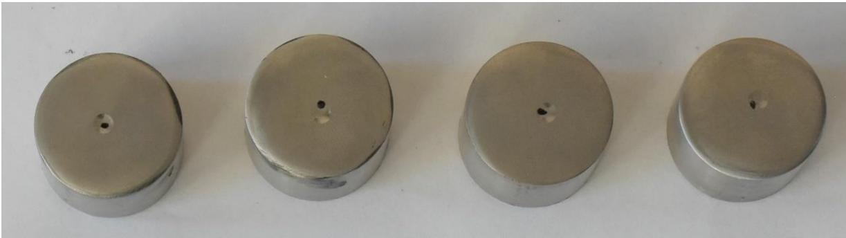
**Figure 4.7 Ti6Al4V Specimens after Brinell Hardness Test**
