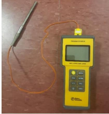
**Figure 5.13 Thermocouple**
