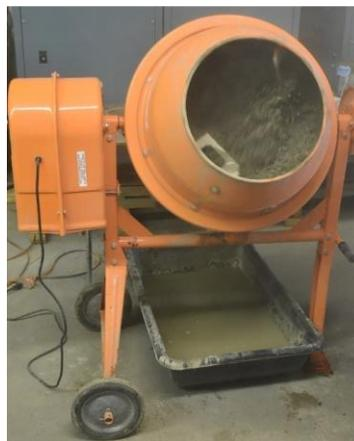
**Figure 7.8 Mixing Concrete**
