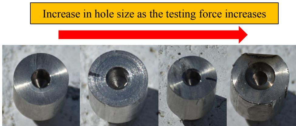
**Figure 6.9 Increase in Alignment Hole Size with Increasing Load**
