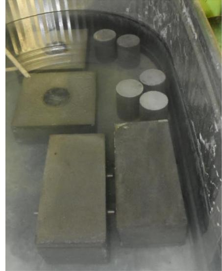
**Figure 7.11 Curing of Concrete Blocks and Cylinders**
