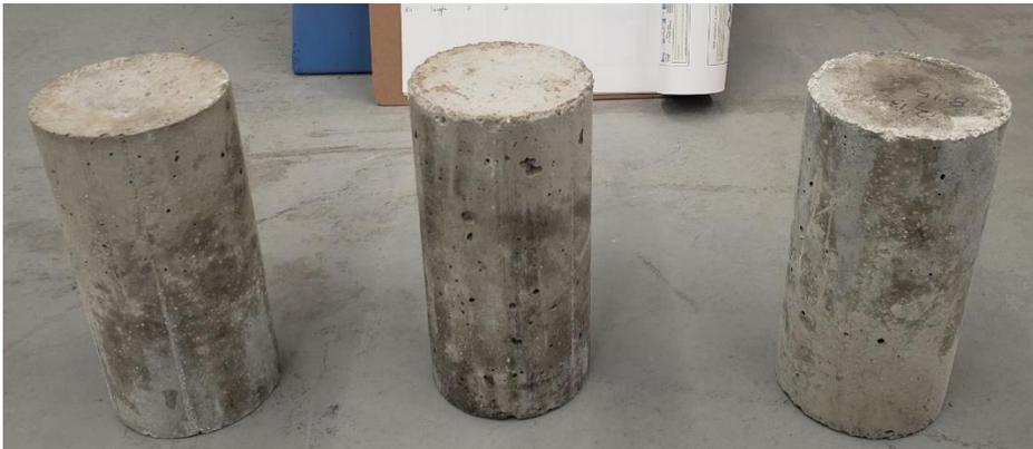
**Figure 7.12 Concrete Specimens for Compressive Test**
