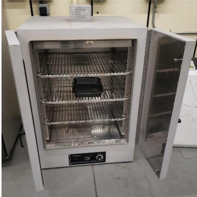
**Figure 5.9 Heating of Charpy Specimen in Lab Oven**
