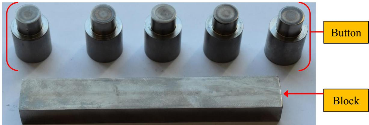
**Figure 6.2 Button and Block Specimens of Ti6Al4V for Galling Test**
