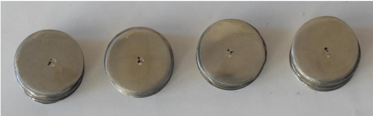
**Figure 4.8 150 ksi Steel Specimens after Brinell Hardness Test**
