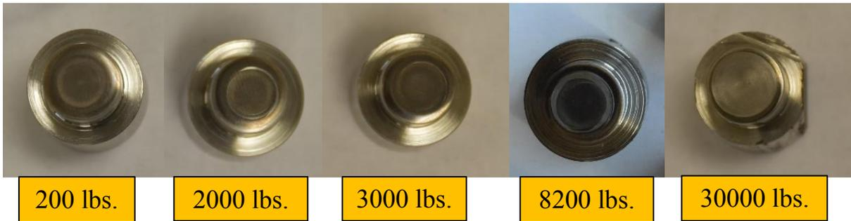
**Figure 6.5 Post Galling Test Ti6Al4V Button Specimens**
