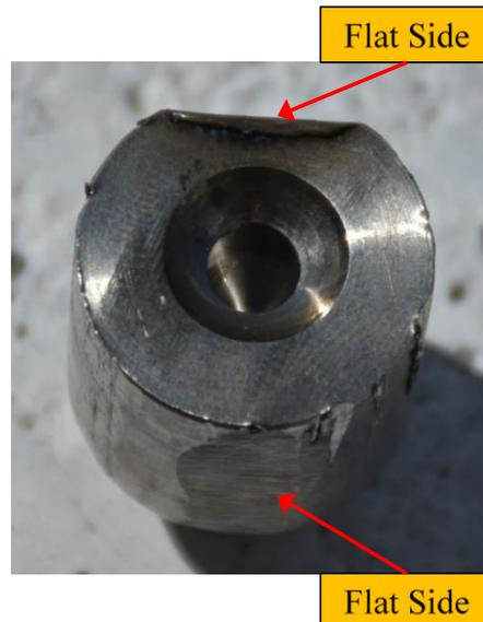
**Figure 6.10 Flattened Button Specimen**
