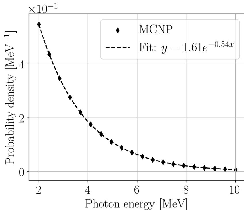
Figure 2.5: MCNP simulation of the energy distribution of the bremsstrahlung photons that reach the fission target. Photons with an energy below 2 MeV are excluded.
