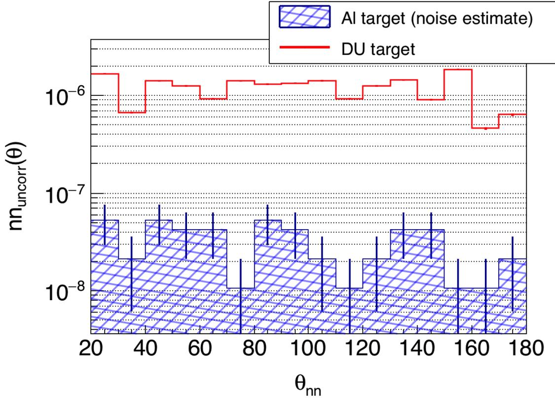
Figure 2.13: An Al target was designed have the same thickness, in radiation lengths, as the  $^{238}\text{U}$  target, thus serving as an equivalent non-neutron producing target well-suited for noise estimates. The rate of the detection of coincident events in the neutron ToF range while using the Al target was 3% that of the  $^{238}\text{U}$  target. Thus, 3% of coincident events used in the determination of n-n angular correlations in  $^{238}\text{U}$  can be attributed to noise.
