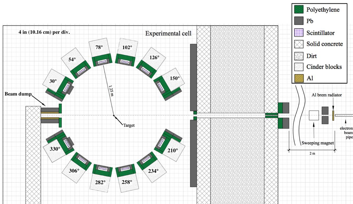
Figure 2.1: To-scale, top down diagram of the experimental setup. An electron beam impinges upon a 3.8 cm thick Al radiator, and the resulting bremsstrahlung beam enters the experimental cell from the top. The supporting structure for each detector has been labeled according to the angle, in degrees, between the center of each detector and direction of the incoming photon beam.
