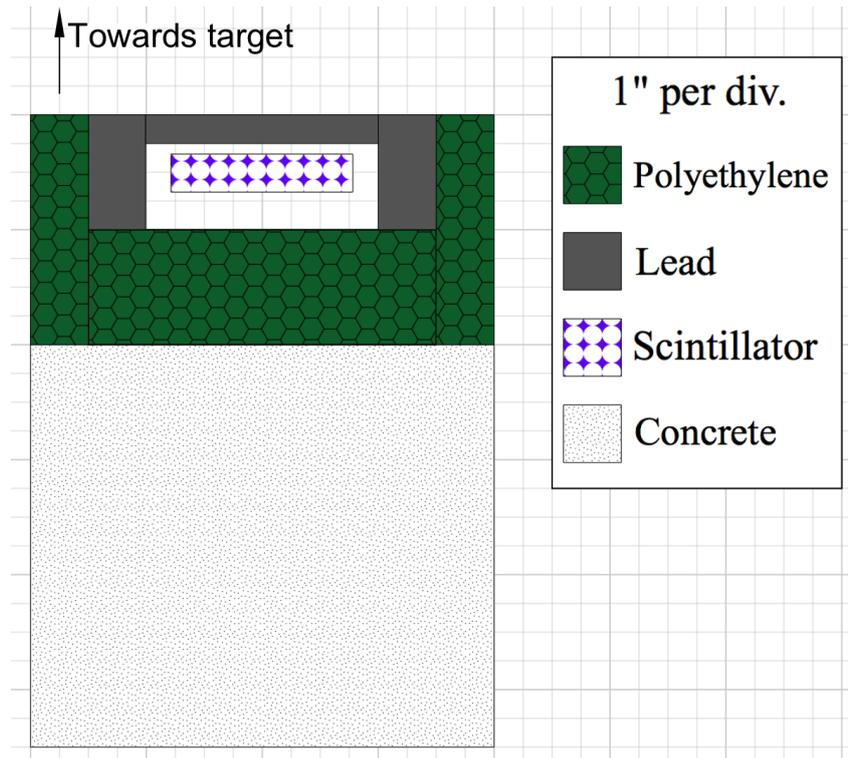
Figure 2.4: Detector shielding was designed to reduce the detection of photons, room return, and detector cross-talk.
