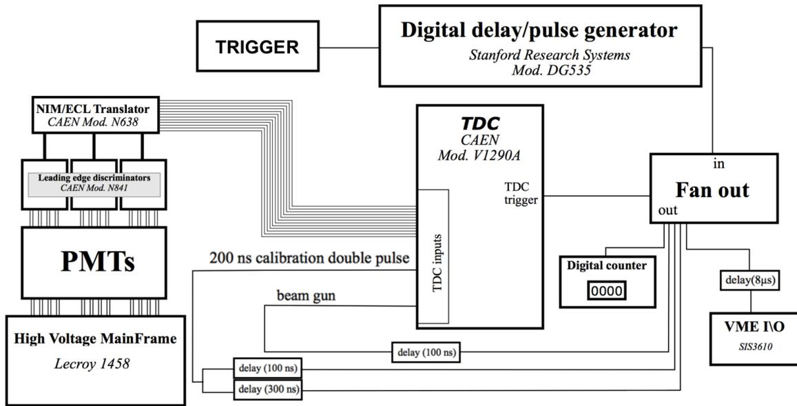
Figure 2.7: Wiring diagram of the electronics setup.
