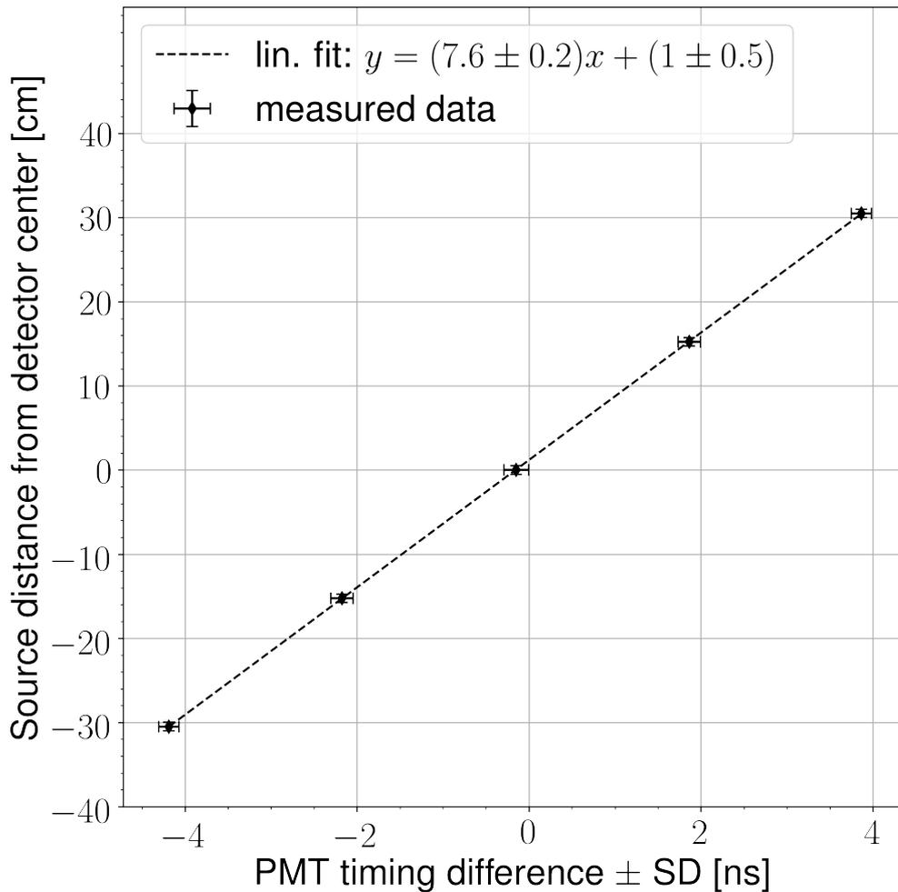
Figure 2.9: A collimated  $^{60}\text{Co}$  source is used to produce photon events at five different positions along the scintillator. The mean PMT timing difference of events at each position varies linearly with respect to the distance of the  $^{60}\text{Co}$  source from the center of the detector. The result of a linear least squares fit to this data is used to calculate the position of detected particles along the length of each scintillator.
