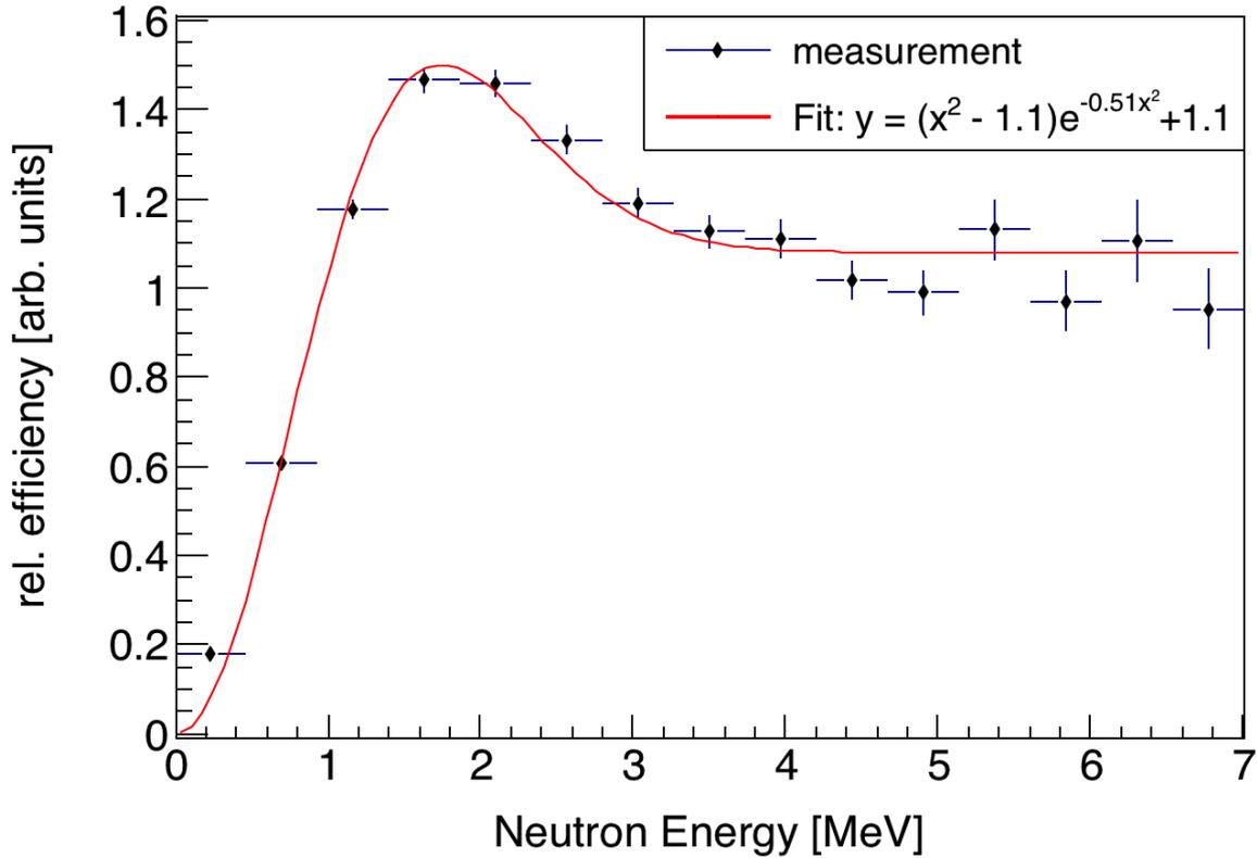
Figure 2.3: The overall relative efficiency of the neutron detection system as a function of neutron energy is calculated by dividing the measured energy distribution by the known energy distribution of neutrons from the SF of  $^{252}\text{Cf}$ . The fit function is empirical.
