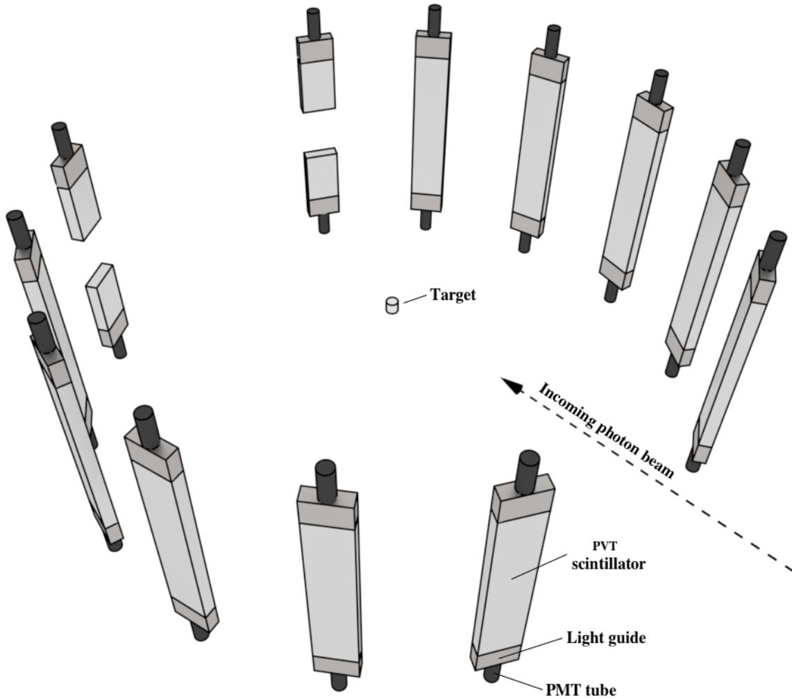
Figure 2.2: 3-D render of the bare, unshielded scintillators, along with PMTs and light guides. Most of the open space between the scintillators was occupied by shielding, as seen in Fig. 2.1.
