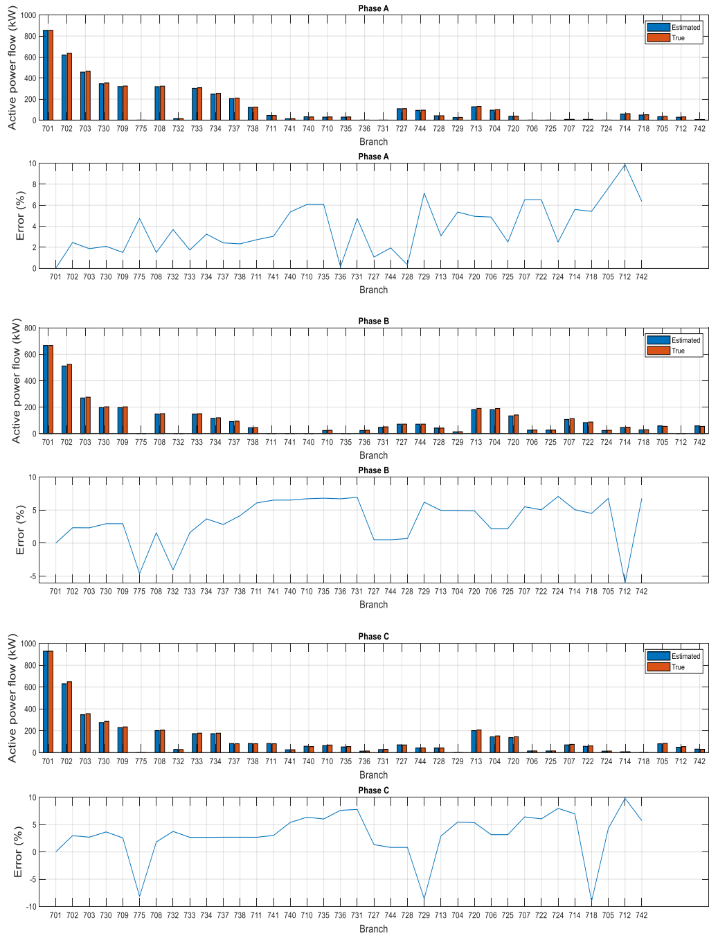
Figure 6. 22: Estimated active power flow (kw) comparison for 37 bus network using LC method
