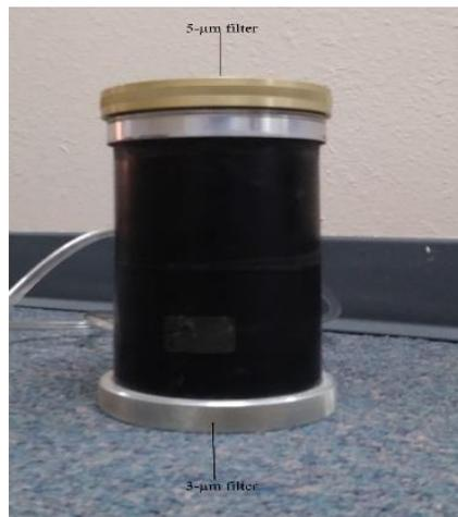
*Figure 15. Series sampling apparatus*
