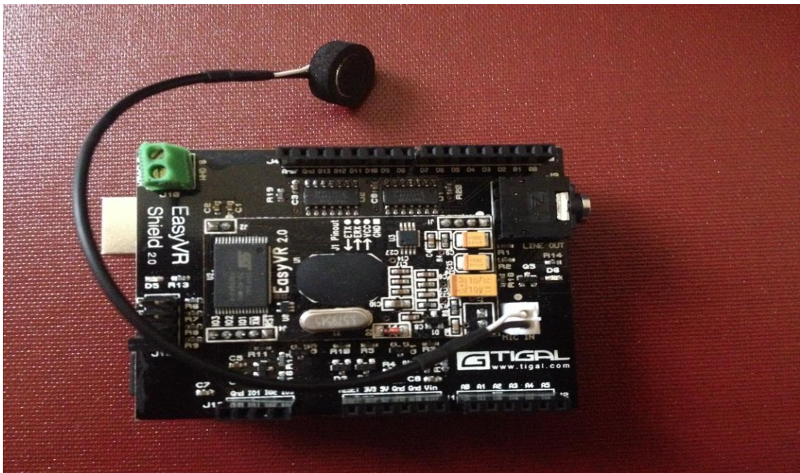
Fig.24 EasyVR shield mounted on top of Arduino™ UNO
