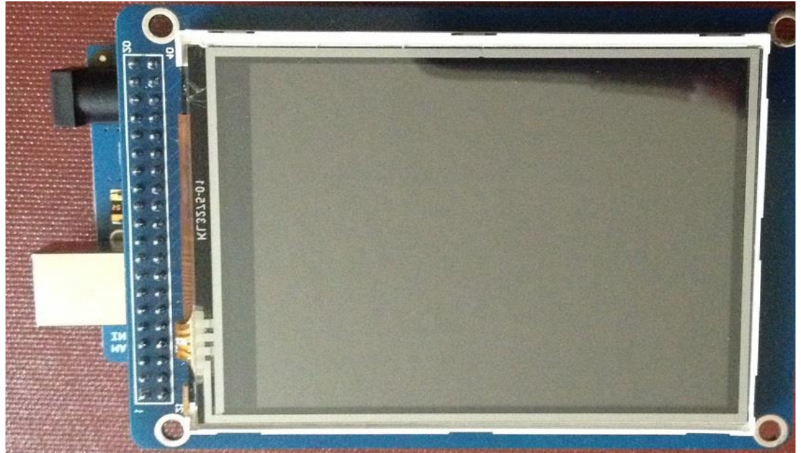
Fig.17 LCD Module top view with 40 pins on left side
